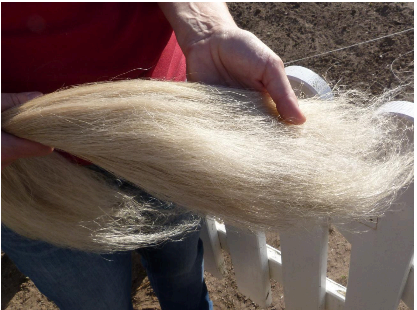
FIG 17. FAILURE. THE FLAX HAD BEEN RETTING FOR TOO LONG. THEREFORE THE LONG FIBRES HAVE DISSOLVED PARTIALLY. PHOTO BY MARTINA KÖNIG.
