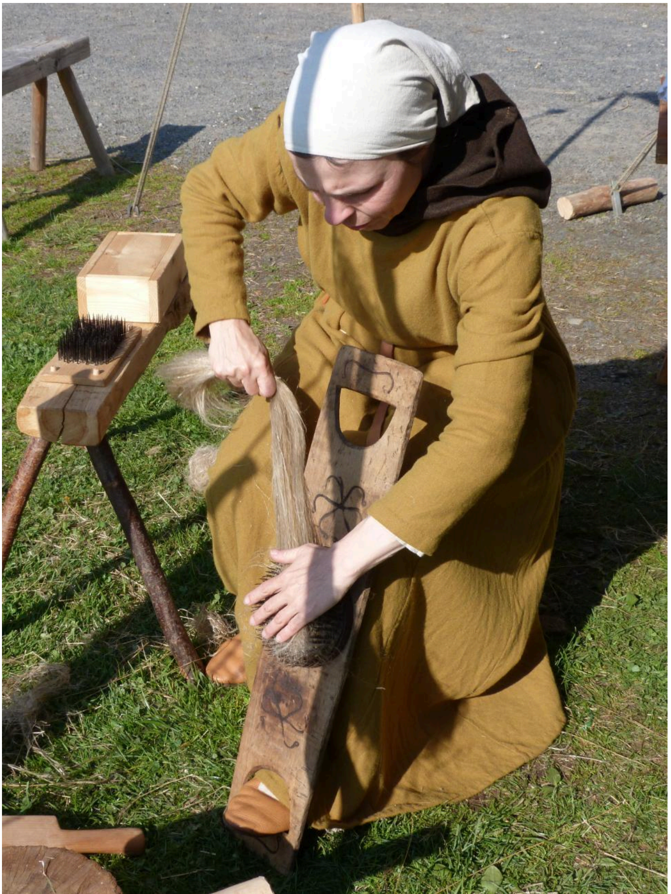
FIG 16. HACKLING THE FLAX FIBRE. PHOTO BY MARTINA KÖNIG.
