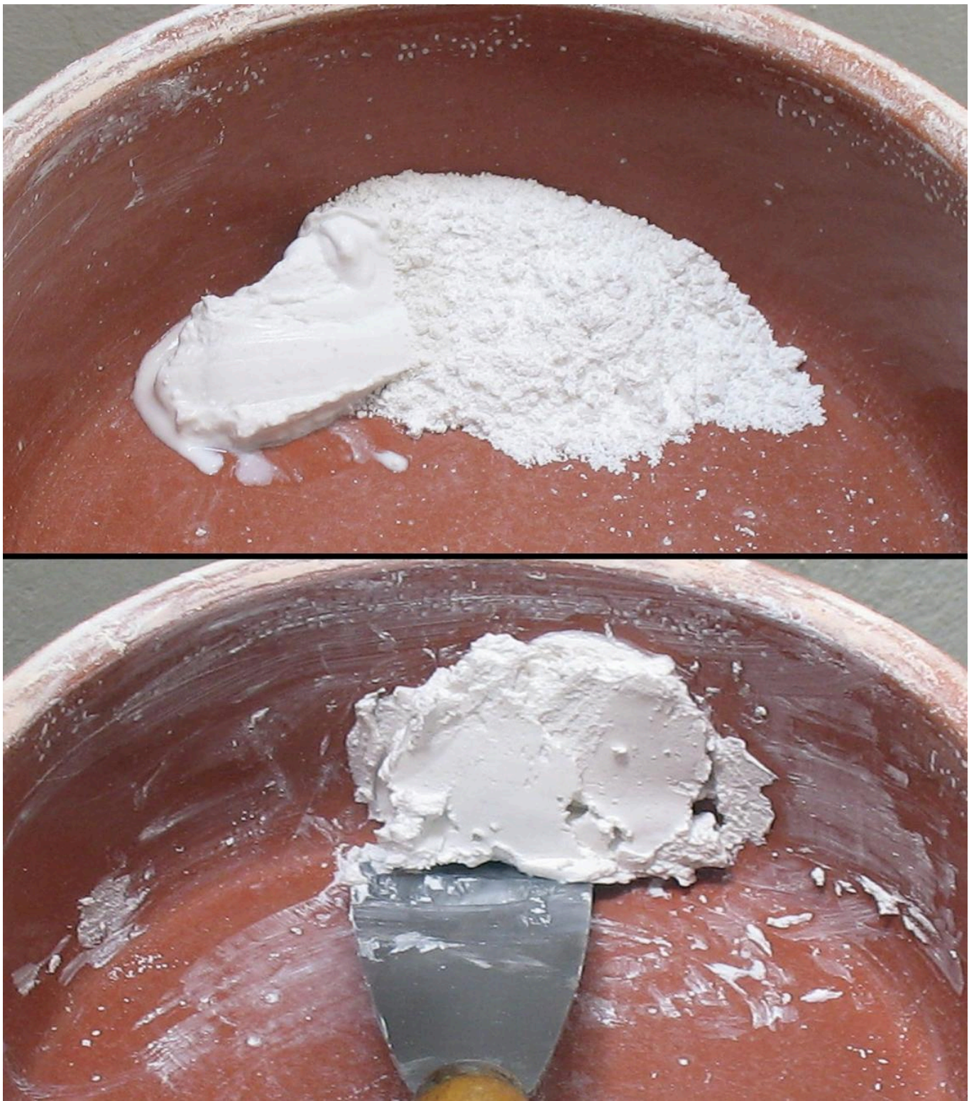
FIG 6. ON THE TOP PICTURE LIME PLASTER AND DRIED POWDERED LIME PLASTER. ON THE BOTTOM PICTURE THE MIXED MORTAR. PHOTO BY ANTONIS VLAVOGILAKIS
