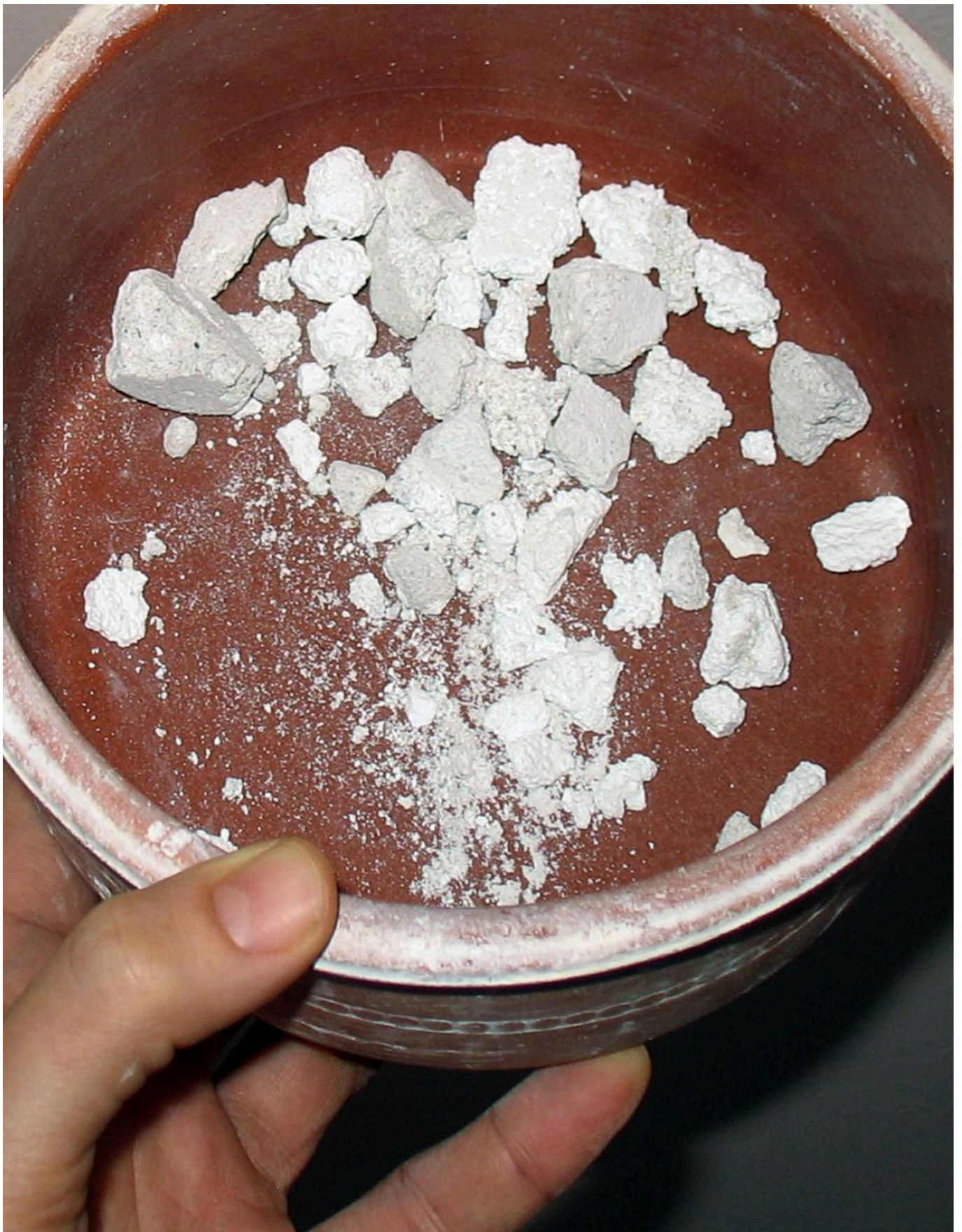
FIG 2. SOME OF THE FRAGMENTS OF MORTARS THAT WERE USED IN THE SAMPLES. PHOTO BY ANTONIS VLAVOGILAKIS
