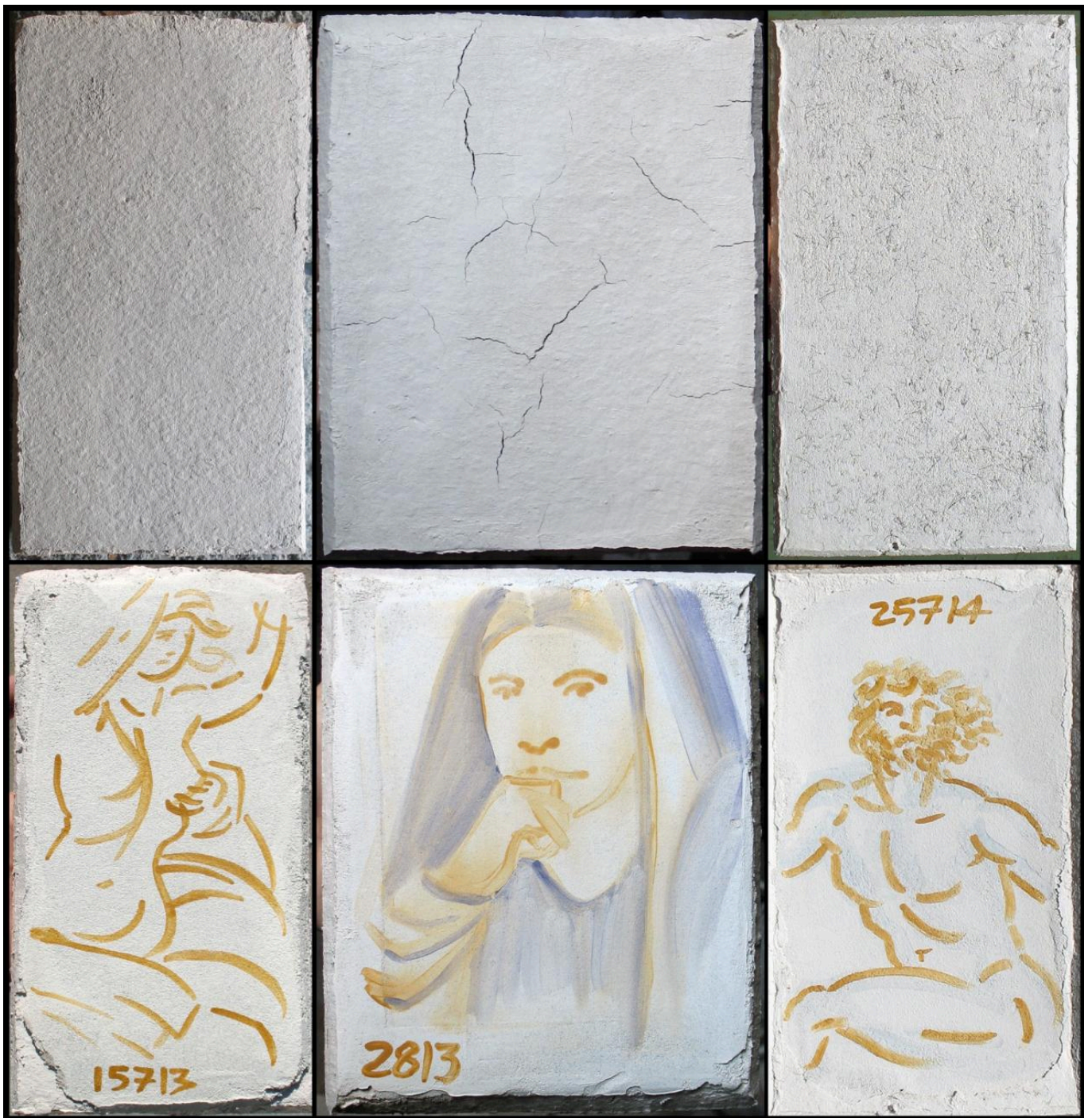
FIG 3. THIS IS A CHARACTERISTIC SELECTION OF SAMPLES FROM THIS SERIES OF EXPERIMENTS. ON THE TOP PICTURES THE DRIED BASE COATS, ON THE BOTTOM PICTURES THE FINAL DRY SAMPLES. IN SAMPLE 15713 ABDUCTION THE BASE MIXTURE DRIED WITHOUT CRACKS. IN SAMPLE 2813 PALMETTE PERSEPHONE THE BASE MIXTURE DEVELOPED CRACKS WHILE DRYING. IN SAMPLE 25714 PLUTO THE MIXTURE ALSO CONTAINED CHOPPED GOAT HAIR, BUT IT STILL DEVELOPED THIN CRACKS. PHOTO BY ANTONIS VLAVOGILAKIS
