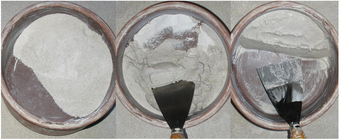
FIG 13. ON THE LEFT CRUSHED SHARDS FROM MORTARS THAT WERE COMPOSED OF LIME AND THIN SAND. IN THE MIDDLE THE ADDITION OF WATER. ON THE RIGHT THE FINAL MIXTURE. PHOTO BY ANTONIS VLAVOGILAKIS
