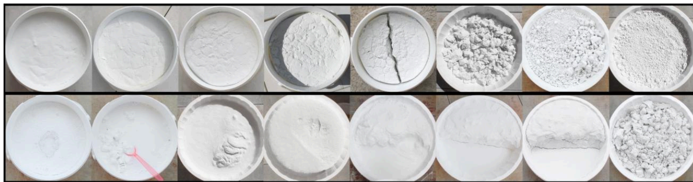
FIG 1. DRYING LIME PLASTER: FIRST ROW FROM LEFT TO RIGHT THE DRYING OF LIME. ON THE SECOND ROW WATER IS ADDED TO THE DRIED POWDERED LIME PLASTER AND AFTER STIRRING IT IS LEFT TO DRY AGAIN. PHOTO BY ANTONIS VLAVOGILAKIS
