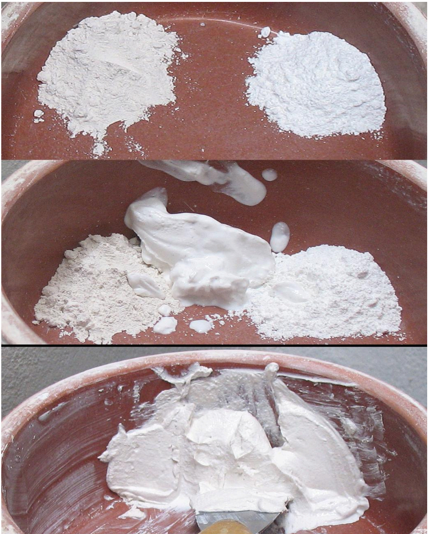
FIG 8. ON THE TOP PICTURE, ON THE RIGHT DRIED POWDERED LIME PLASTER, ON THE LEFT POWDERED CHALK. IN THE PICTURE IN THE MIDDLE THE ADDITION OF LIME PLASTER. ON THE BOTTOM PICTURE THE FINAL MIXTURE. PHOTO BY ANTONIS VLAVOGILAKIS
