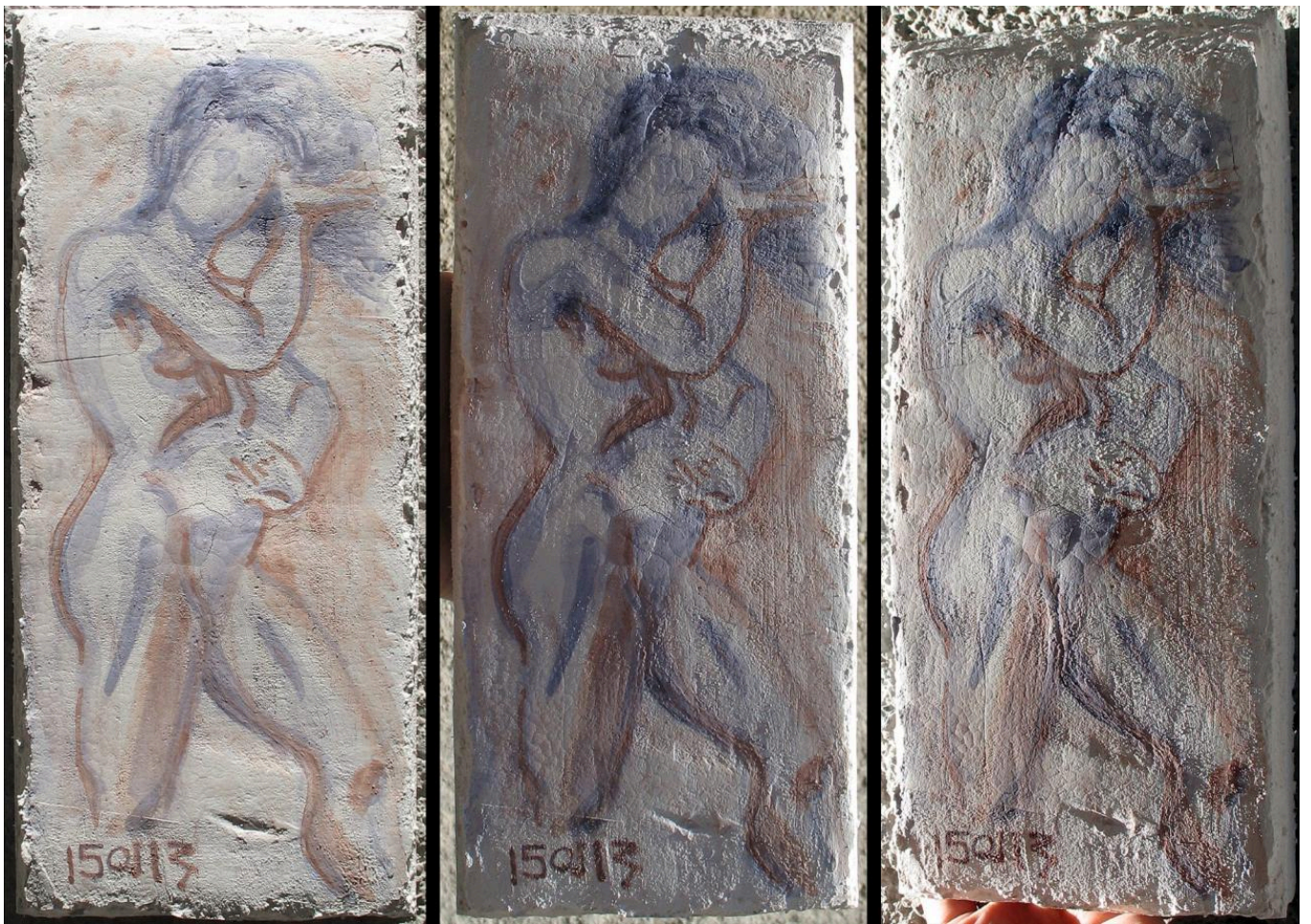
FIG 5. . SAMPLE 150113 FEMALE FIGURE: THREE PHOTOGRAPHS OF THE DRY SAMPLE TAKEN WITH LIGHT AT DIFFERENT ANGLES TO SHOW THE SURFACE TEXTURE AND EXTEND OF THE CRACKING. PHOTO BY ANTONIS VLAVOGILAKIS
