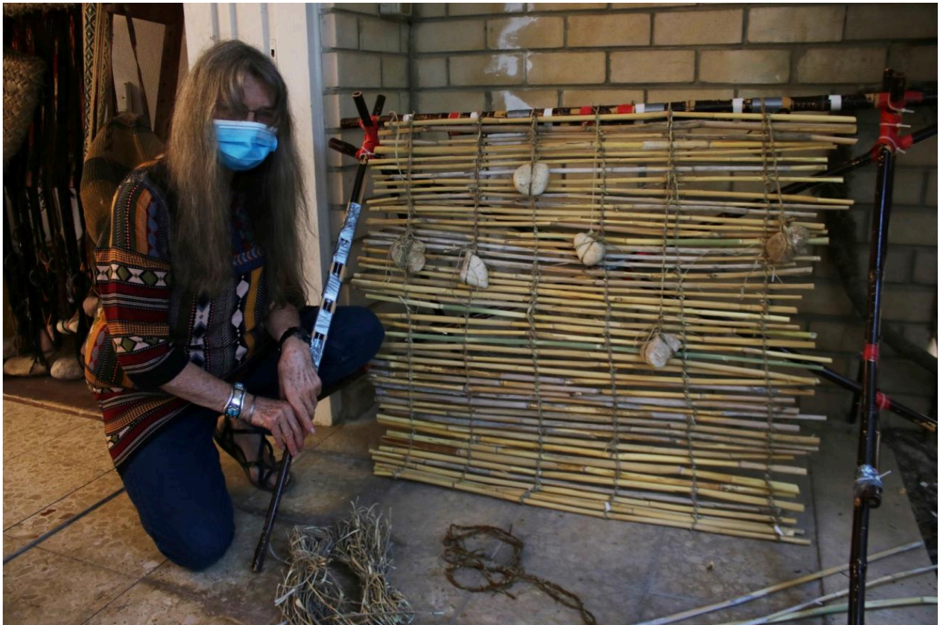
FIG 5. RECONSTRUCTION OF LOOM FOR WARP TWINED MATS. PHOTO BY DAVIDA EISENBERG-DEGEN.
