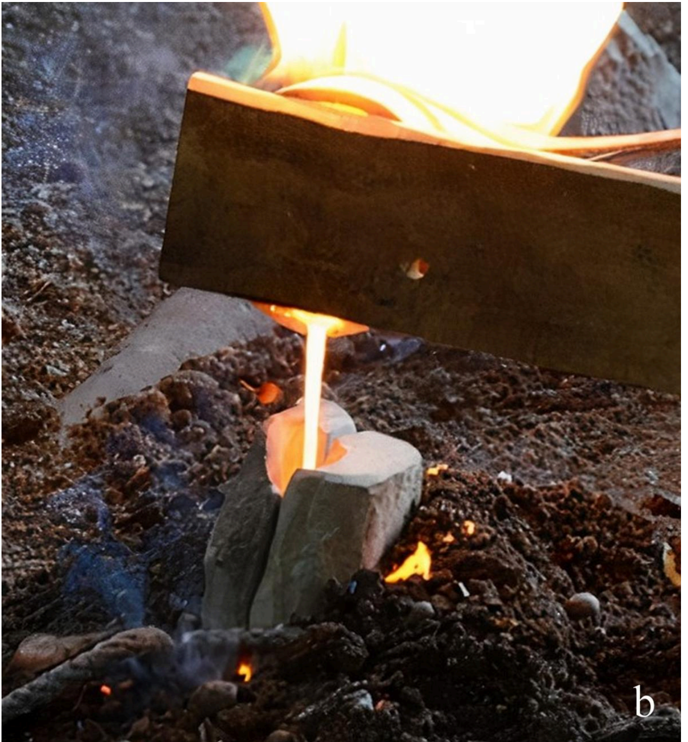
FIG 4B. EXPERIMENTAL REPRODUCTION OF THE BRONZE FLANGED AXE: BRONZE CASTING. PHOTO BY ALESSIO PELLEGRINI.
