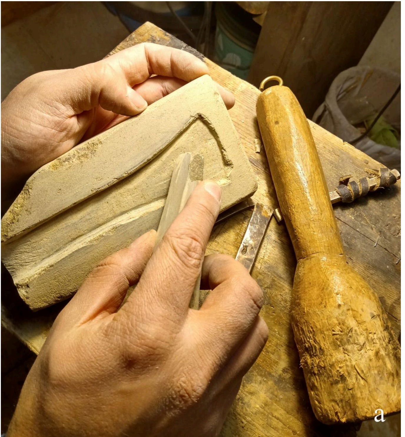
FIG 4A. EXPERIMENTAL REPRODUCTION OF THE BRONZE FLANGED AXE: SANDSTONE MOULD CARVING. PHOTO BY ALESSIO PELLEGRINI.
