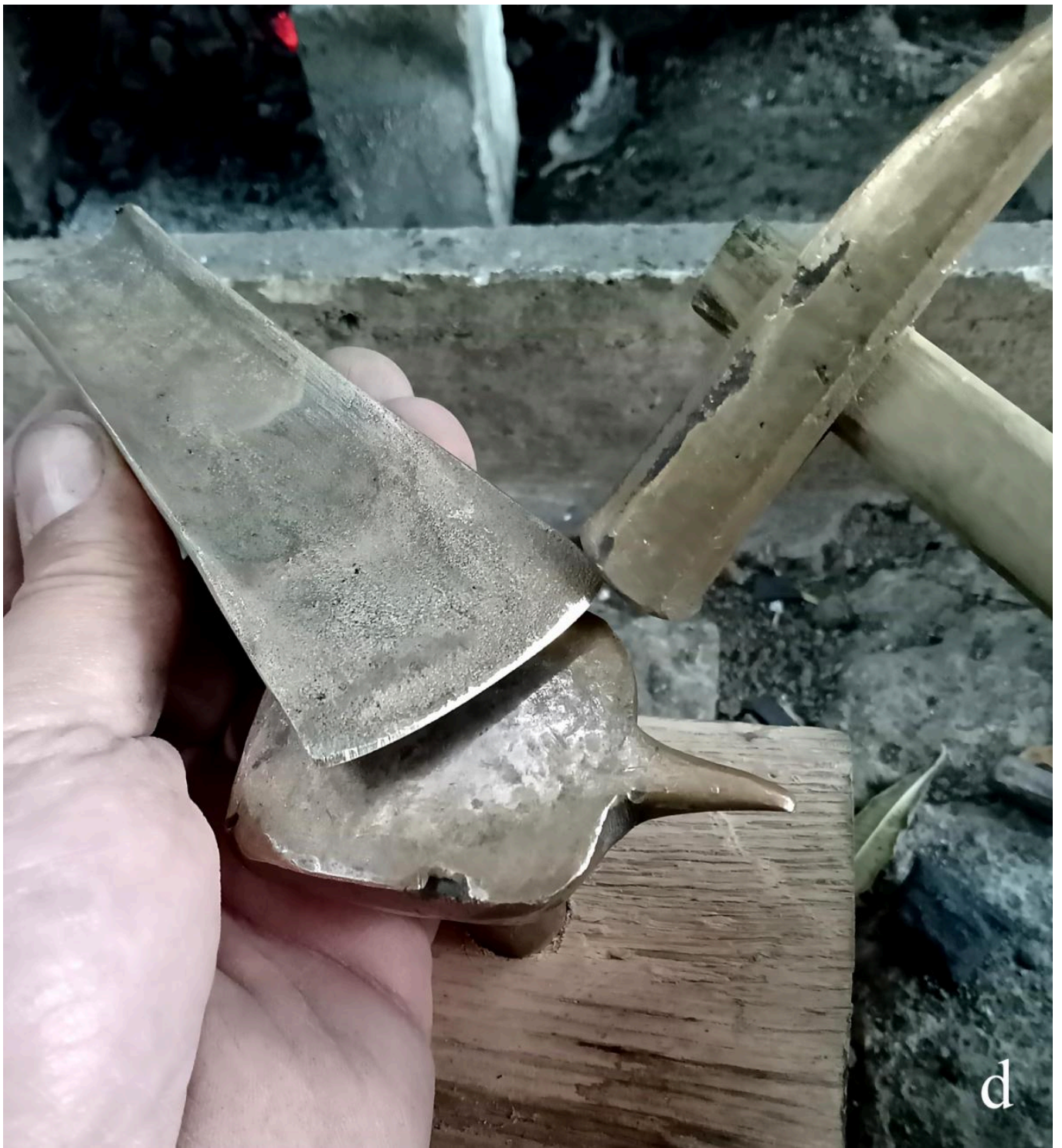
FIG 4D. EXPERIMENTAL REPRODUCTION OF THE BRONZE FLANGED AXE: BEVEL HAMMERING. PHOTO BY ALESSIO PELLEGRINI.
