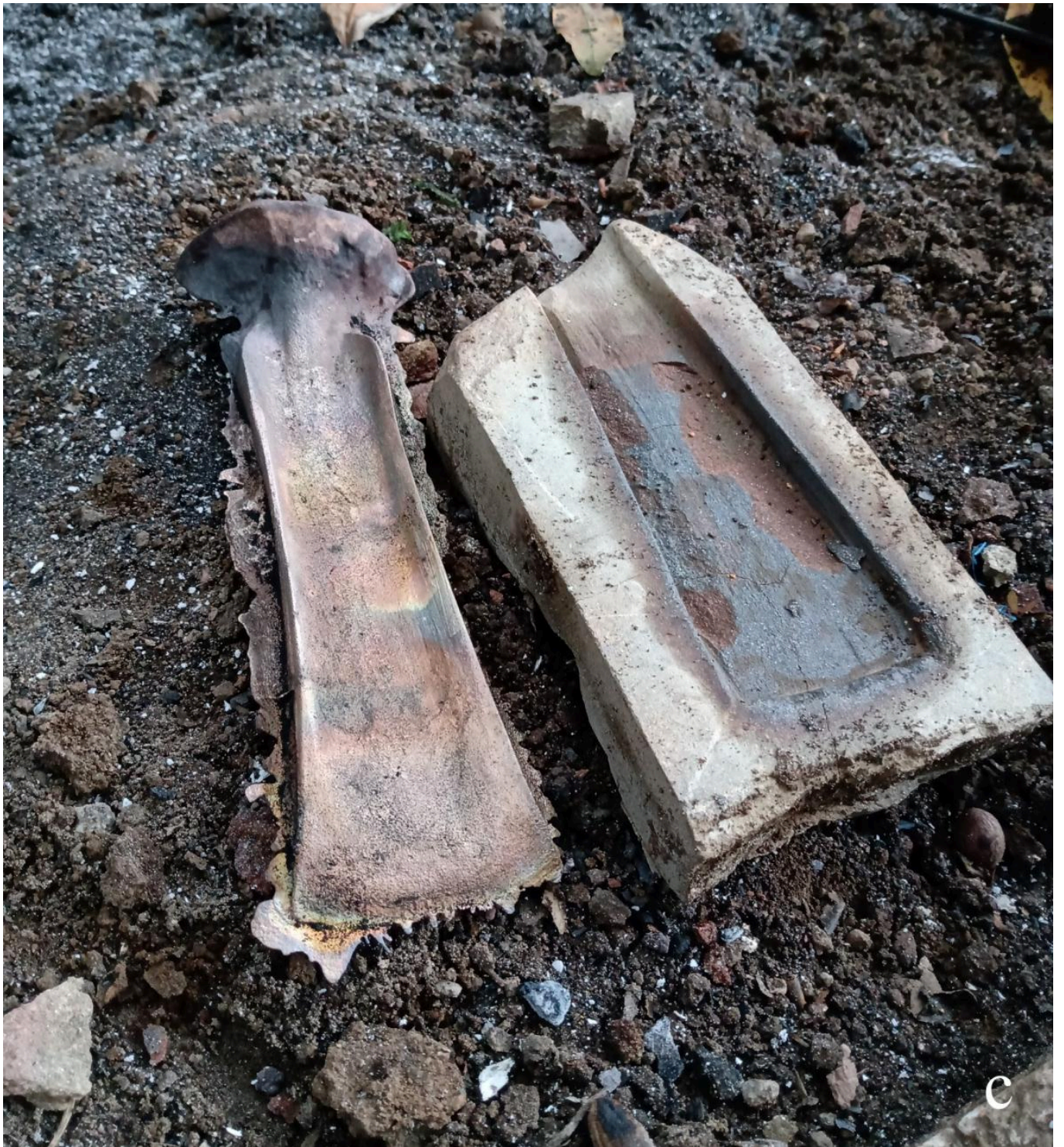
FIG 4C. EXPERIMENTAL REPRODUCTION OF THE BRONZE FLANGED AXE: POST CASTING. PHOTO BY ALESSIO PELLEGRINI.
