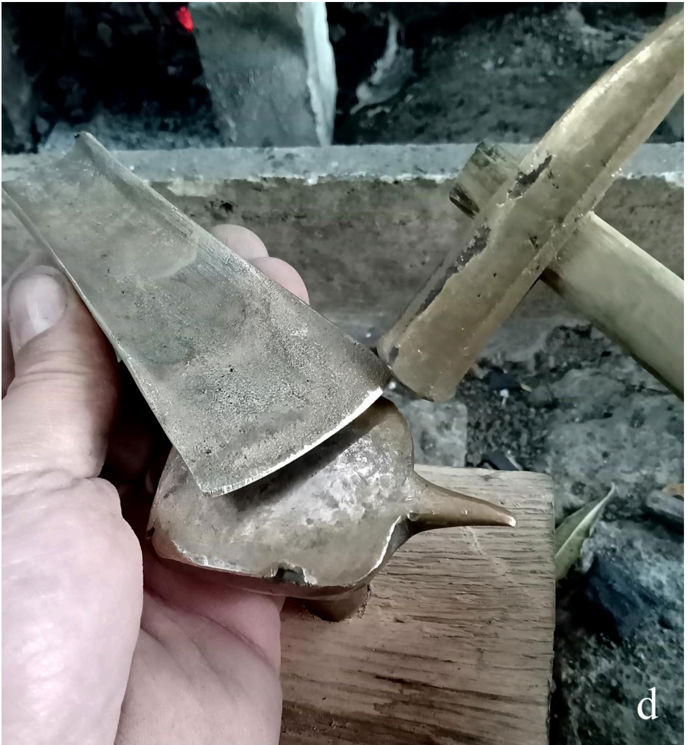
FIG 4D. EXPERIMENTAL REPRODUCTION OF THE BRONZE FLANGED AXE: BEVEL HAMMERING. PHOTO BY ALESSIO PELLEGRINI.
