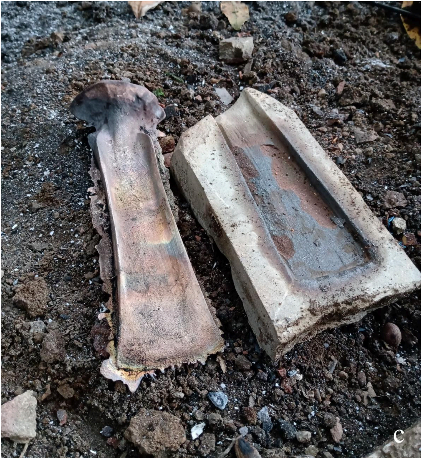
FIG 4C. EXPERIMENTAL REPRODUCTION OF THE BRONZE FLANGED AXE: POST CASTING. PHOTO BY ALESSIO PELLEGRINI.
