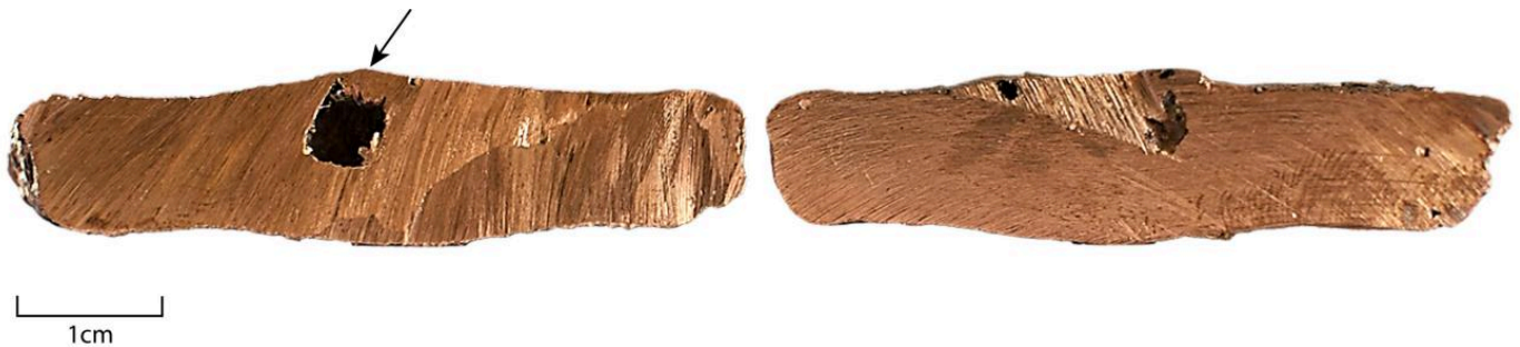
FIG 10. TRAPPED GAS BUBBLE WITHIN THE CORE OF EA11 WITHIN THE MAIN SWELL (SEE FIGURE 7 IN BLUE). THE ARROW SHOWS THE LOCATION AND ANGLE OF THE EXHAUST VACUOLE. PHOTO BY AURÉLIEN BURLLOT
