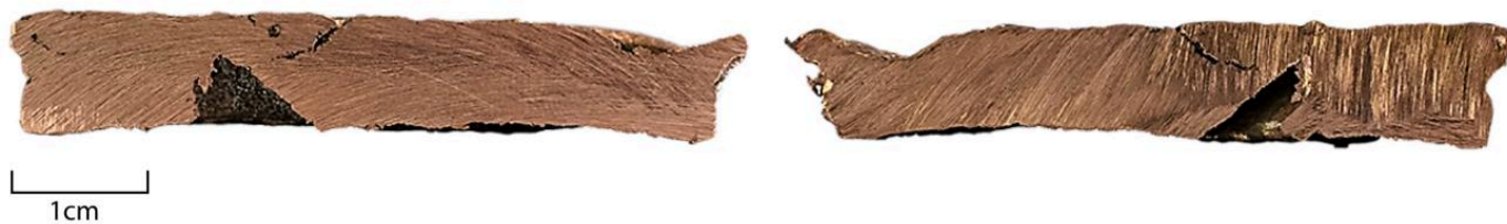
FIG 12. DEFECTS WITHIN THE CORE OF EAI2 INCLUDING THE SMALL DEPRESSION LOCATED BELOW THE CENTRAL DIP WHICH HAD A HOLE IN IT (SEE FIGURE 8 IN RED AND YELLOW), AS WELL AS A SMALL BUT NOTICEABLE CRACK RUNNING TOWARDS THE TOP SURFACE. PHOTO BY AURÉLIEN BURLOT
