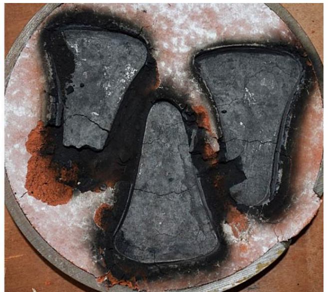
FIG 4. SURFACE OF THE SAND MOULDS AFTER CASTING. HOMEMADE GREEN SAND WITH A CRUMBLY SURFACE BUT NO BURNT MARKS (LEFT) AND SCORCHED AND FLAKY SURFACES IN DELFT CLAY (RIGHT). PHOTO BY AURÉLIEN BURLOT
