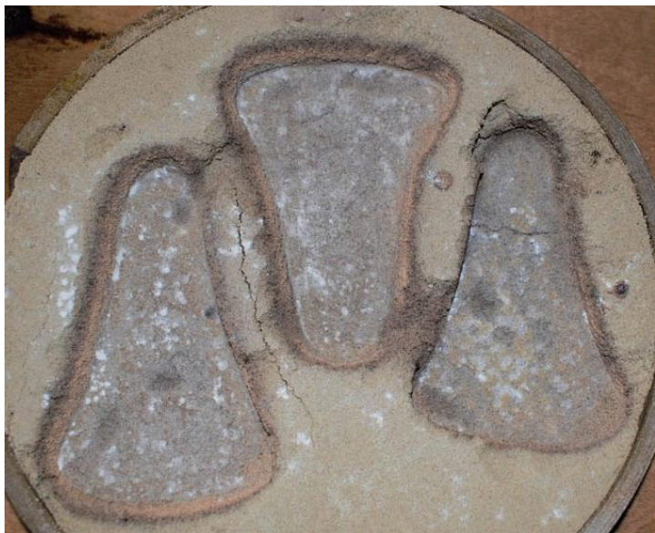
FIG 4. SURFACE OF THE SAND MOULDS AFTER CASTING. HOMEMADE GREEN SAND WITH A CRUMBLY SURFACE BUT NO BURNT MARKS (LEFT) AND SCORCHED AND FLAKY SURFACES IN DELFT CLAY (RIGHT). PHOTO BY AURÉLIEN BURLOT
