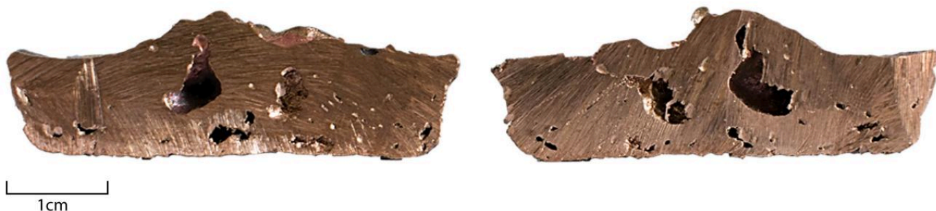
FIG 13. TRAPPED GAS BUBBLES WITHIN THE CORE OF EAI3 INCLUDING TWO CENTRALLY LOCATED AND SOME SMALLER ONES ON THE EDGES, NOTABLY NEAR THE BASE. PHOTO BY AURÉLIEN BURLOT
