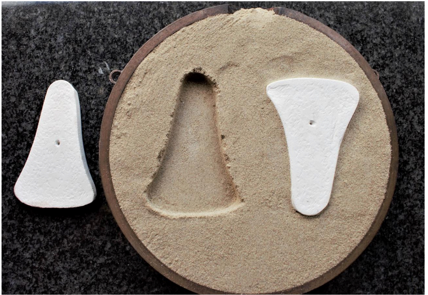
FIG 6. THE DOUBLE MOULDS MADE FOR EACH EXPERIMENT. THE SAND WAS COMPACTED WITHIN A METAL RING AND THE CLAY TEMPLATES PRESSED DOWN TO MAKE THE IMPRINTS. THE TEMPLATES WERE REMOVED USING A SCREW INSERTED WITHIN THE HOLE ON THE TOP. NOTE THE CRUMBLING TOP EDGE WITHIN THE LEFT IMPRINT. THIS CONTRIBUTED TO SOME OVERFLOWING WHEN THE COPPER WAS PUSHED UPWARDS AS IT REACTED WITH THE WET SAND AS SEEN ON THE FIRST EXPERIMENT (SEE FIGURE 7). PHOTO BY AURÉLIEN BURLOT
