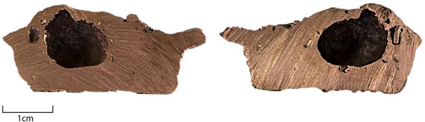
FIG 11. LARGE TRAPPED GAS BUBBLE WITHIN THE CORE OF EA11 WITHIN THE SWELL TOWARDS THE BUTT (SEE FIGURE 7 IN BLUE). PHOTO BY AURÉLIEN BURLLOT
