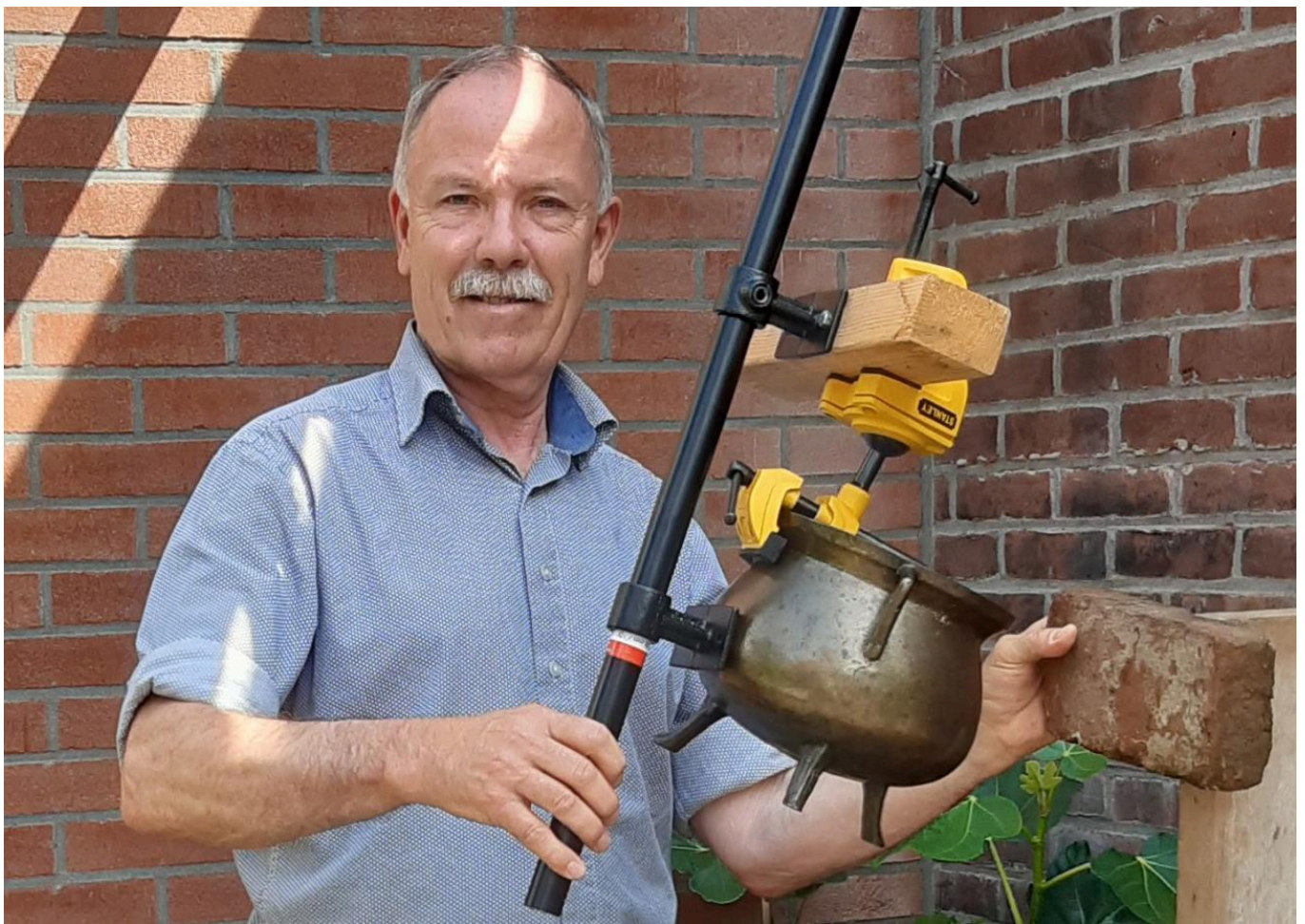
FIG 7. IN ORDER TO BE ABLE TO MANEUVER THE CAULDRON FREELY IN ANY POSITION IN THE EXPERIMENT, THE VESSEL WAS FASTENED BY A MULTI-AXIS VISE ATTACHED TO THE PENDULUM. PHOTO BY J.R. BEUKER.
