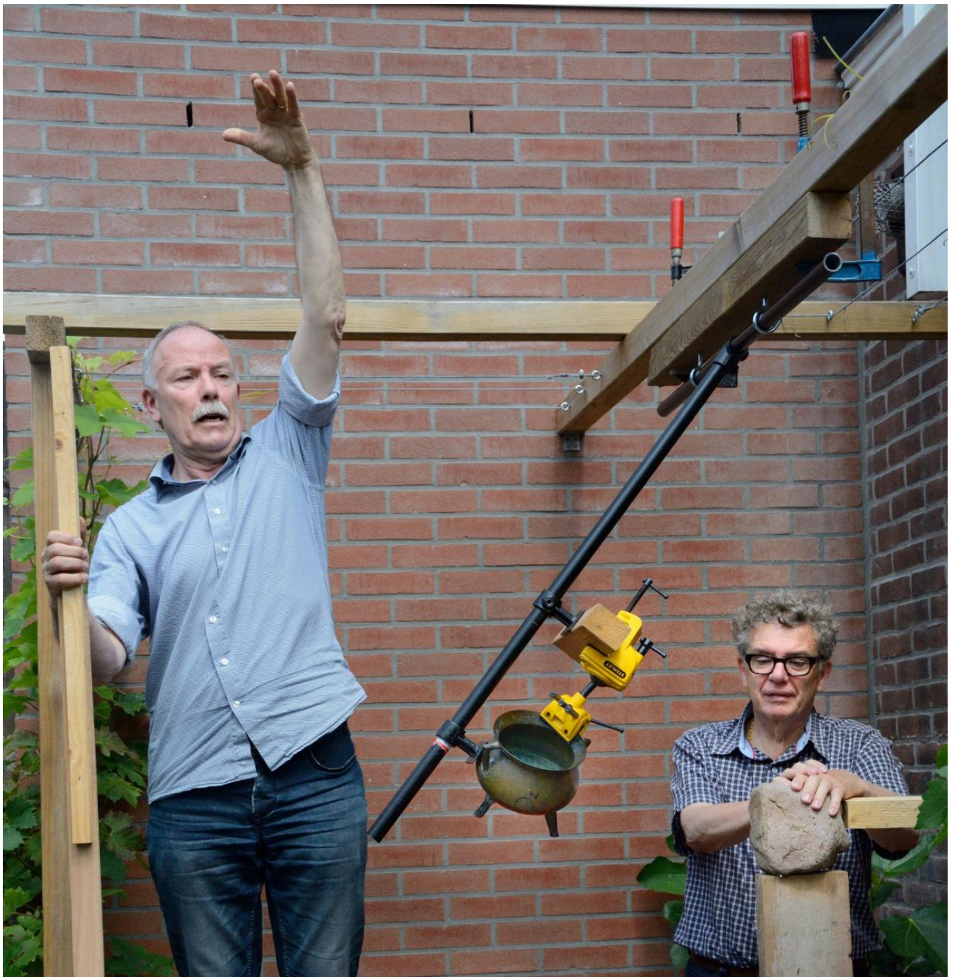
FIG 5. THE CONSTRUCTION OF THE PENDULUM USED FOR THE EXPERIMENT. IN THIS CASE THE CAULDRON IS CLOSE TO A COLLISION WITH A BOULDER OF QUARTZITE SANDSTONE. PHOTO BY J.R. BEUKER.
