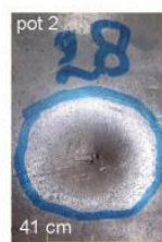
FIG 8. EXPERIMENTAL MUTILATION OF THE TWO BRONZE CAULDRONS: RESULTS OF THE ATTEMPTS WITH WOOD, BRICK, BOULDER, AND AXE. NOTE THAT THE CRACK AT NR. 5 IS NOT THE RESULT OF THE ATTEMPT WITH THE BOULDER, BUT OF A LATER ATTEMPT TO BREAK OFF THE NEARBY LEG. PHOTO BY V.T. VAN VILSTEREN.
