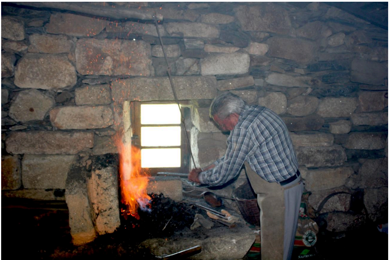
FIG 16. MR. MAMEDE GARCÍA IN HIS TRADITIONAL FORGE (PENTES, OURENSE). SMELTING CASSITERITE AND CASTING A TIN INGOT IN AN TURNIP MOULD, APRIL 2013. COPYRIGHT: BEATRIZ COMENDADOR
