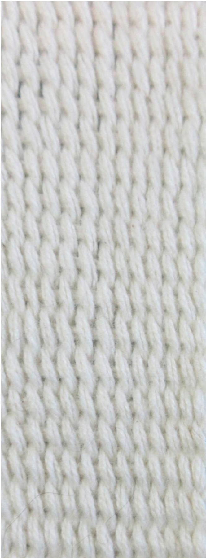
FIG 3. TIGHTLY PACKED, WARP-FACED WARP-TWINED FABRIC AS PRODUCED IN THIS EXPERIMENT. PHOTO BY BILLIE J. A. FOLLENSBEE
