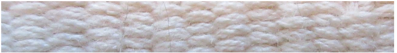
FIG 2. LOOM-WOVEN, WEFT-FACED 2/2 TABBY WEAVE PRODUCED USING THE LUNATE ARTIFACTS USING 1.5 MM COTTON YARN CORDAGE (FOLLENSBEE 2020). PHOTO BY BILLIE J. A. FOLLENSBEE
