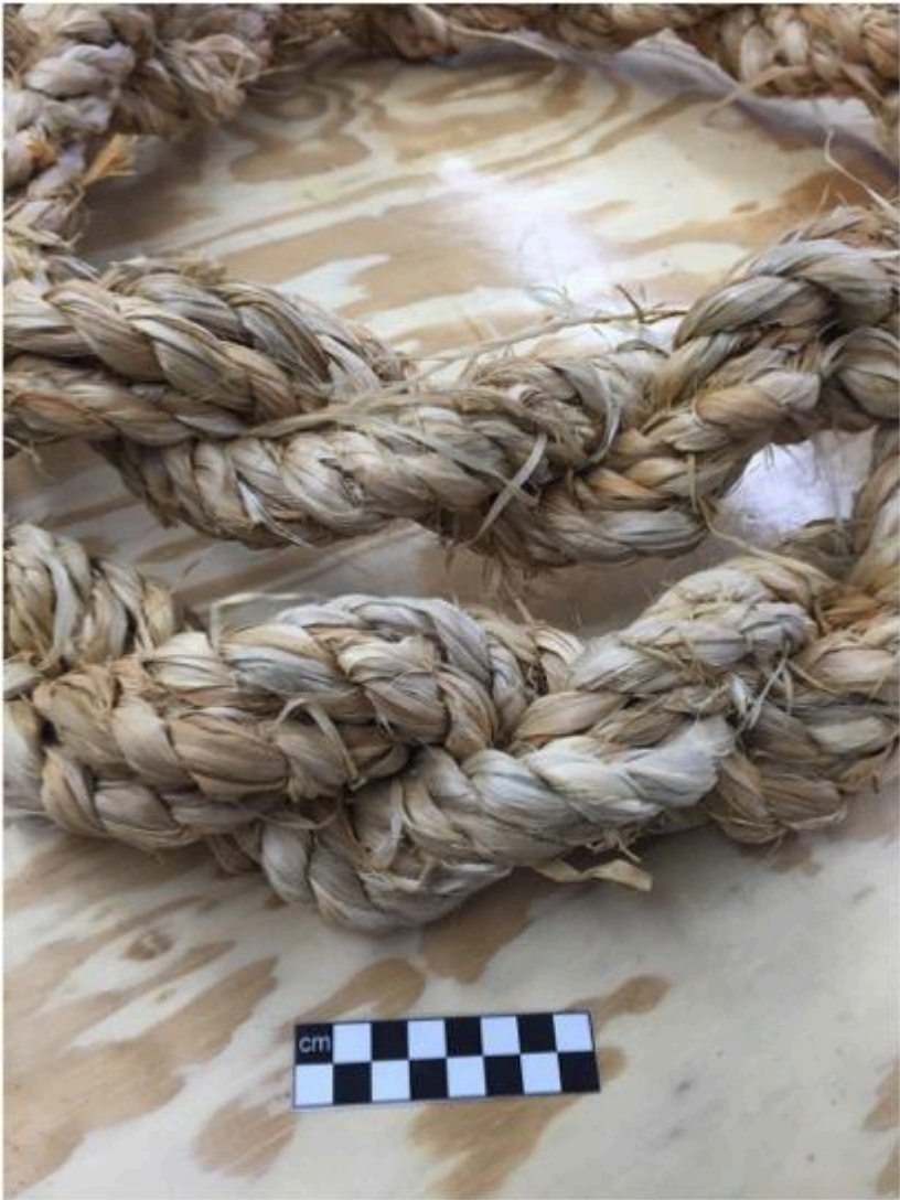
FIG 8. THE COMPLETED COMPOSITE ROPE WITH SCALE.
