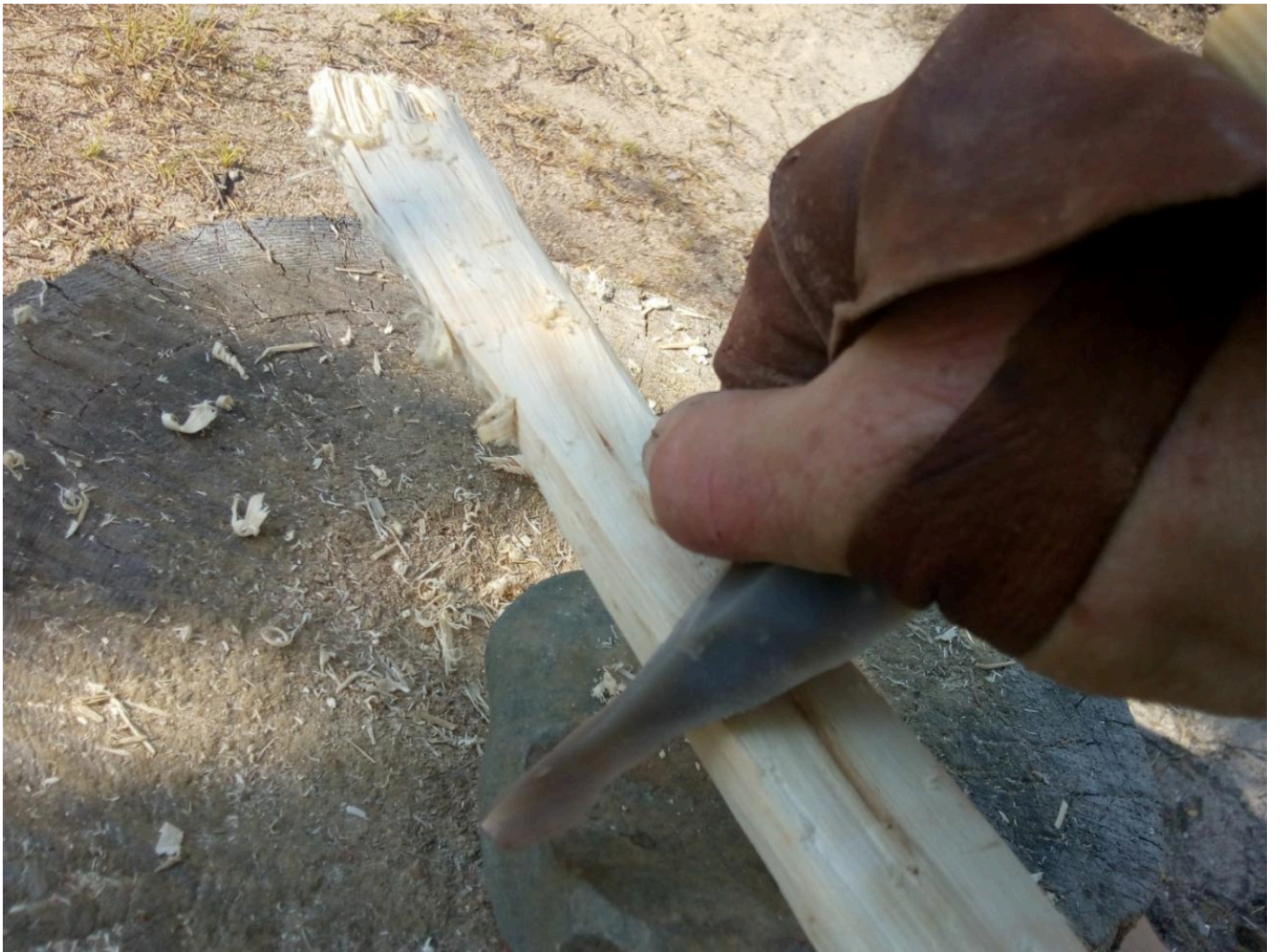
FIG 16. THE IMPROVISED HAND GUARD AND WORKING THE BOW TIPS. PHOTO BY CHRIS WOODLAND
