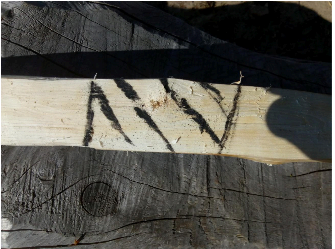
FIG 15. MARKING AREAS OF THE BOWSTAVE FOR REMOVAL OF MATERIAL WITH CHARCOAL. PHOTO BY CHRIS WOODLAND
