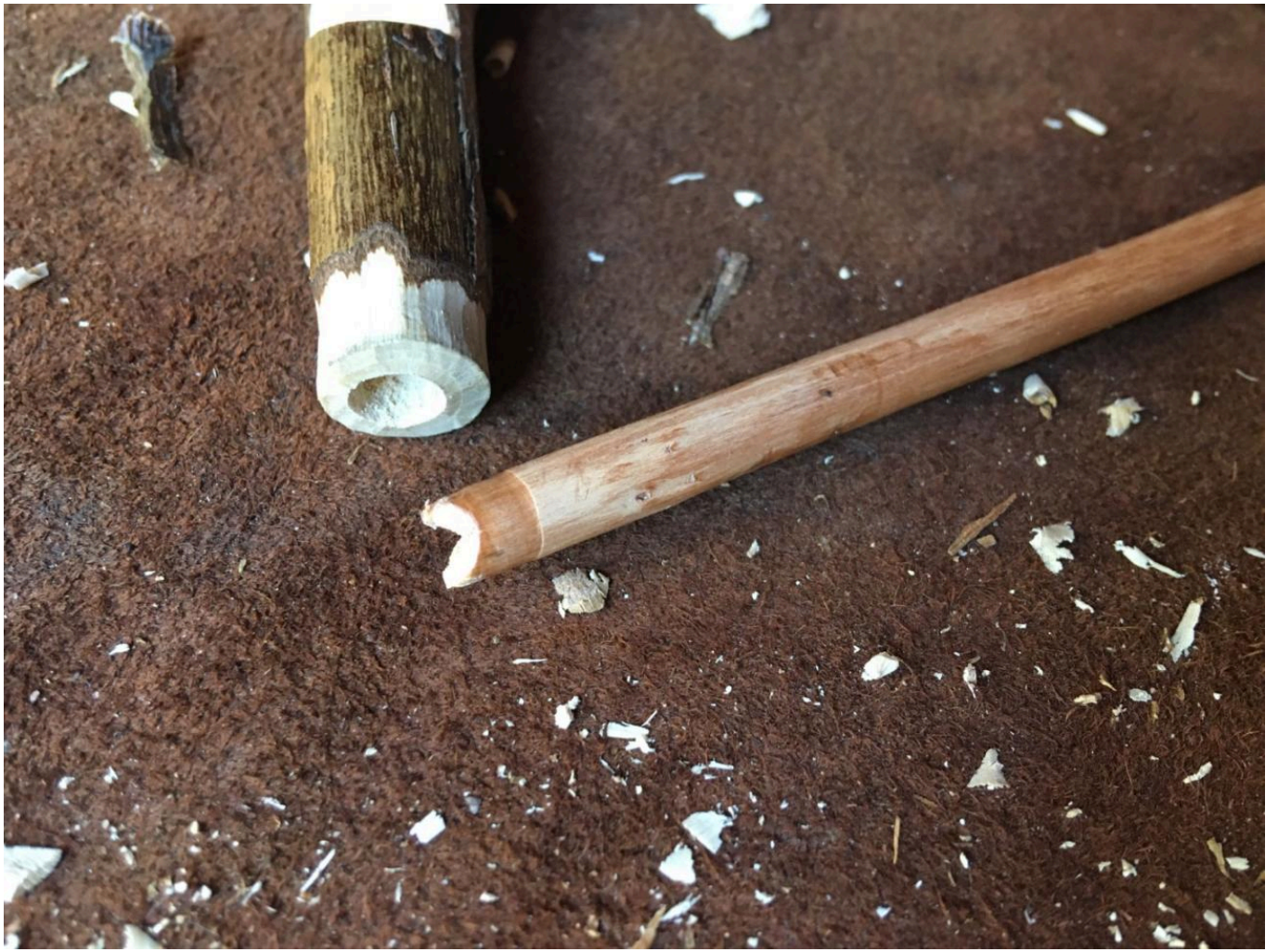
FIG 8. PITH REMOVED USING WILLOW TOOL. PHOTO BY SIMON WYATT
