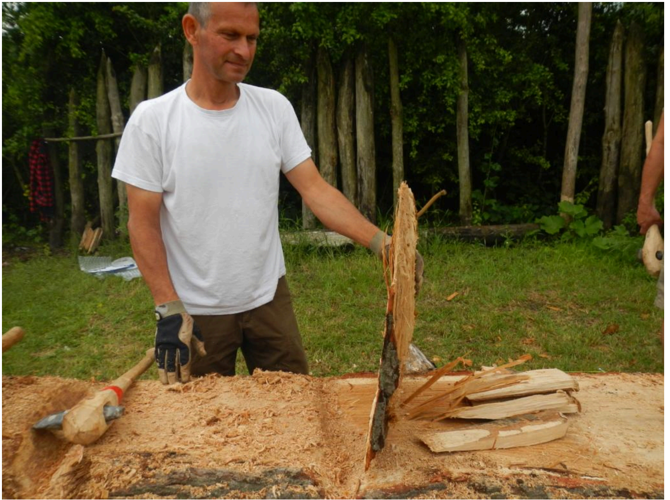
FIG 3. MAKING WEDGES STEP 3: REMOVING THE SLICE SPLIT WOOD FROM THE TRUNK.
