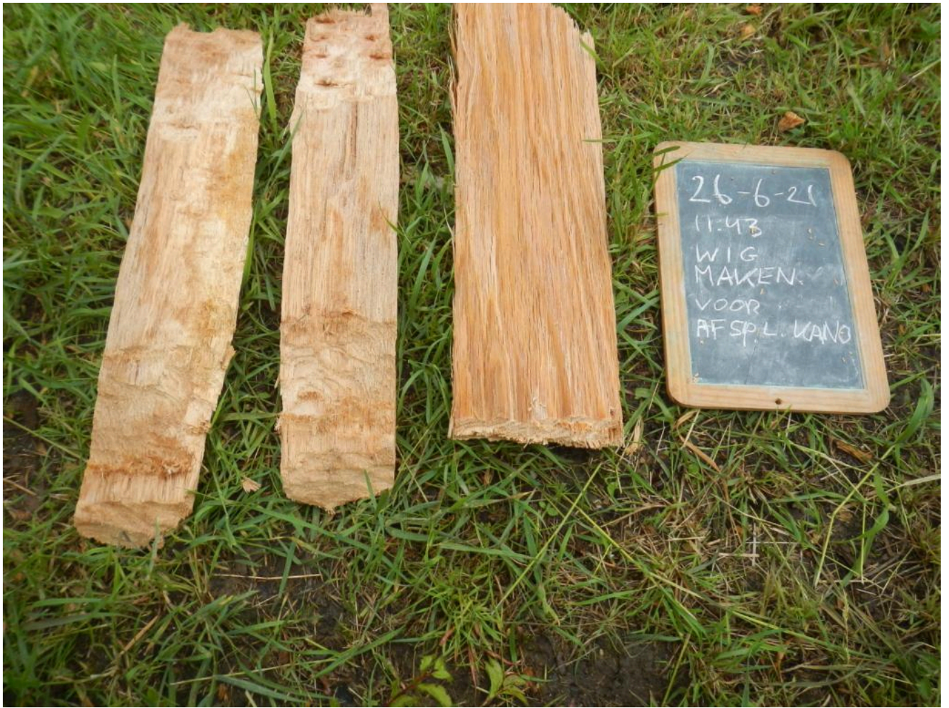
FIG 5. THE SLICE OF WOOD REMOVED WITH THE WEDGES MADE OF PREVIOUS SLICES.
