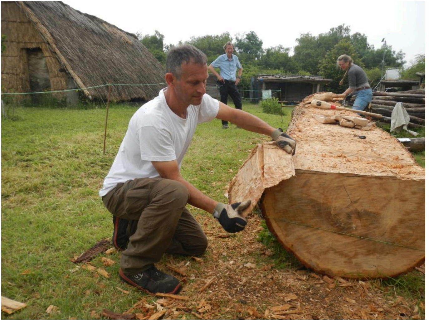
FIG 4. MAKING WEDGES STEP 4: SPLITTING THE SLICE OF WOOD INTO THREE WEDGES.
