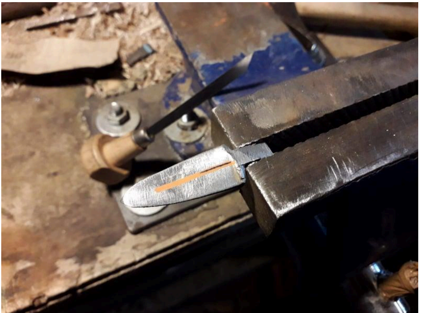
FIG 1. CARVING THE GROOVE ON THE LEFT SIDE. PHOTO BY MAURO FIORENTINI
