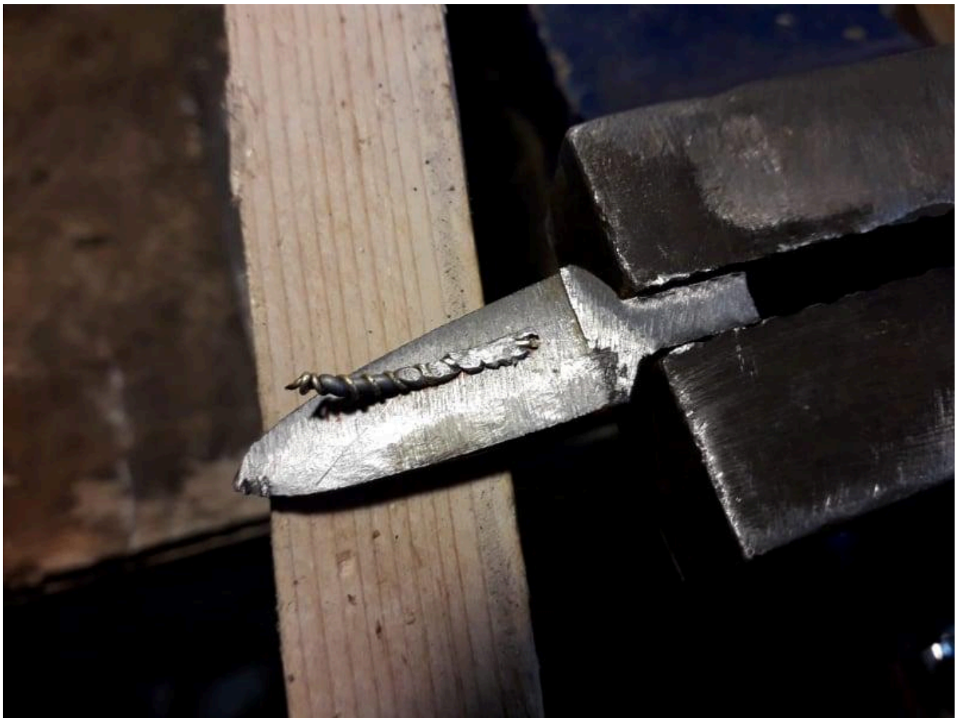
FIG 5. THE SECOND COUPLE OF TWISTED WIRES IS BEING HAMMERED ON THE BLADE'S RIGHT SIDE. PHOTO BY MAURO FIORENTINI
