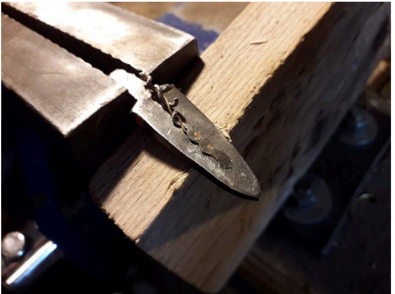
FIG 4. EARLY PHASES OF HAMMERING THE TWISTED WIRES ON THE LEFT SIDE GROOVE. PHOTO BY MAURO FIORENTINI
