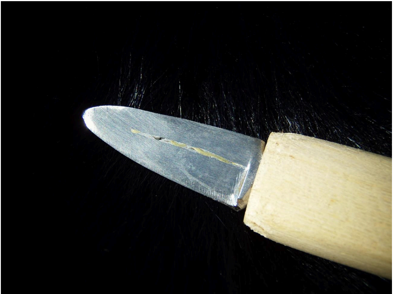
FIG 8E. ZOOMING ON THE LEFT SIDE OF THE BLADE, WHERE THE INLAY IS CLEARLY VISIBLE. PHOTO BY MAURO FIORENTINI
