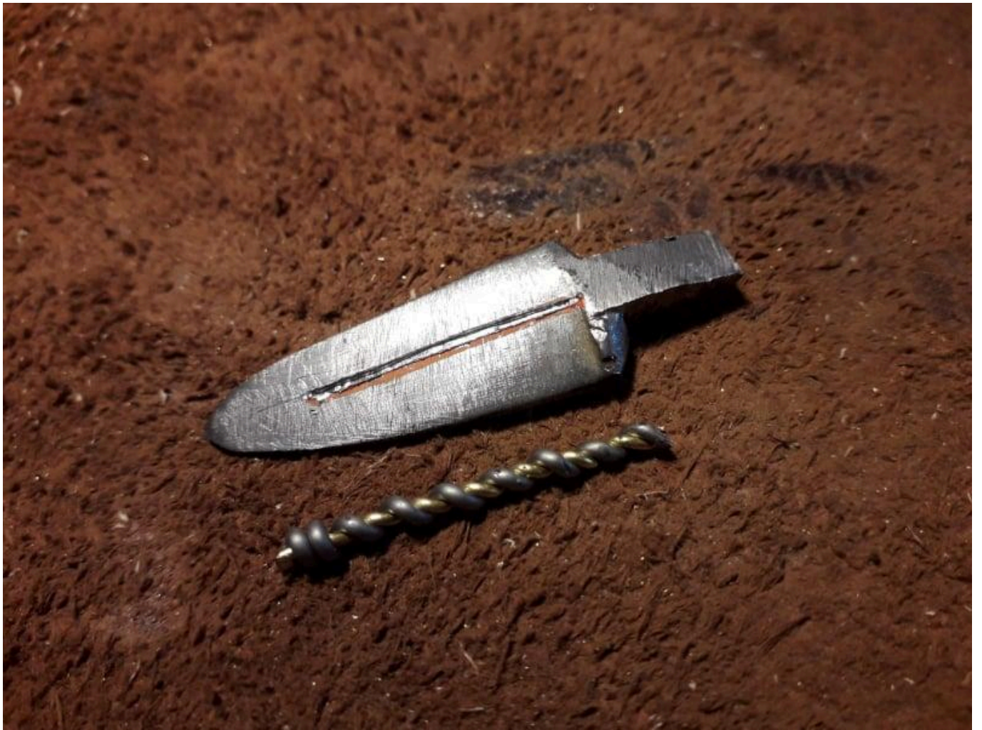
FIG 2. THE GROOVE IS CARVED AND THE SOFTER METAL WIRES TWISTED. PHOTO BY MAURO FIORENTINI
