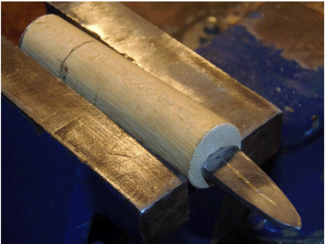
FIG 6. GROOVES HAVE BEEN FILLED WITH THE TWISTED WIRES, THE BLADE SURFACE HAS BEEN SMOOTHED AND IS NOT TIME TO WORK ON THE HANDLE. PHOTO BY MAURO FIORENTINI
