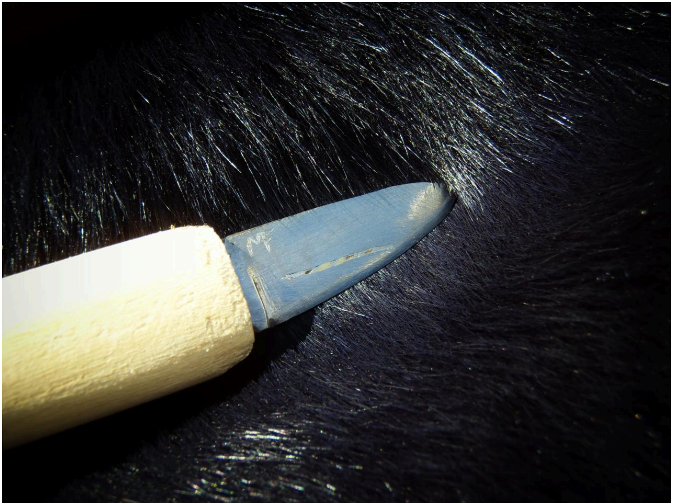
FIG 8C. A CLOSE UP OF THE BLADE'S RIGHT SIDE SHOWS THE MAKER'S MARK AND LITTLE IMPERFECTION ON THE INLAY. PHOTO BY MAURO FIORENTINI
