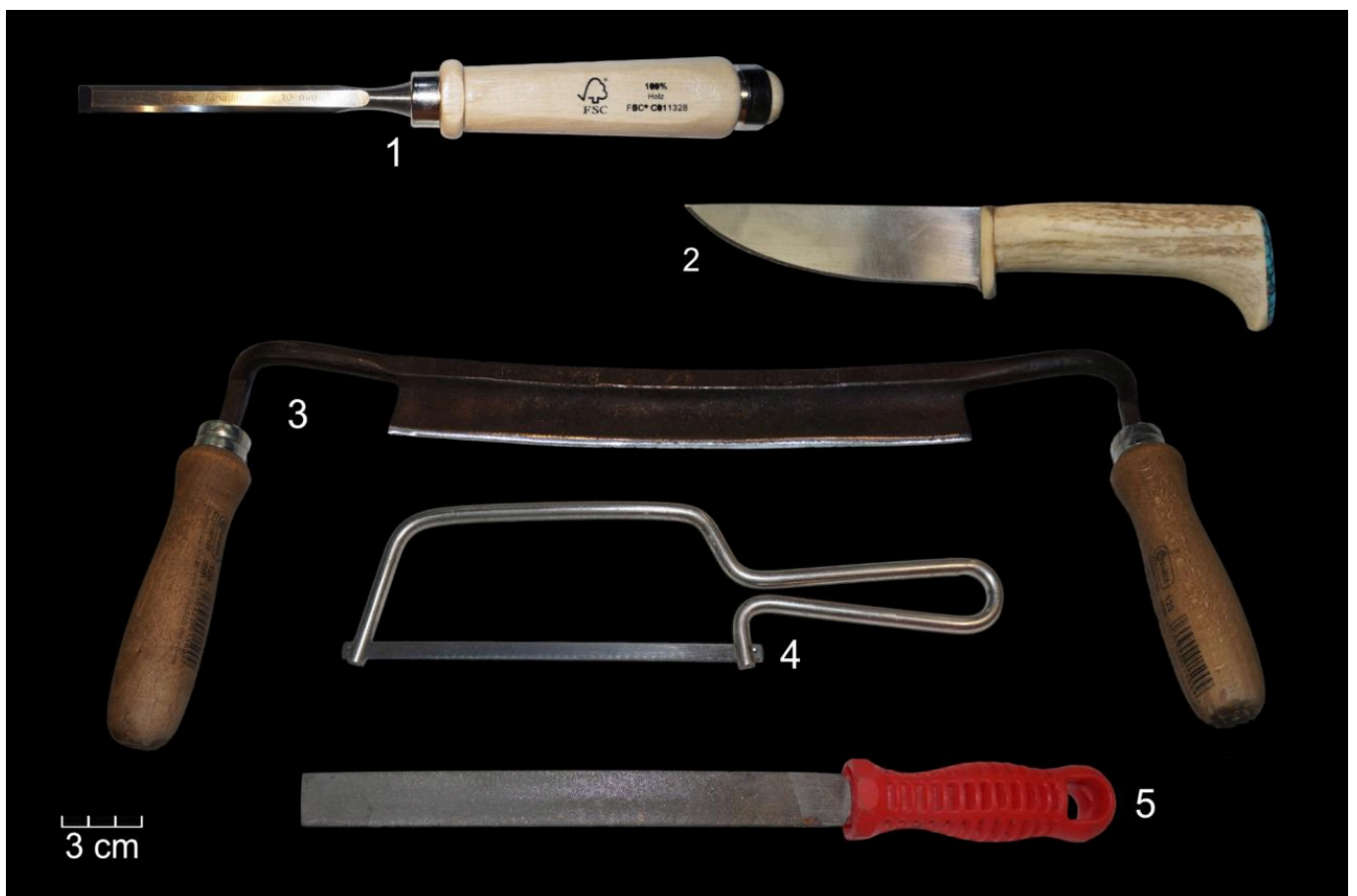
FIG 4. FOR THIS STUDY, MODERN METAL TOOLS WERE USED TO REPRODUCE MANUFACTURING TRACES EXPERIMENTALLY. THE FLAT CHISEL WAS 10 MM WIDE AND HAD A WEDGE ANGLE OF 45^\circ (1). THE KNIFE'S BLADE WAS 107 MM LONG, 30 MM WIDE, AND HAD A STRAIGHT SPINE AND A CONVEX CUTTING EDGE (2). THE BLADE OF THE DRAWKNIFE HAD A SLIGHT CURVATURE, WAS 29 MM WIDE AND 208 MM LONG (3). THE USED METAL SAW HAD
