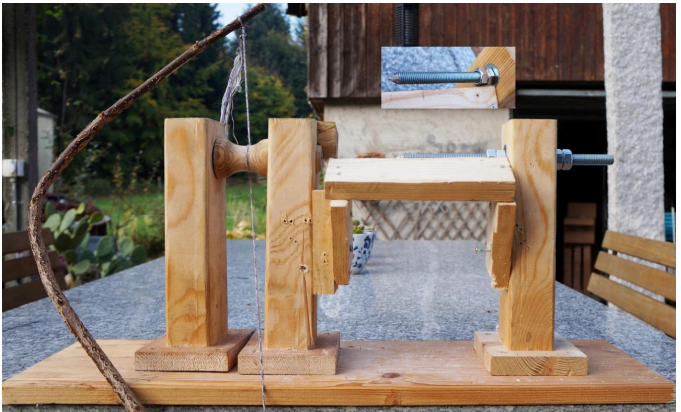
FIG 3. A SIMPLE WOODEN LATHE WITH A FIDDLE BOW DRIVE WAS BUILT TO PRODUCE REPLICAS. PHOTO BY HILDEGARD MÜLLER.
