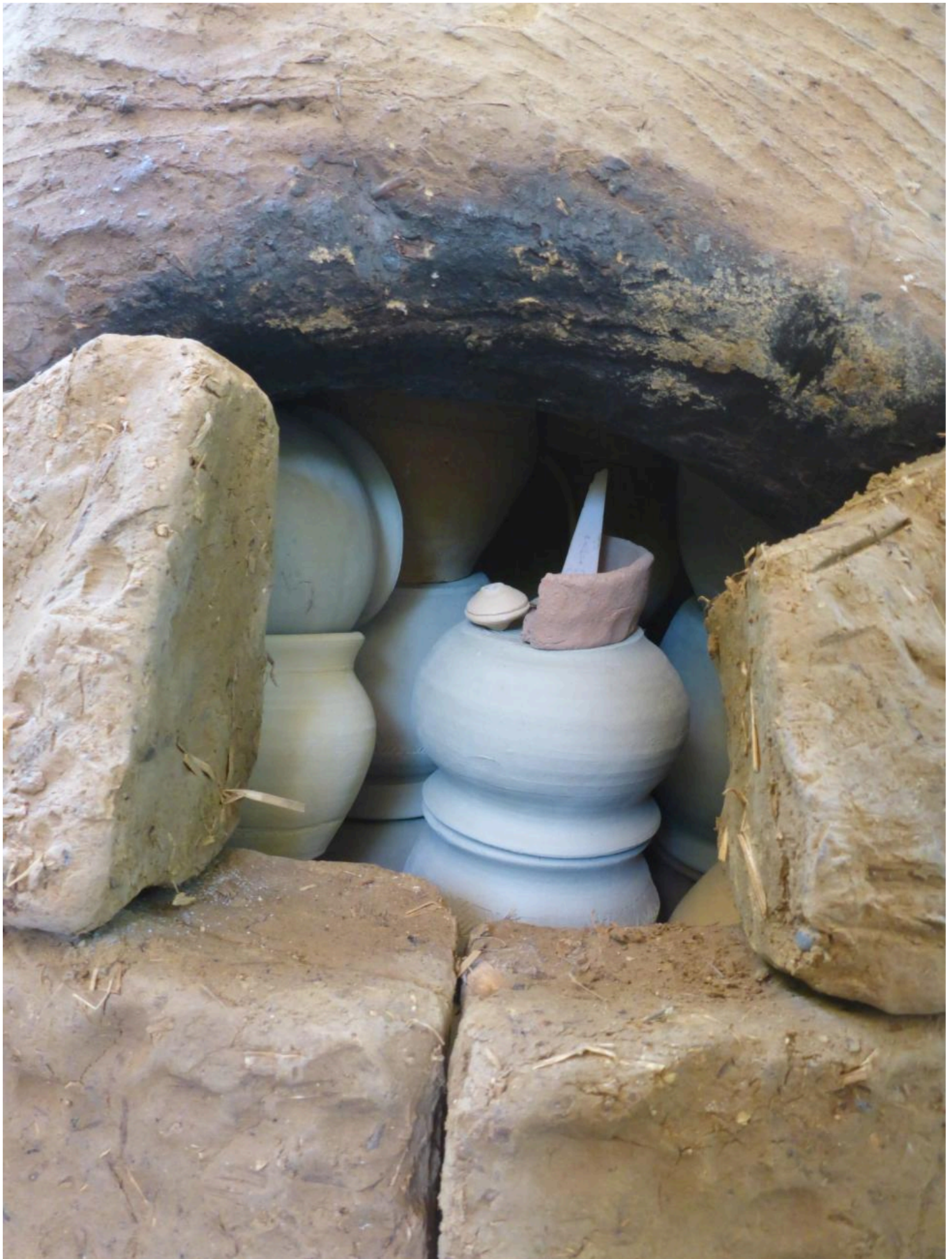
FIG 28. ONE BRICK OF THE LOADING DOOR IS NOT FIXED WITH CLAY GROUT, SO IT CAN BE REMOVED DURING THE FIRING TO PROVIDE A FIRE OBSERVATION HOLE, SO THE PYROMETRIC CONES OR THE HEAT RADIANT COLOR CAN BE CHECKED OR LITTLE SAMPLE VESSELS CAN BE PULLED OUT.
