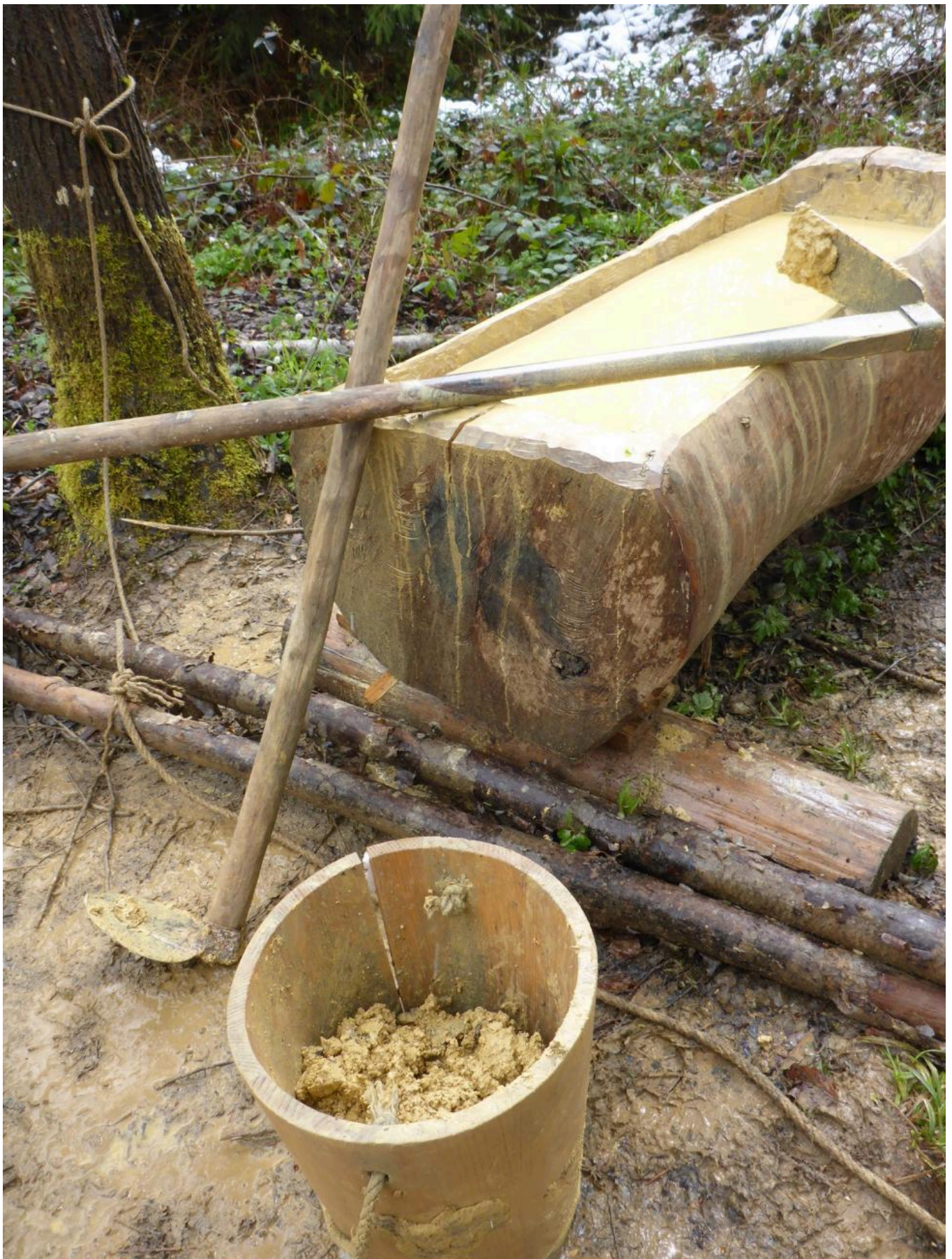
FIG 3. MIXING THE YELLOW CLAY WITH WATER IN A WOODEN TROUGH TO PREPARE THE LEVIGATION PROCESS.
