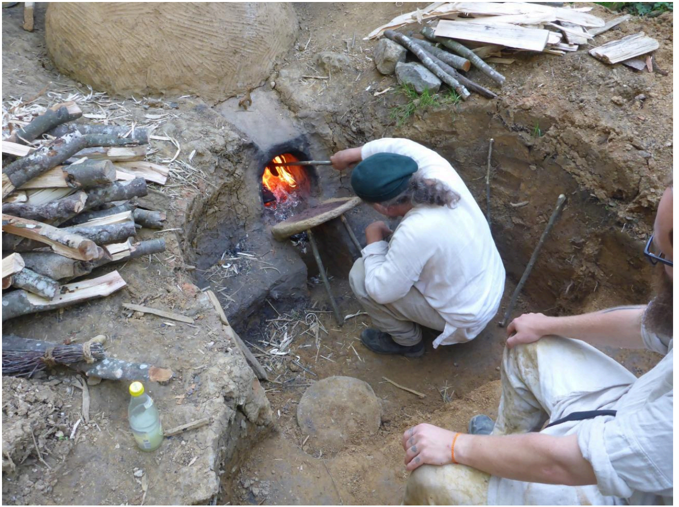
FIG 27. STOKE HOLE OF THE KILN DURING THE FIRING WITH KILN DOOR MADE OF COB.
