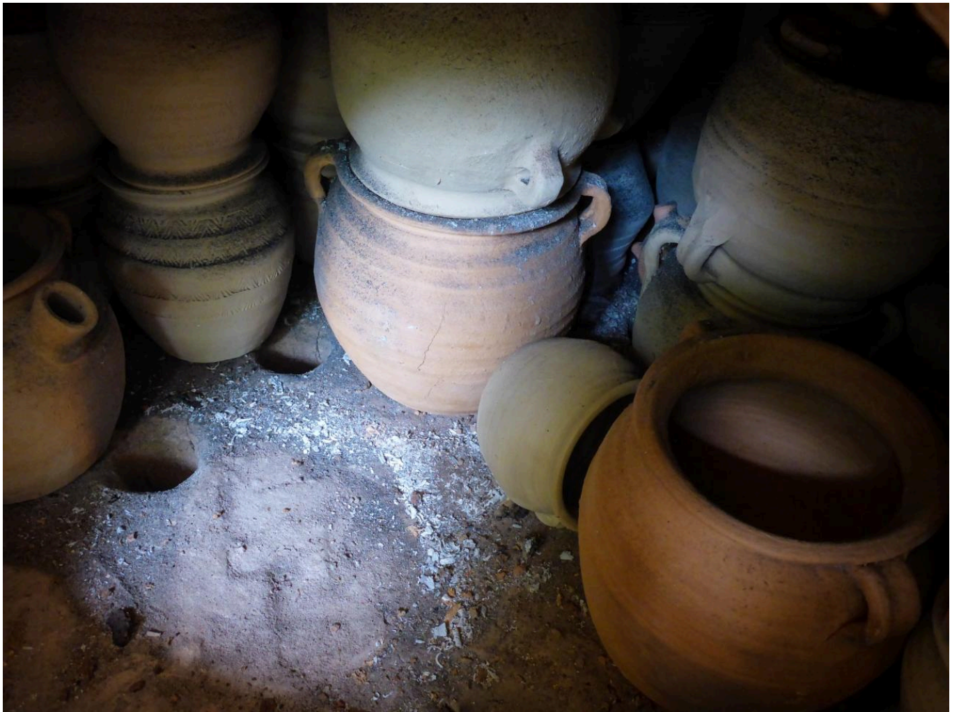
FIG 29. STACKS OF FIRED POTS ON THE PERFORATED FLOOR IN THE FIRING CHAMBER DURING THE UNLOADING OF THE FIRED WARE OUT OF THE KILN.
