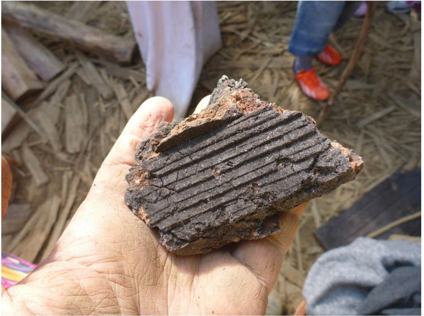
FIG 22. FRAGMENT OF THE RAISED KILN FLOOR WITH IMPRINTS OF THE SUPPORTING WOOD. THE FRAGMENT BROKE OUT DURING PREHEATING THE MOIST KILN FLOOR WITH A FIRE. TRACES OF WOOD LIKE THAT ARE FOUND ON FRAGMENTS OF ARCHEOLOGICAL KILNS (KELLER, 2007, FIG 9 AND 10).
