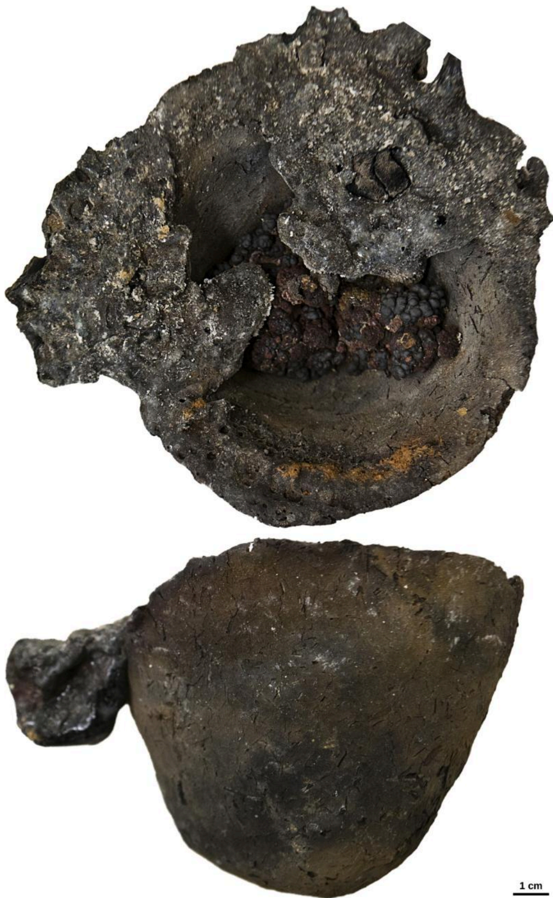
FIG 7. THE CRUCIBLE OF RUN 4 (FAZAEEL CLAY, TWO BELLOWS), PARTIALLY COVERED BY THE MELTED TUYÈRE MATERIAL. PHOTOS BY THOMAS ROSE.
