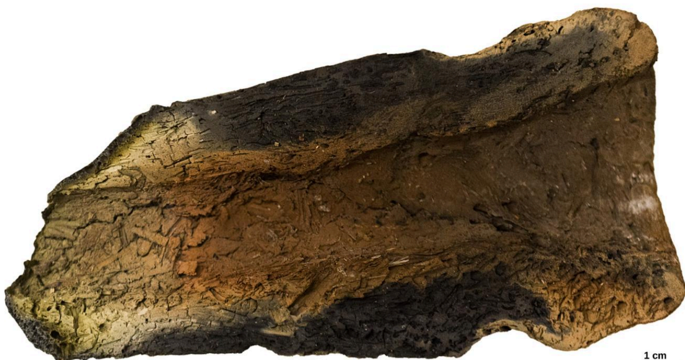
FIG 8. SELECTION OF TUYÈRES AFTER THE EXPERIMENT, SHOWING EXTENSIVE MATERIAL LOSS DUE TO MELTING (SEE FIGURE 2A FOR UNUSED TUYÈRES). THE TUYÈRE AT THE TOP LEFT AND THE CROSS-SECTION SHOW THE THIN LAYER OF MELTED CLAY ON THE SURFACE. PHOTOS BY THOMAS ROSE.
