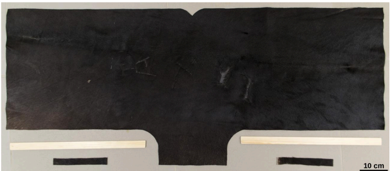
FIG 3A. THE BAG BELLOWS USED IN THE EXPERIMENT. PARTS OF THE BELLOWS BEFORE ASSEMBLING. PHOTO BY THOMAS ROSE.
