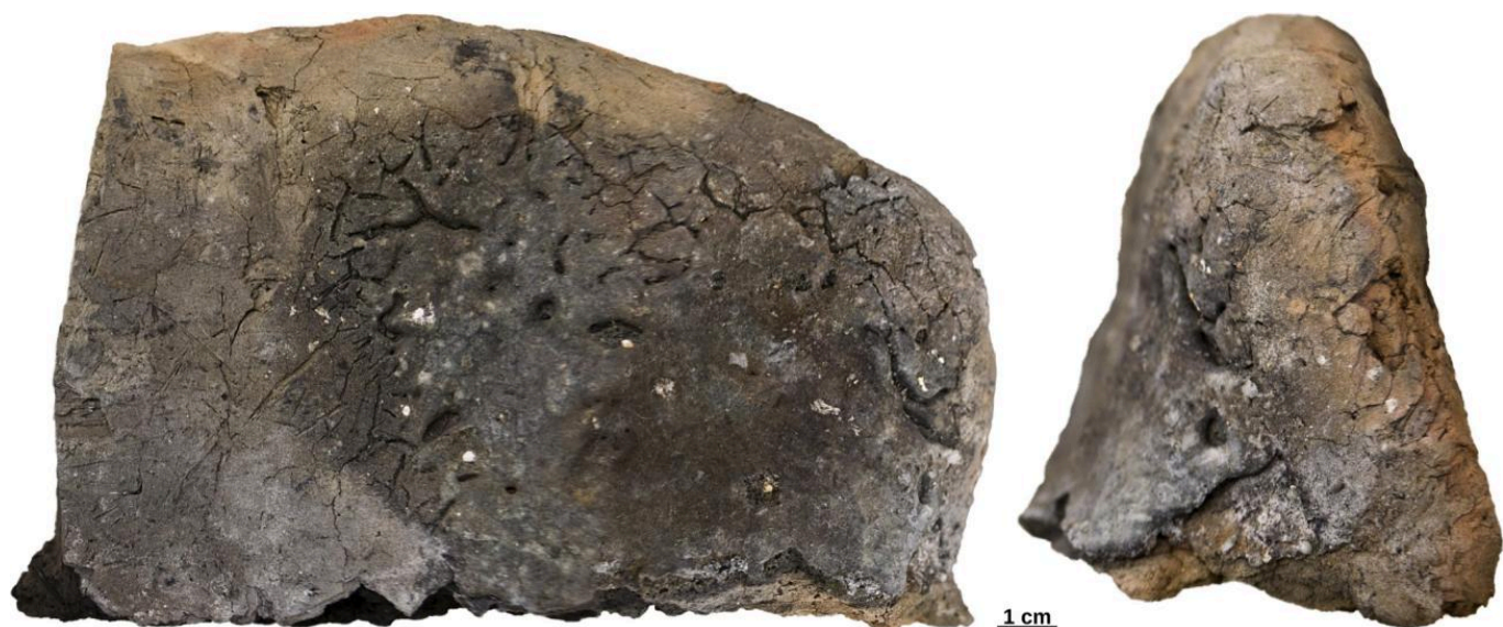
FIG 8. SELECTION OF TUYÈRES AFTER THE EXPERIMENT, SHOWING EXTENSIVE MATERIAL LOSS DUE TO MELTING (SEE FIGURE 2A FOR UNUSED TUYÈRES). THE TUYÈRE AT THE TOP LEFT AND THE CROSS-SECTION SHOW THE THIN LAYER OF MELTED CLAY ON THE SURFACE. PHOTOS BY THOMAS ROSE.
