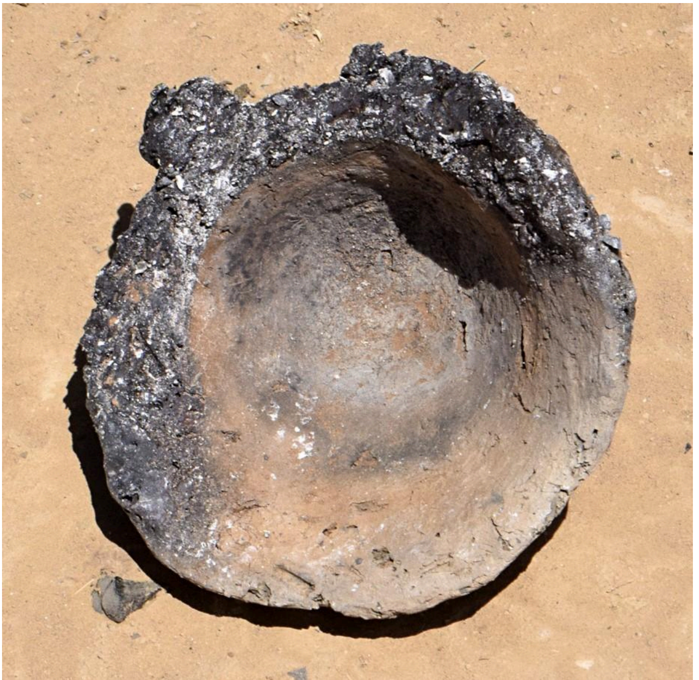
FIG 4A. THE CRUCIBLE OF RUN 1 (NEGEV LOESS). IN THE FIELD WHILE COOLING. PHOTO BY CÉCILE FOSSÉ.
