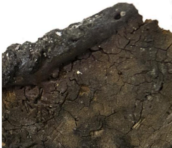
FIG 12. COMPARISON OF MELTING ON THE CRUCIBLE FROM RUN 1 (RIGHT) AND CRUCIBLE FRAGMENTS FROM ABU MATAR (LEFT, WITH CATALOGUE NUMBERS). ESPECIALLY THE TRANSITION BETWEEN FULLY MELTED AREAS AND UNMELTED AREAS BELOW THEM IS VERY SIMILAR. PHOTOS BY THOMAS ROSE.
