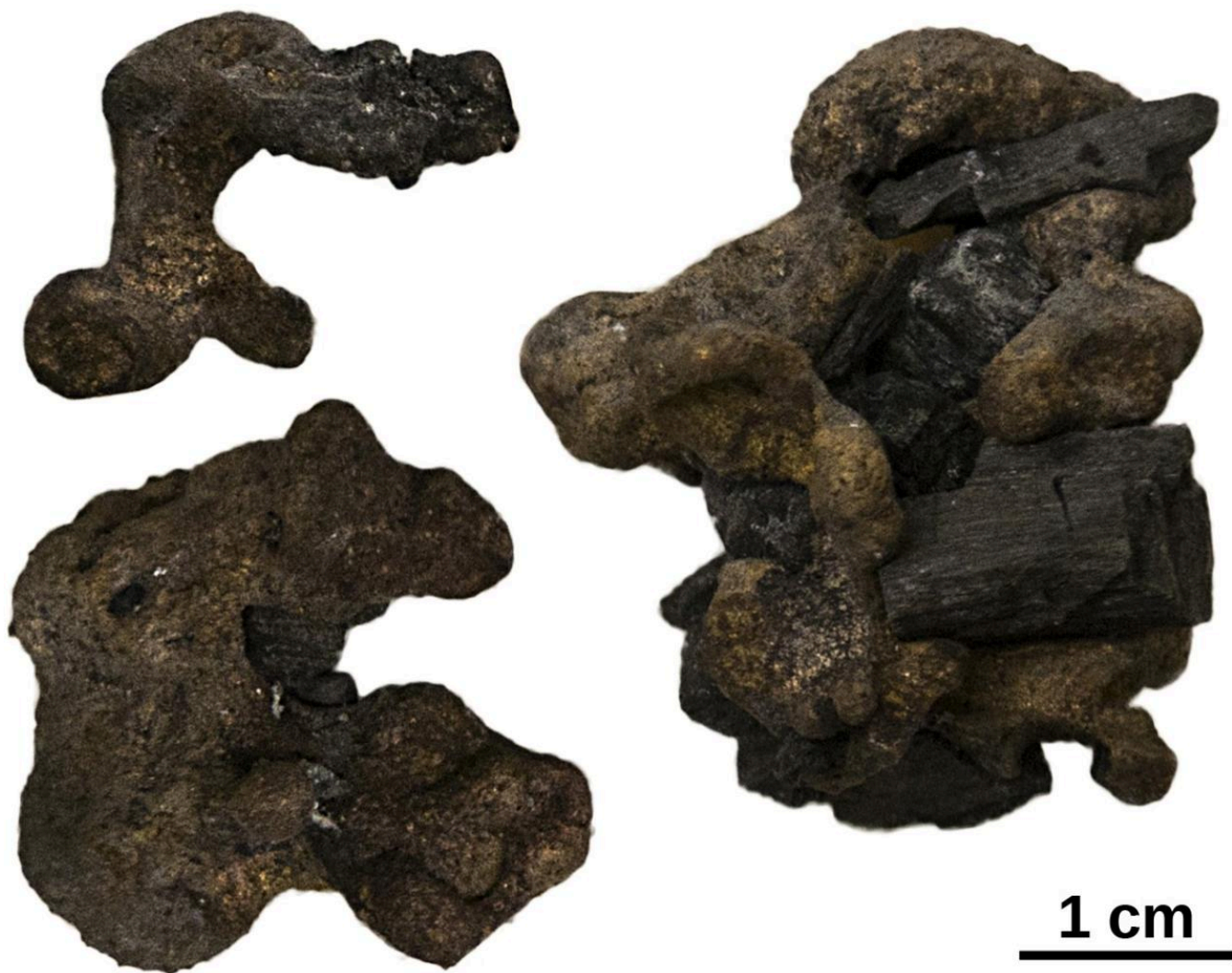
FIG 11. THE METAL LUMPS RECOVERED FROM THE CHARCOAL AFTER THE EXPERIMENTS. PHOTOS BY THOMAS ROSE.
