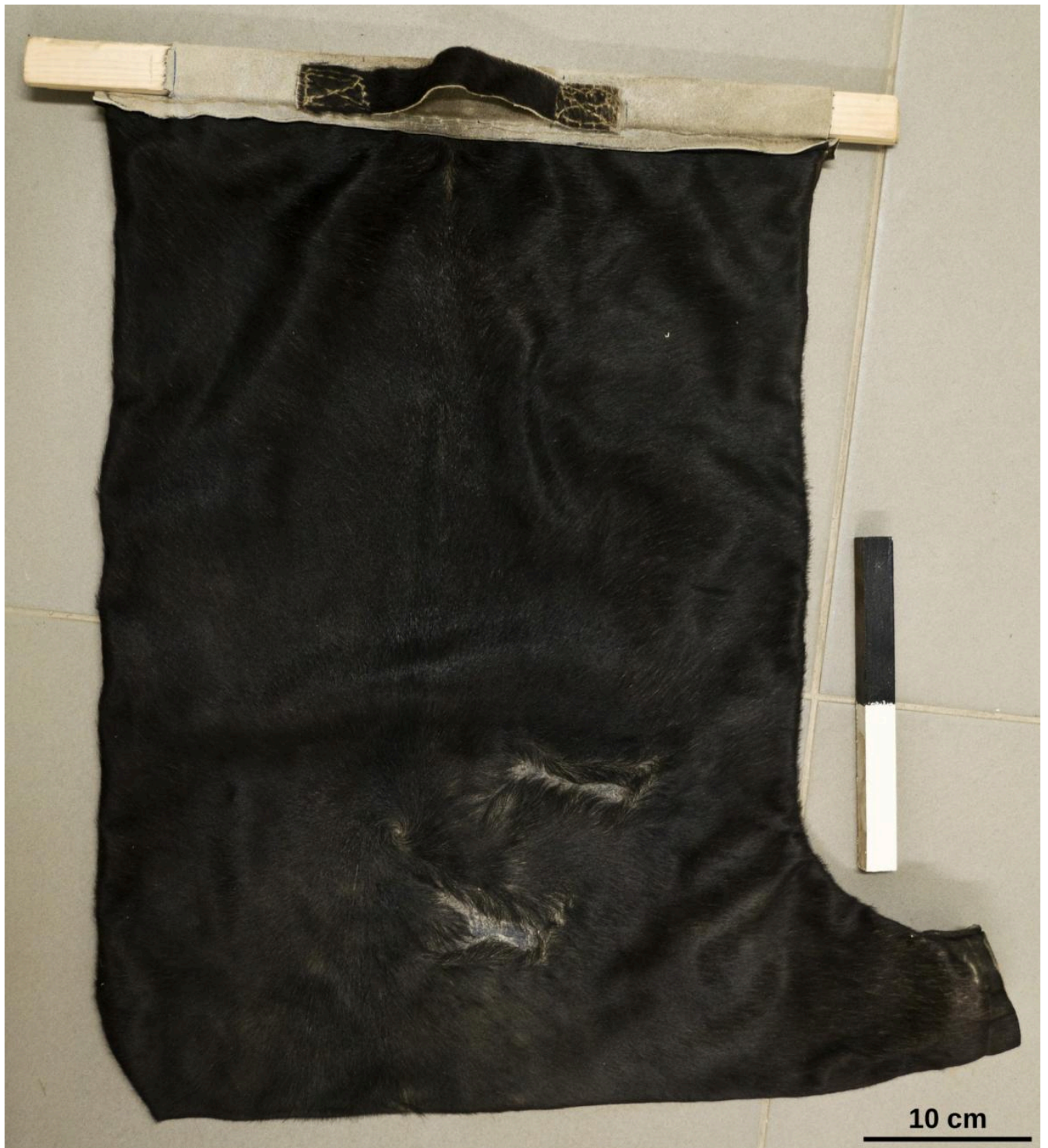
FIG 3B. THE BAG BELLOWS USED IN THE EXPERIMENT. THE ASSEMBLED BELLOWS AFTER THE EXPERIMENT. PHOTO BY THOMAS ROSE.
