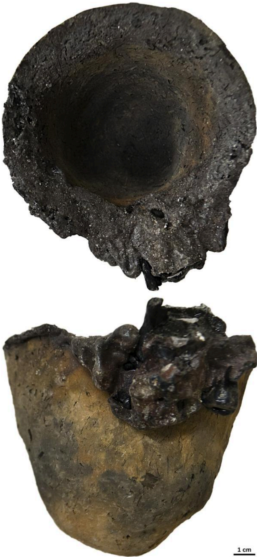
FIG 6. THE CRUCIBLE OF RUN 3 (FAZAEAL CLAY) WITH REMAINS OF THE MELTED TUYÈRE . PHOTOS BY THOMAS ROSE.
