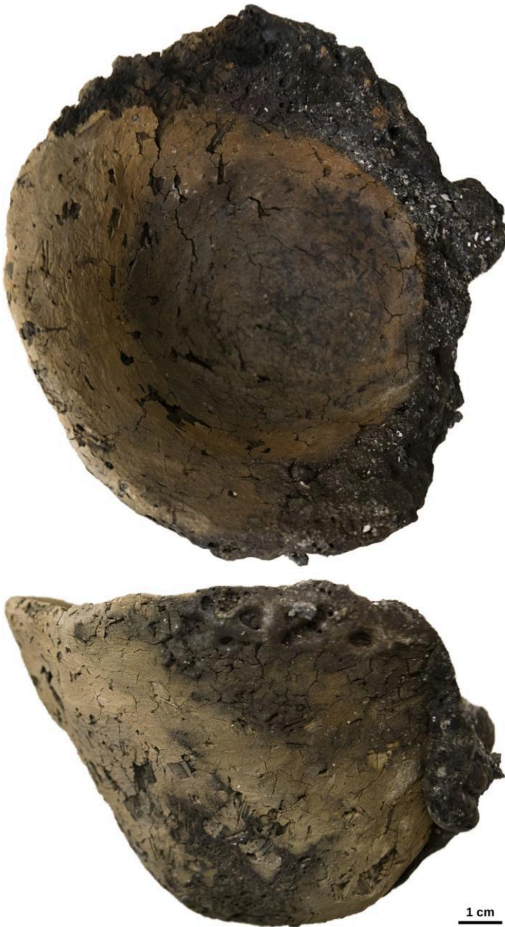
FIG 4B. THE CRUCIBLE OF RUN 1 (NEGEV LOESS). SEVERAL DAYS LATER. NOTE THE EXTENSIVE SPALLING THAT DEVELOPED IN THE MEANWHILE . PHOTOS BY THOMAS ROSE.
