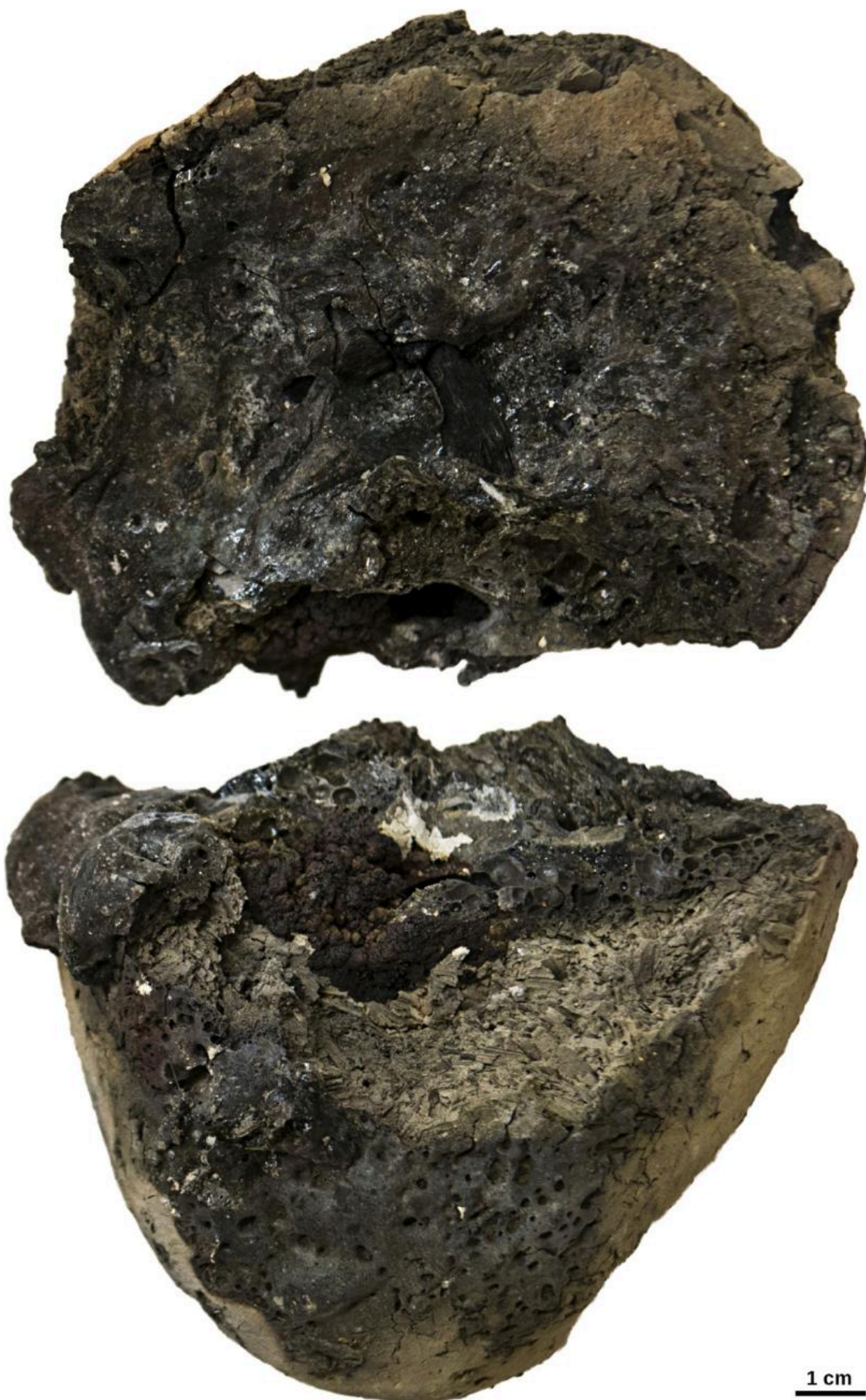
FIG 5. THE CRUCIBLE OF RUN 2 (NEGEV LOESS, WITH LID). THE CRUCIBLE WAS INTENTIONALLY BROKEN AT THE FRONT TO REMOVE THE TUYÈRE MELTED TO IT . PHOTOS BY THOMAS ROSE.
