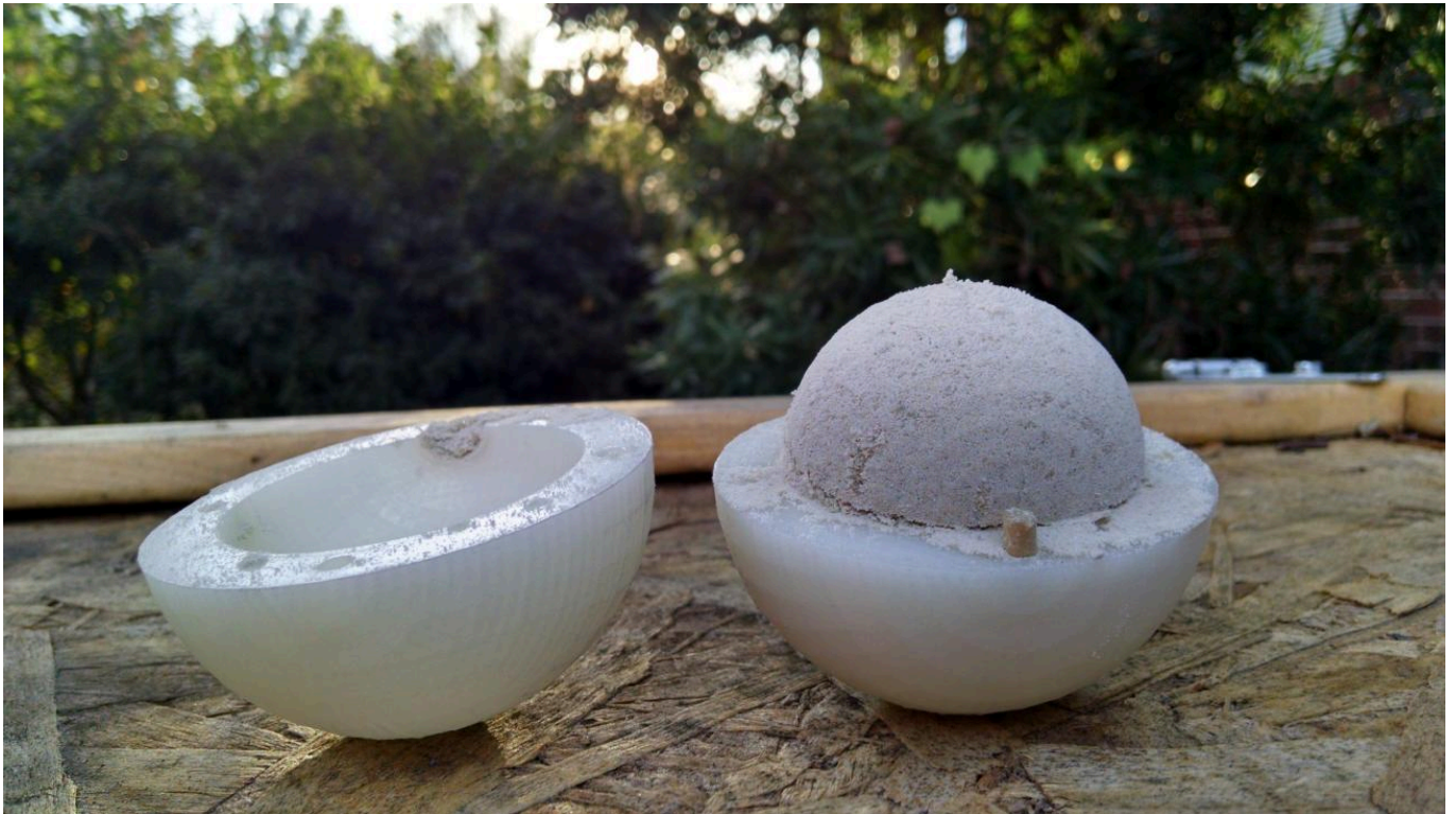
FIG 3. GREENSAND CORE FORMED USING THE 3D PRINTED GRENADE BLANK. (PHOTOGRAPH TAKEN BY AUTHOR).
