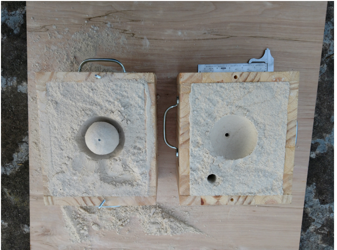
FIG 4. OVERVIEW OF THE GREENSAND MOLD WITH CORE FIXED IN PLACE. (PHOTOGRAPH TAKEN BY AUTHOR).
