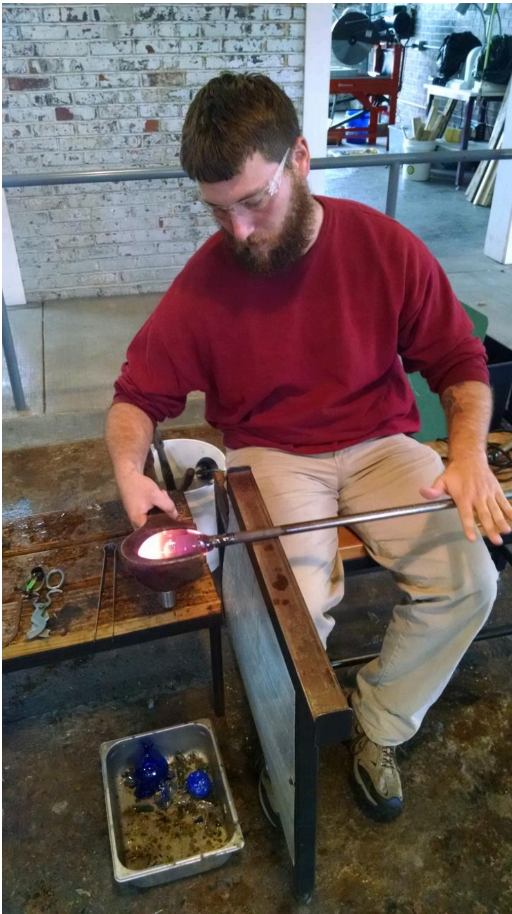
FIG 1. USING A WOODEN BLOCK TO FORM A GLASS GRENADE. (PHOTOGRAPH TAKEN BY MIKE TRACY).
