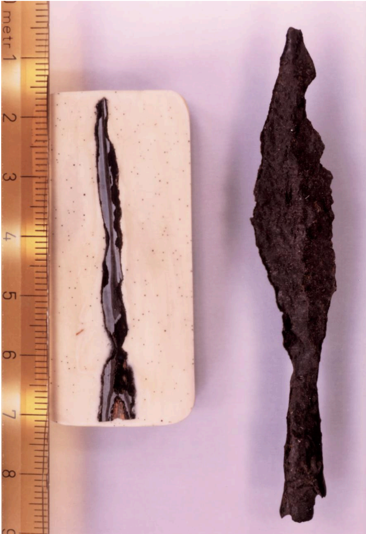
FIG 3. MULTI-LAYER STEEL (SANDWICH) STRUCTURE OF AN ALEMANNIC ARROWHEAD. 6/7TH CENT. PHOTO BY BECKER & RIESCH
