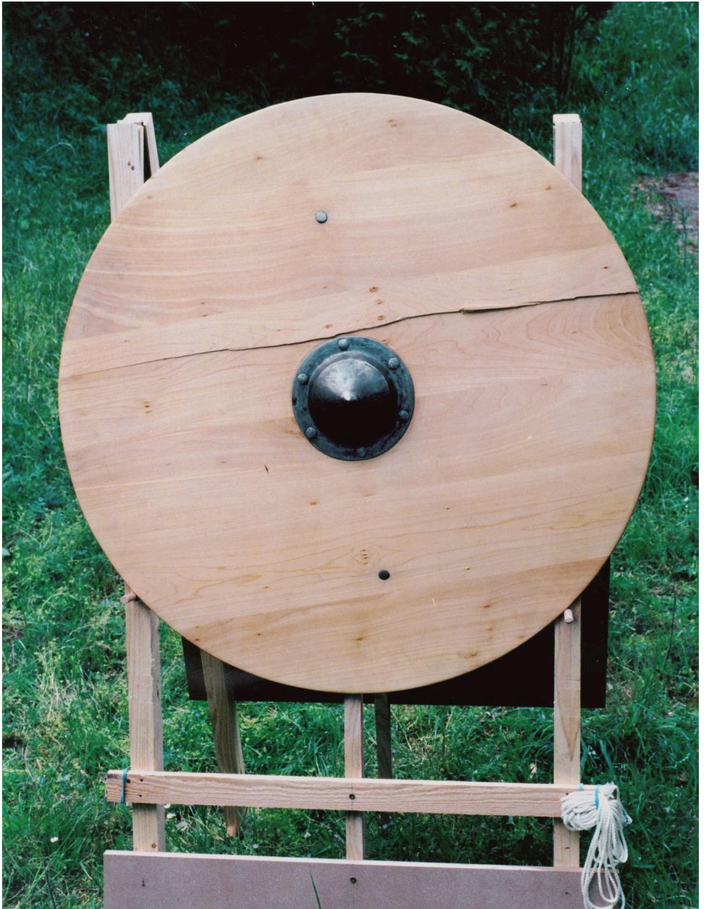
FIG 6. THE UNCOVERED SHIELD WITH AN IRON SHIELD-BOSS AND GRIP WAS SPLIT BY ONLY ONE SHOT. PHOTO BY HOLGER RIESCH
