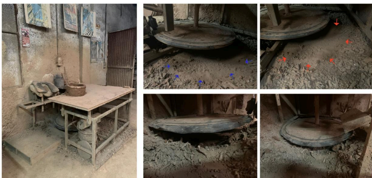
FIG 11. (LEFT). POTTER'S KICK-WHEEL USED TO MODEL POTTERY IN THE POTTERY WORKSHOP OF THE BROTHERS ANTONIO AND BARTOLOMÉ PADILLA HERRERA. (RIGHT) DETAIL OF THE LOWER PART OF THIS KICK WHEEL. THE ARROWS MARK THE CLEAR EVIDENCE OF WEAR CAUSED BY THE FRICTION OF THE BASAL WHEEL FROM DIFFERENT PERSPECTIVES.
