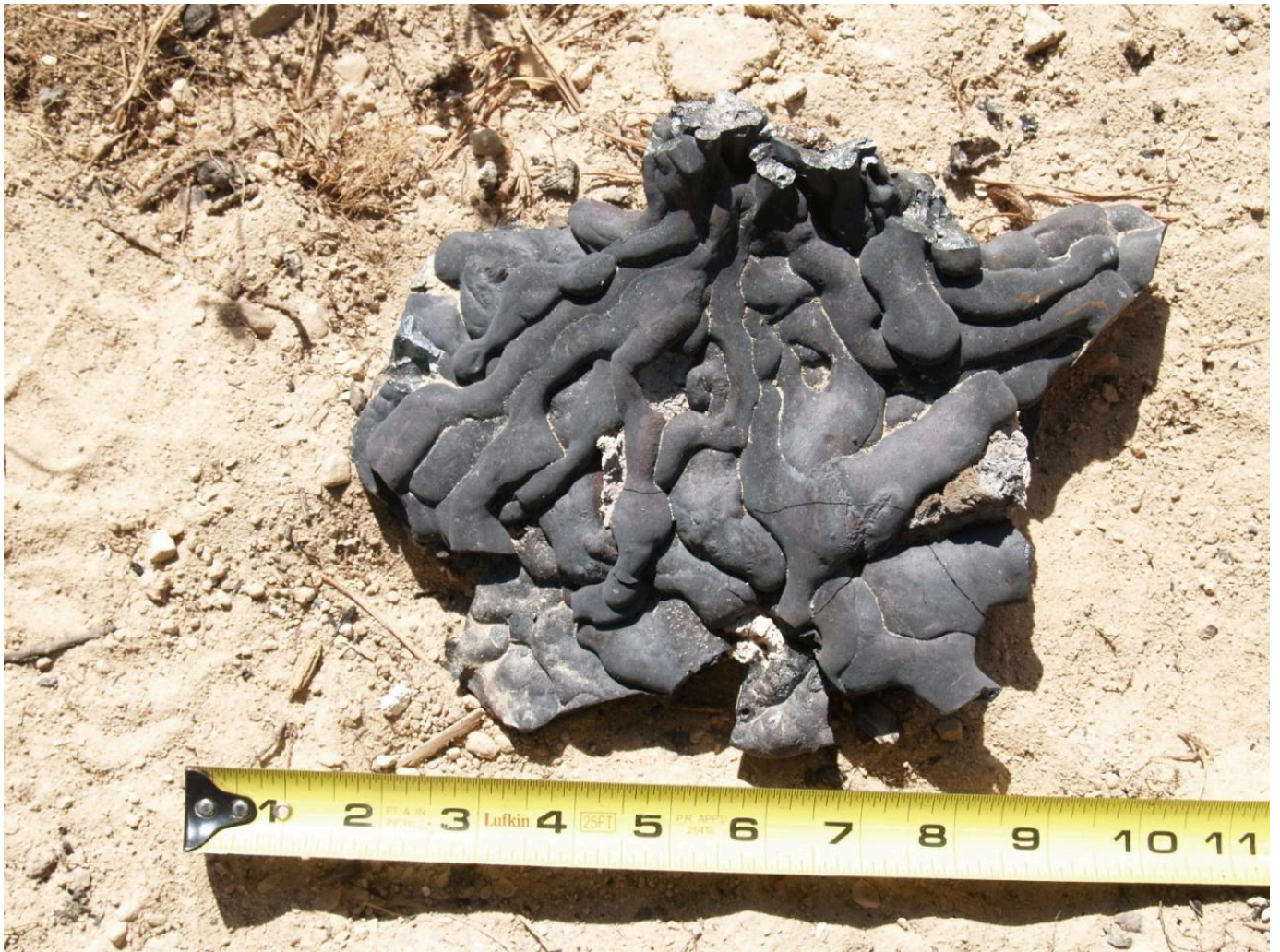
FIG 1B. BASIC SLAG TYPES: BLACK 'TAP' SLAG DENSE, 'MELTED CANDLE WAX' LOOK (FAST RUNNING AS TAPPED)
