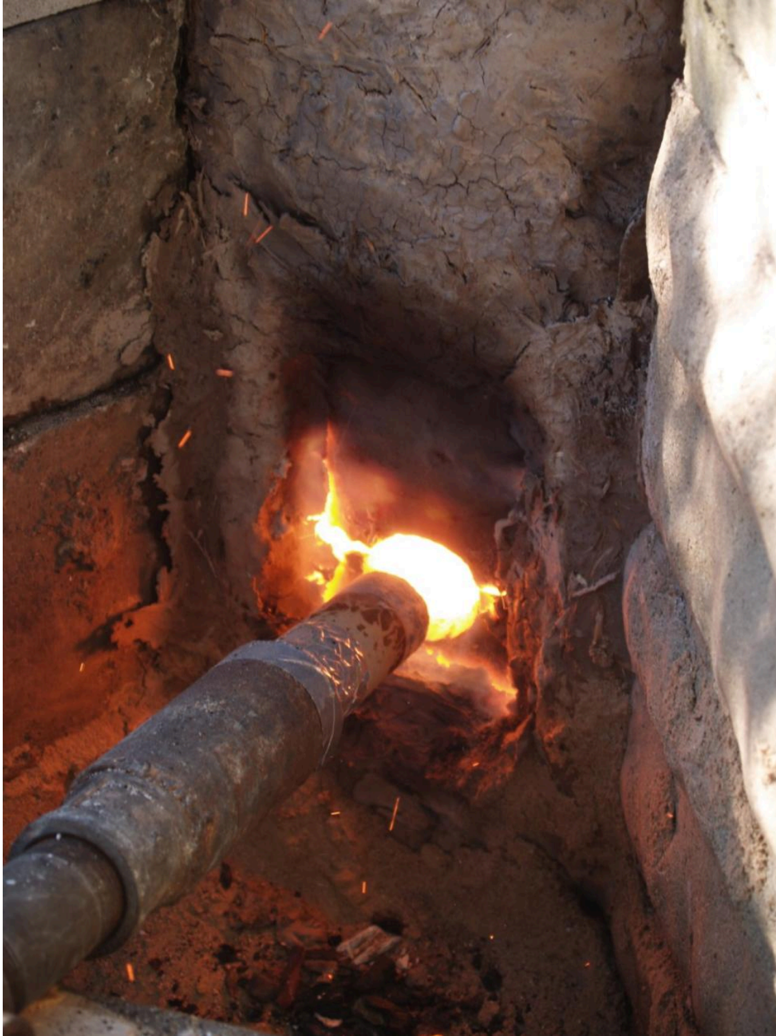
FIG 9. SHOWING USE OF THE BLOW HOLE AIR DELIVERY METHOD. ICELANDIC 3, 2008
