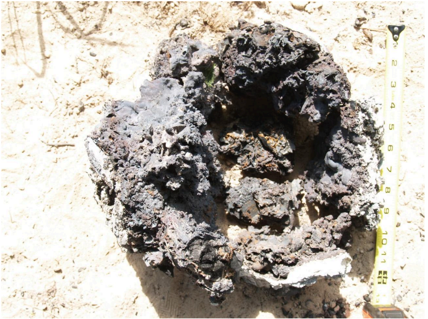
FIG 1C. BASIC SLAG TYPES: SLAG BOWL DARK GRANULAR SURFACES WITH PARTICLES OF IRON INCLUDED
