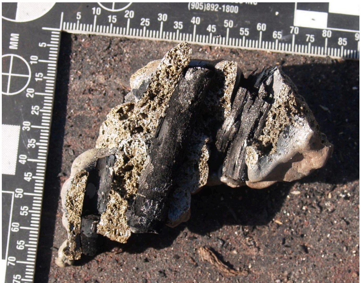
FIG 1A. BASIC SLAG TYPES: GREEN 'SILICA' SLAG LIGHT AND FROTHY (SLOW MOVING AS TAPPED)
