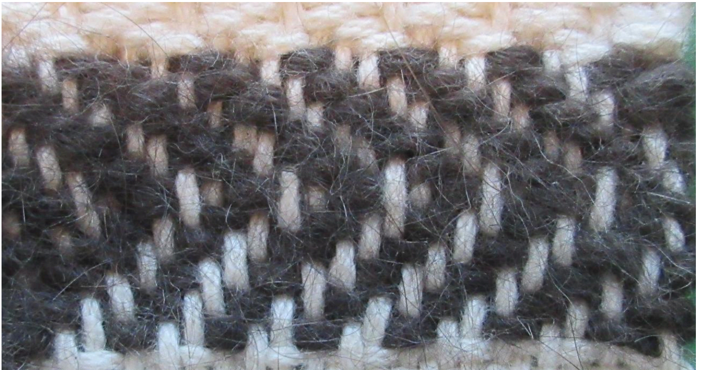
FIG 13. THE 2/1 TWILL WEAVE PRODUCED IN THIS EXPERIMENT. PHOTO BY BILLIE J. A. FOLLENSBEE
