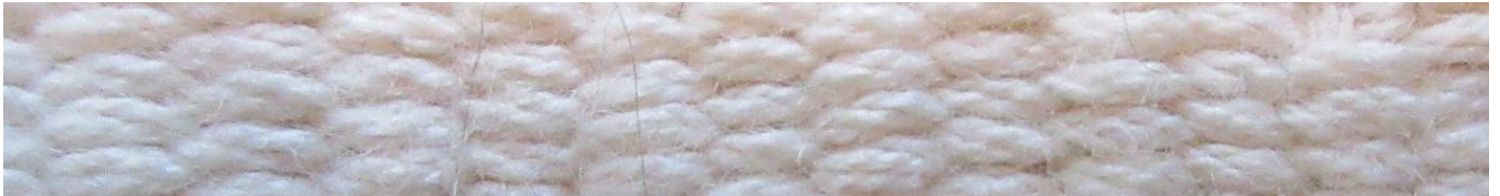
FIG 12. THE WEFT-FACED 2/2 TABBY WEAVE PRODUCED IN THIS EXPERIMENT. PHOTO BY BILLIE J. A. FOLLENSBEE
