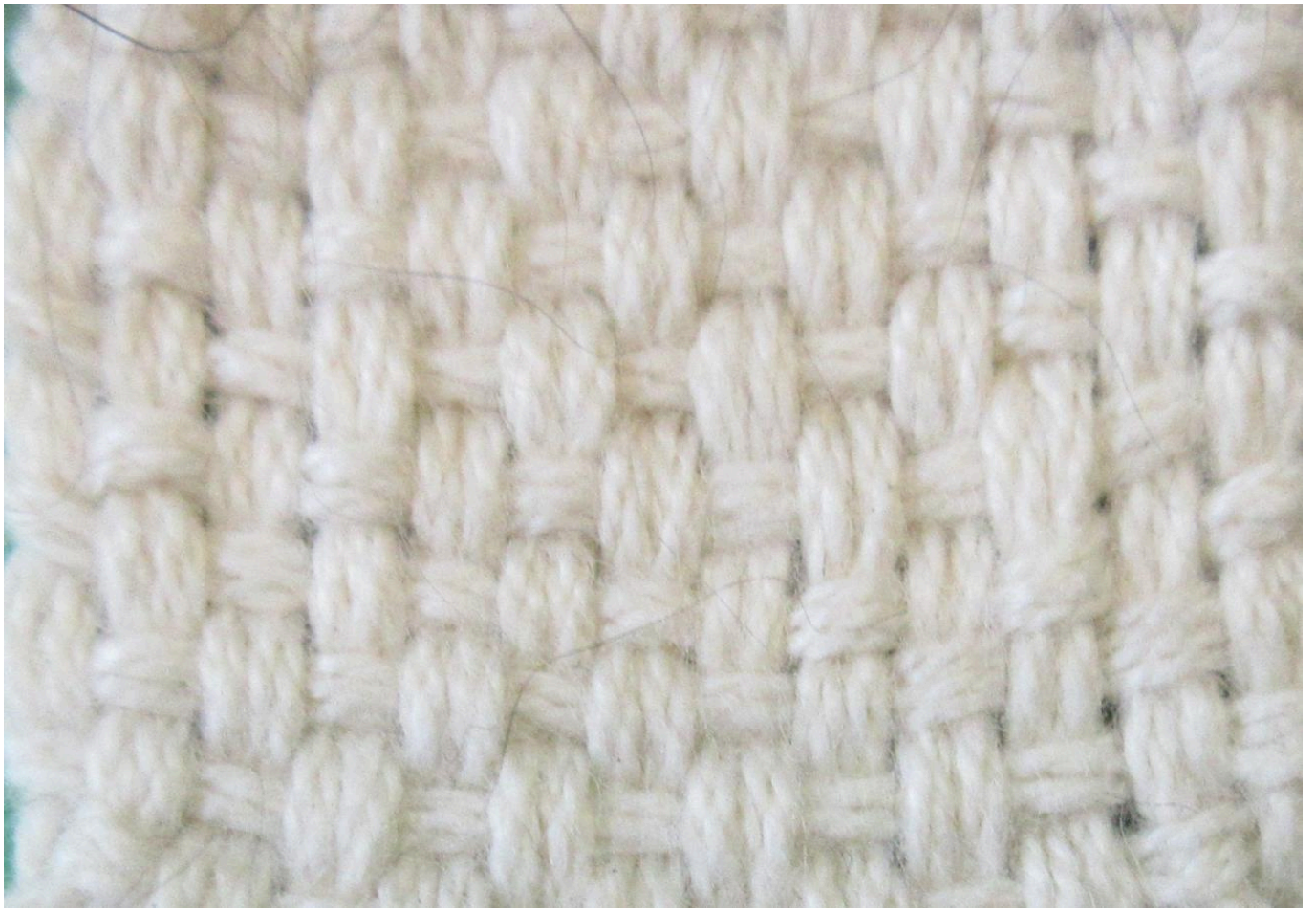
FIG 17. THE BASKET WEAVE PRODUCED IN THIS EXPERIMENT. PHOTO BY BILLIE J. A. FOLLENSBEE
