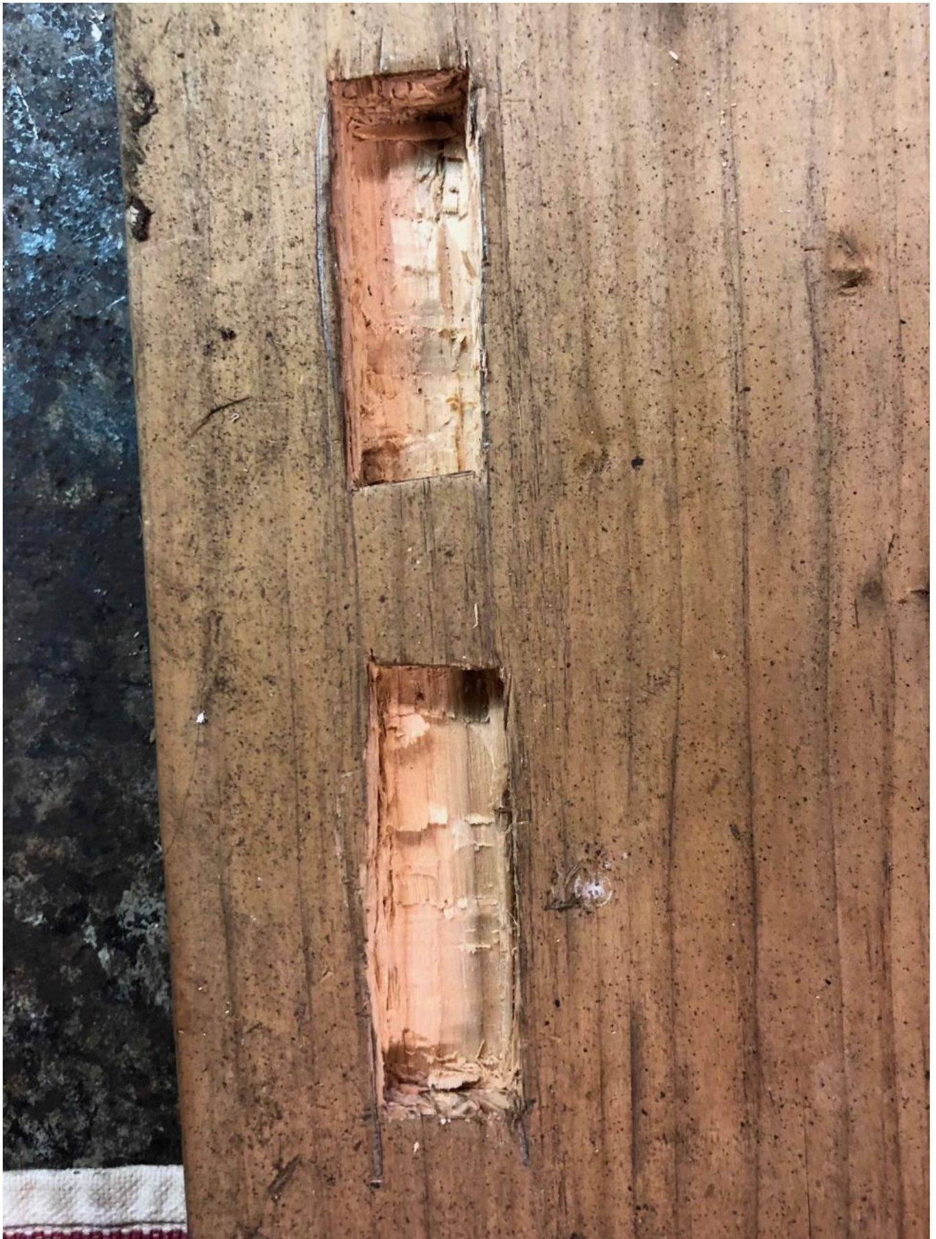
FIG 3. NOTCHES CUT INTO A PINE WOOD BOARD WITH A CHISEL APPROXIMATELY 2"X ½" X 3/8" DEEP.
