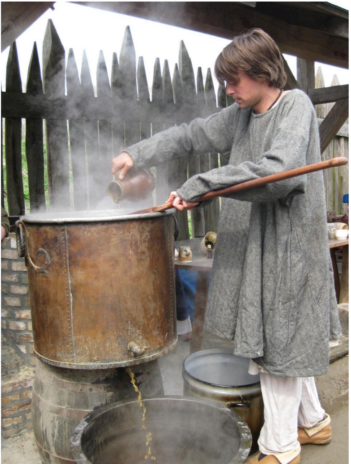
FIG 32. LAUTERING: CLOUDY WORT IS POURED THROUGH THE MASH UNTIL IT RUNS CLEAR. COPYRIGHTS BY MERRY DINELEY
