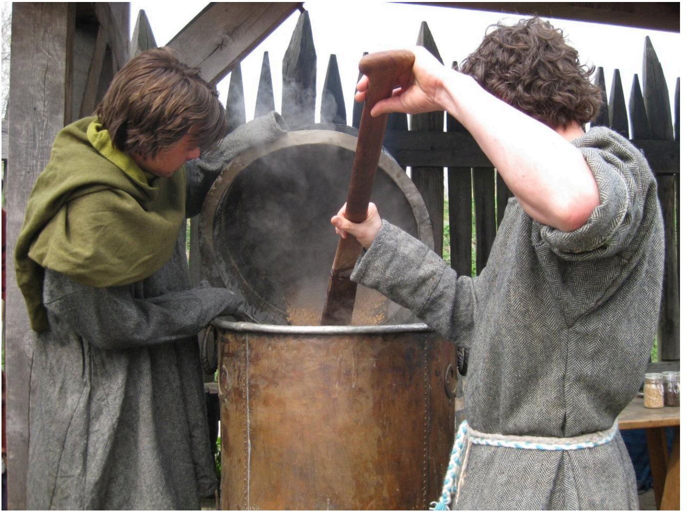
FIG 31. THE LAST OF THE MASH IS TRANSFERRED TO THE LAUTER TUN BY TIPPING THE STILL HOT MASH TUN. COPYRIGHTS BY MERRY DINELEY
