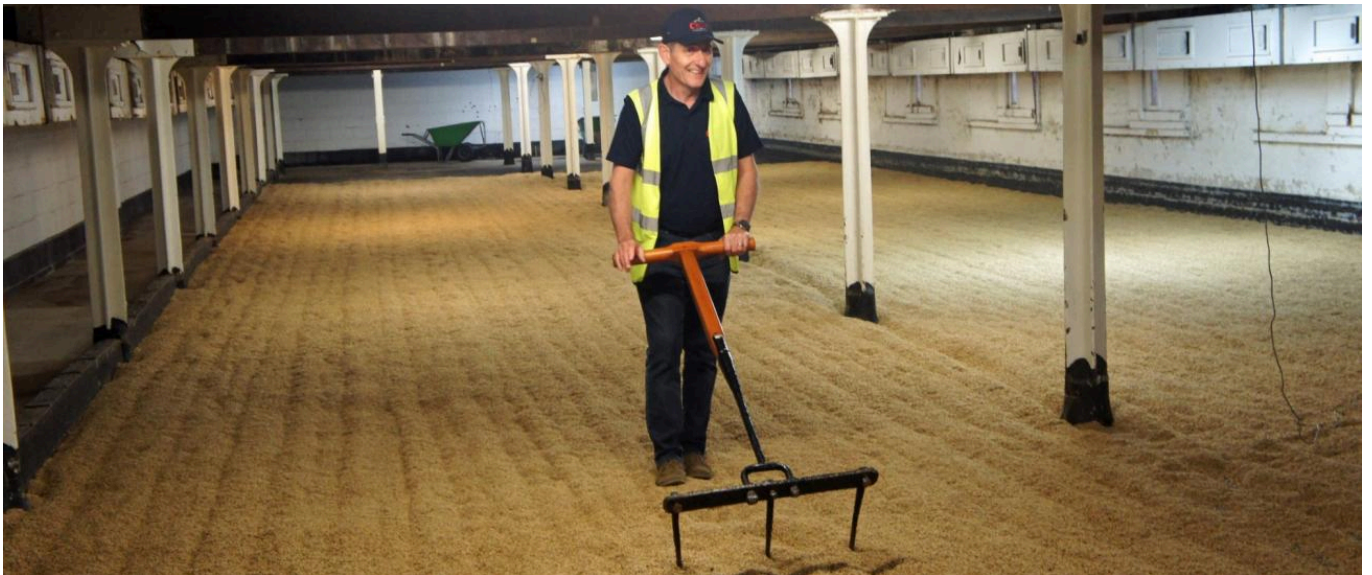
FIG 12. A MALTMAN RAKING THE MALT IN A FLOOR MALTINGS AT CRISP'S MALTINGS, GREAT RYBURGH, NORFOLK. COPYRIGHTS BY MARTYN CORNELL
