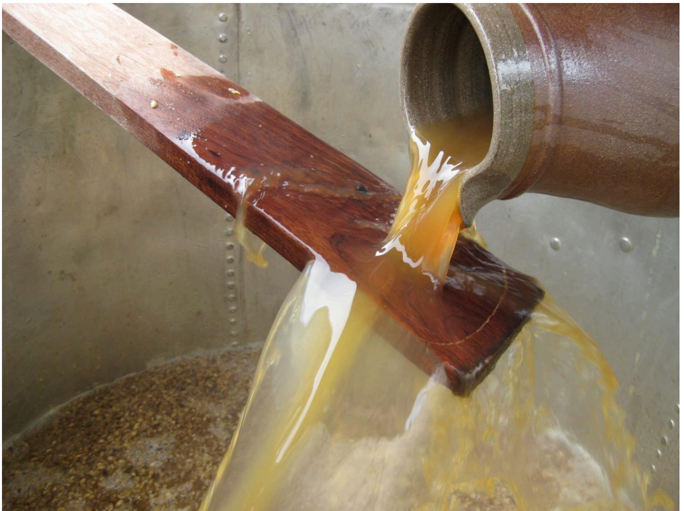
FIG 33. A CLOSE UP OF LAUTERING: WORT IS POURED OVER THE MASH PADDLE TO AVOID DISTURBING THE GRAIN BED. COPYRIGHTS BY MERRYN DINELEY
