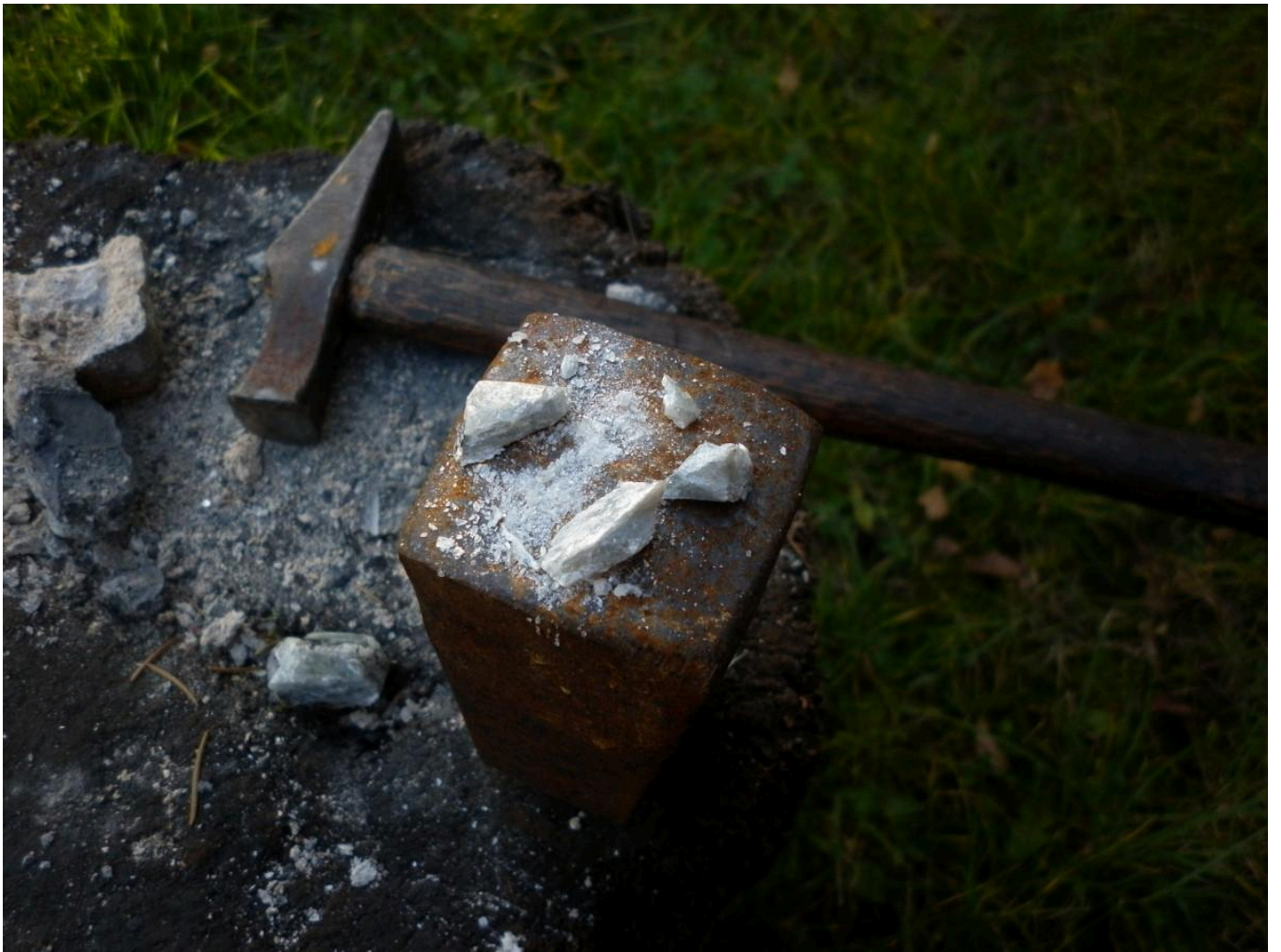
FIG 10. SAPPHIRE BREAKING FOR BURINS. PHOTO BY IRENA PODOLSKA
