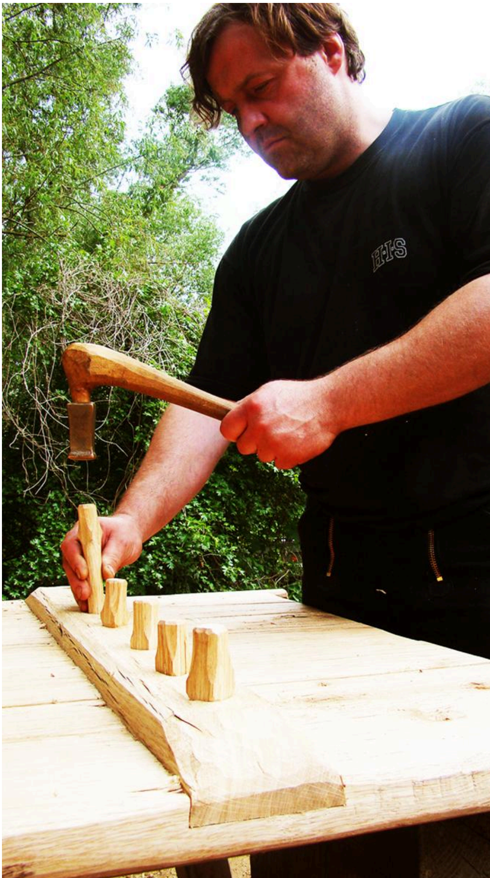
FIG 13. THE RECTANGULAR BOARDS OF THE DOORS WERE FIXED TOGETHER WITH CONICAL PLANKS OF TRAPEZE-FORMED CROSS-SECTION, WHICH WERE INSERTED CROSSWISE IN WELL MATCHED GROOVES AND FIXED WITH WOODEN PEGS. COPYRIGHT: WOLFGANG LOBISSER
