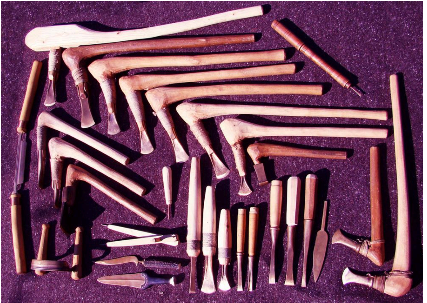
FIG 2. REMAKES OF BRONZE AGE TOOLS THAT WERE USED TO BUILD THE NEW LONGHOUSE MODEL: AXES, ADZES, CHISELS, CARVING KNIVES, DRAWING KNIVES, DRILLS, HAMMERS, GOUGES, COMPASSES, AND AWLS. COPYRIGHT: WOLFGANG LOBISSER
