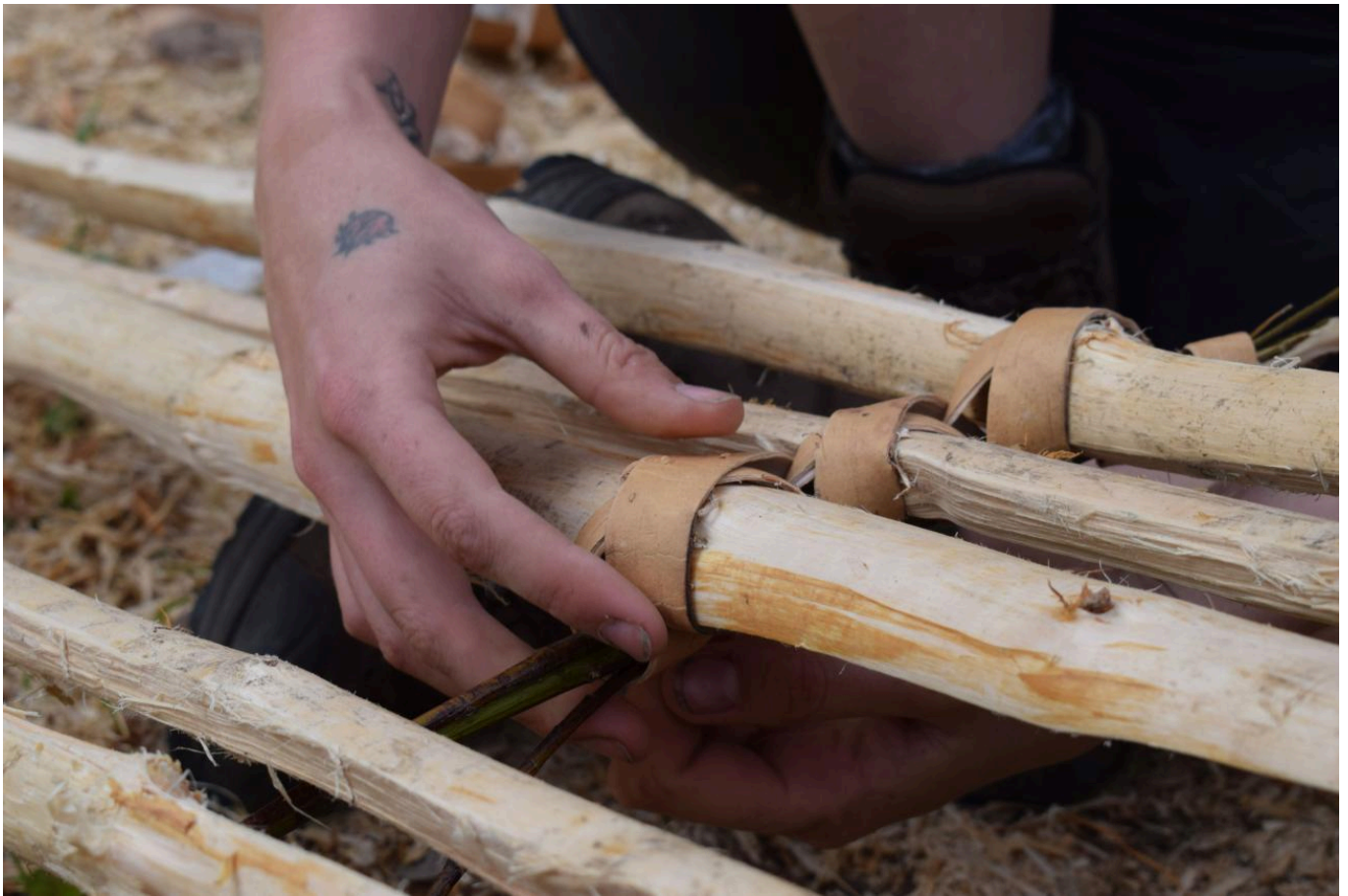
FIG 10B. BINDING THE WILLOW RODS TO THE SLATS USING THE HEAT-TREATED STRIPS OF BIRCH BARK. PHOTO BY JAMES FINDLAY
