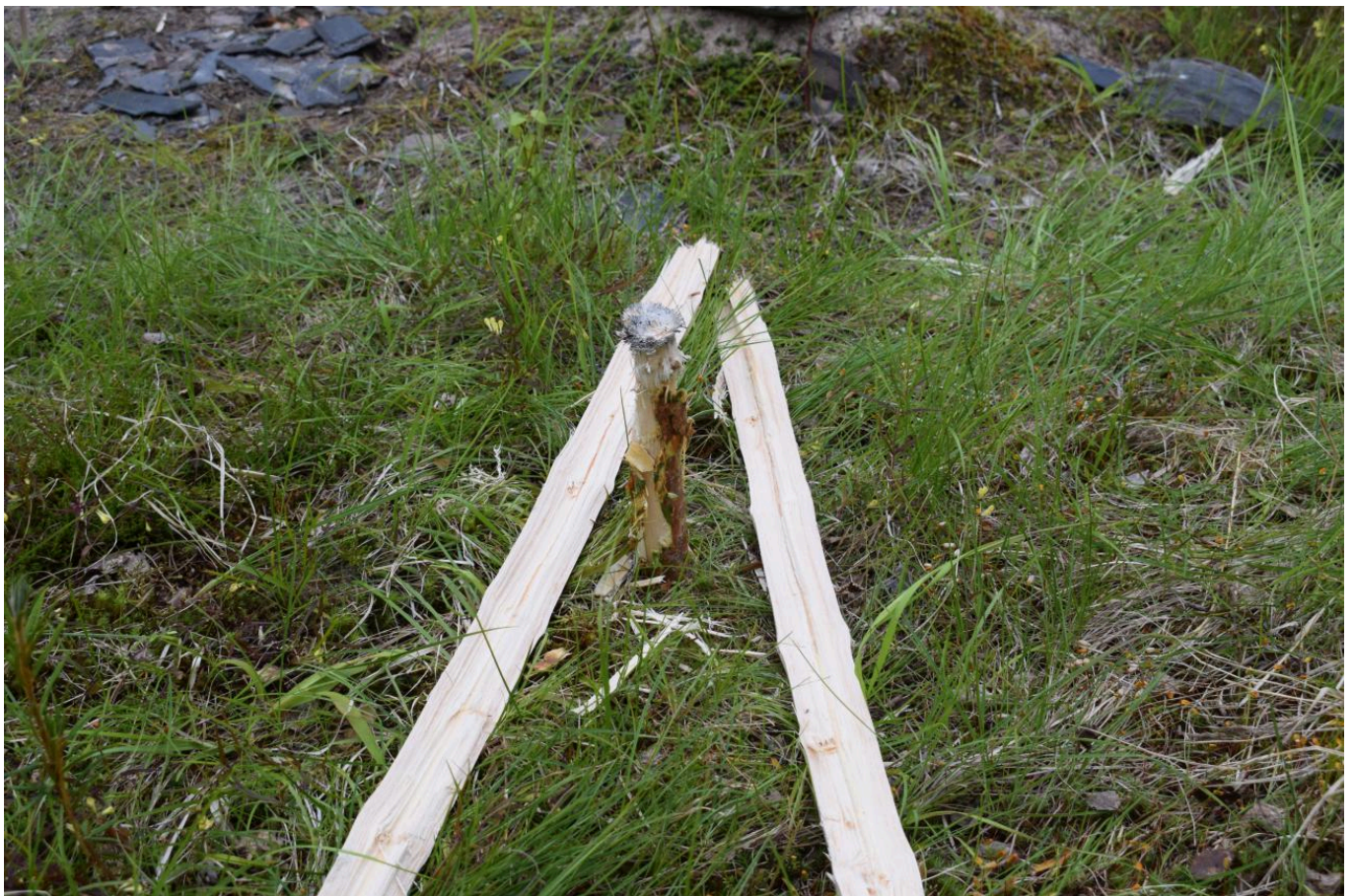
FIG 8B. THE RESULTANT (RIVEN) SPLITTING OF THE STRIPPED PINE. PHOTO BY JAMES FINDLAY
