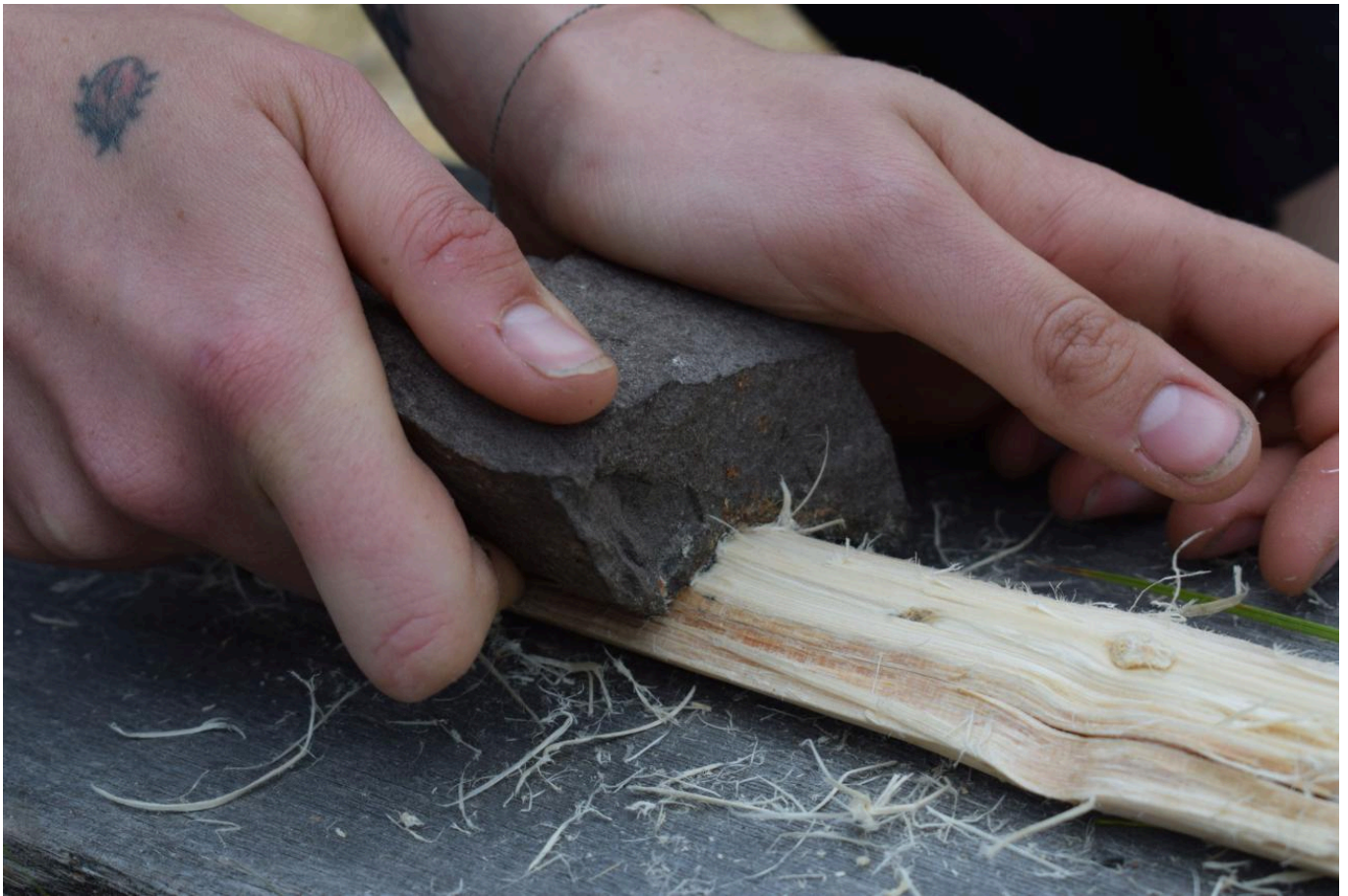
FIG 9. SHAPING THE RIVEN SLAT USING AN UNMODIFIED LOCALLY SOURCED PIECE OF SLATE. PHOTO BY JAMES FINDLAY
