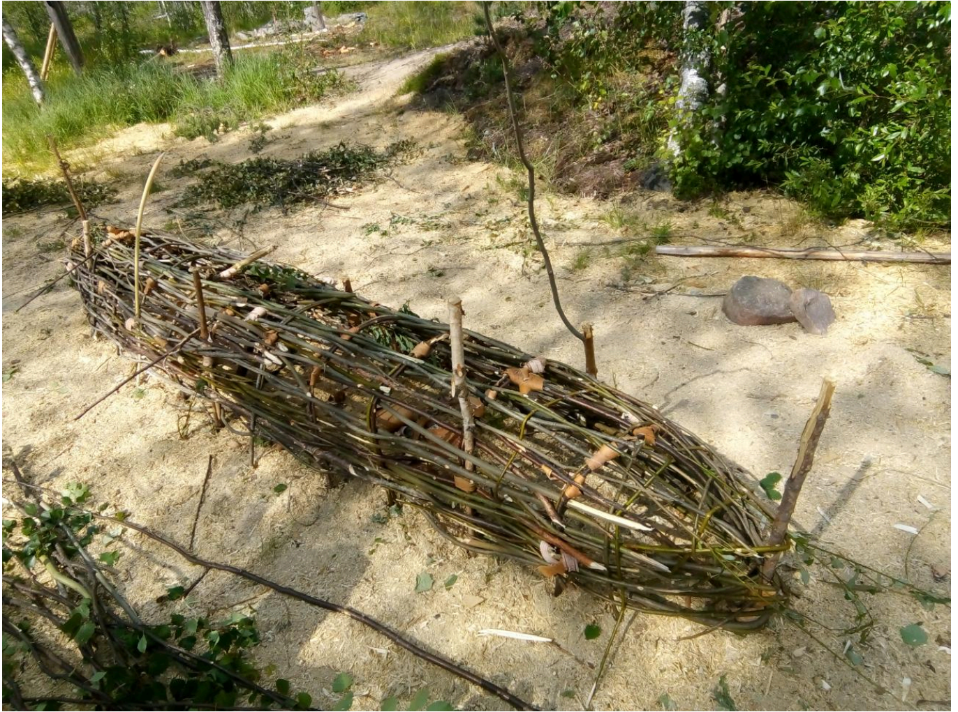
FIG 3. THE OUTER BASKETRY FRAME PRIOR TO TURNING UPRIGHT AND ADDITION OF THE THWARTS. ADDITIONAL SHORT RODS ARE HOLDING THE TENSION IN THE WEAVE. PHOTOGRAPH PATRICK SWEENEY.
