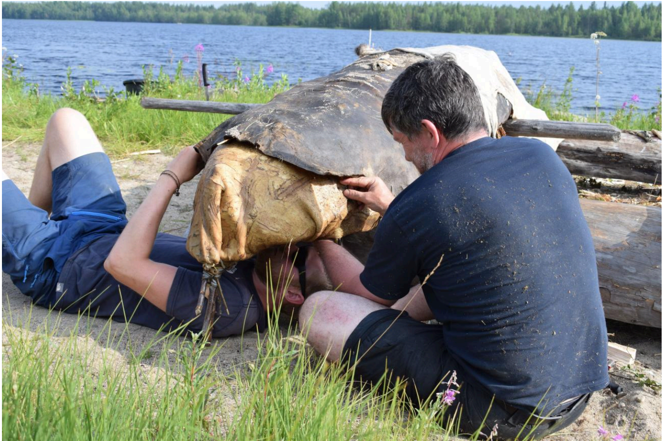
FIG 6. THE HIDES AT THE STERN BEING DOUBLE STITCHED TOGETHER USING THIN RAWHIDE LACING. PHOTOGRAPH JAMES FINDLAY.
