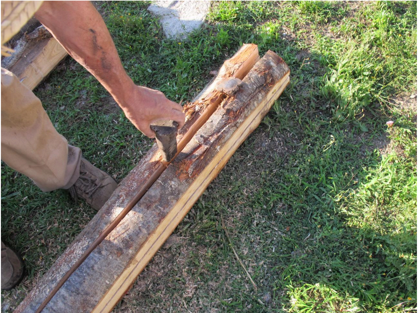
FIG 15. USING BIG METAL NAILS TO CUT TRUNKS
