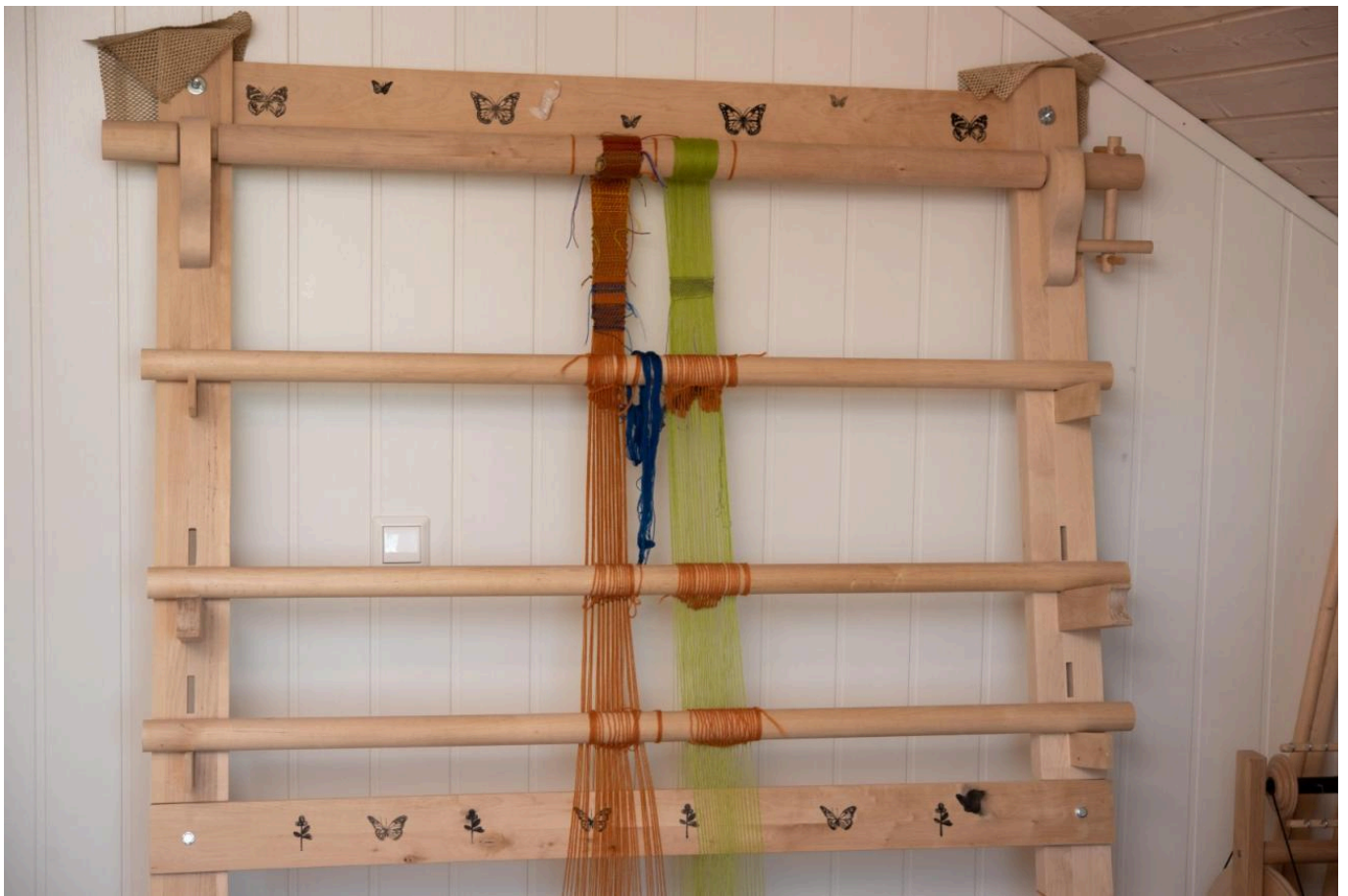
FIG 8. THE WARP-WEIGHTED LOOM WITH THE 3/1 CHEVRON TWILL TO THE LEFT AND THE PLAIN 2/2 TWILL TO THE RIGHT. PHOTO BY RUNE AASEN, LEVANGER (NO)
