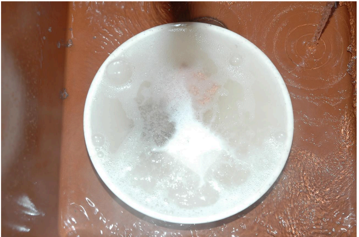
FIG 13. CALCITE BLOCKS QUENCHED IN WATER DEVELOP TYPICAL EFFERVESCENCY. PHOTO BY CELAURO & MAASS
