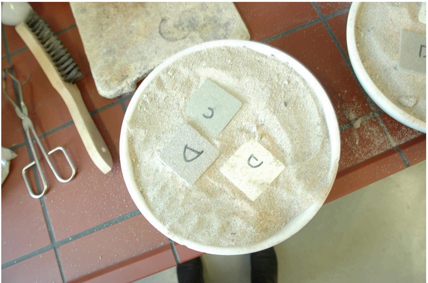
FIG 12A. LOCATION OF BLOCKS IN SAND AND ELECTRIC OVEN USED FOR THE SECOND EXPERIMENTAL TRIAL. PHOTO BY CELAURO & MAASS
