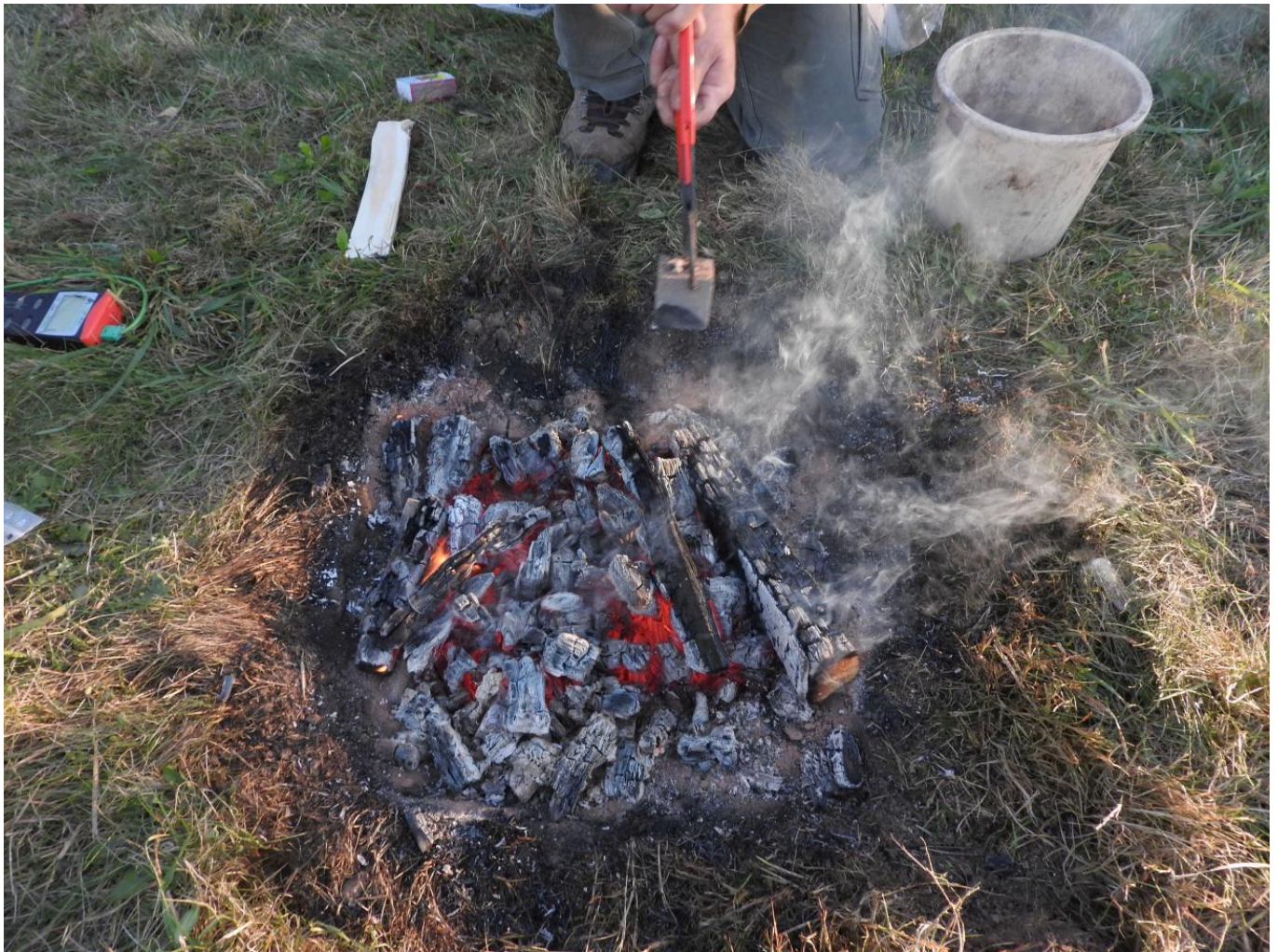
FIG 3C. THE FIRE-SETTING EXPERIMENT WITH NATURAL FIRE AND NATURAL ENVIRONMENT. PHOTO BY CELAURO & MAASS
