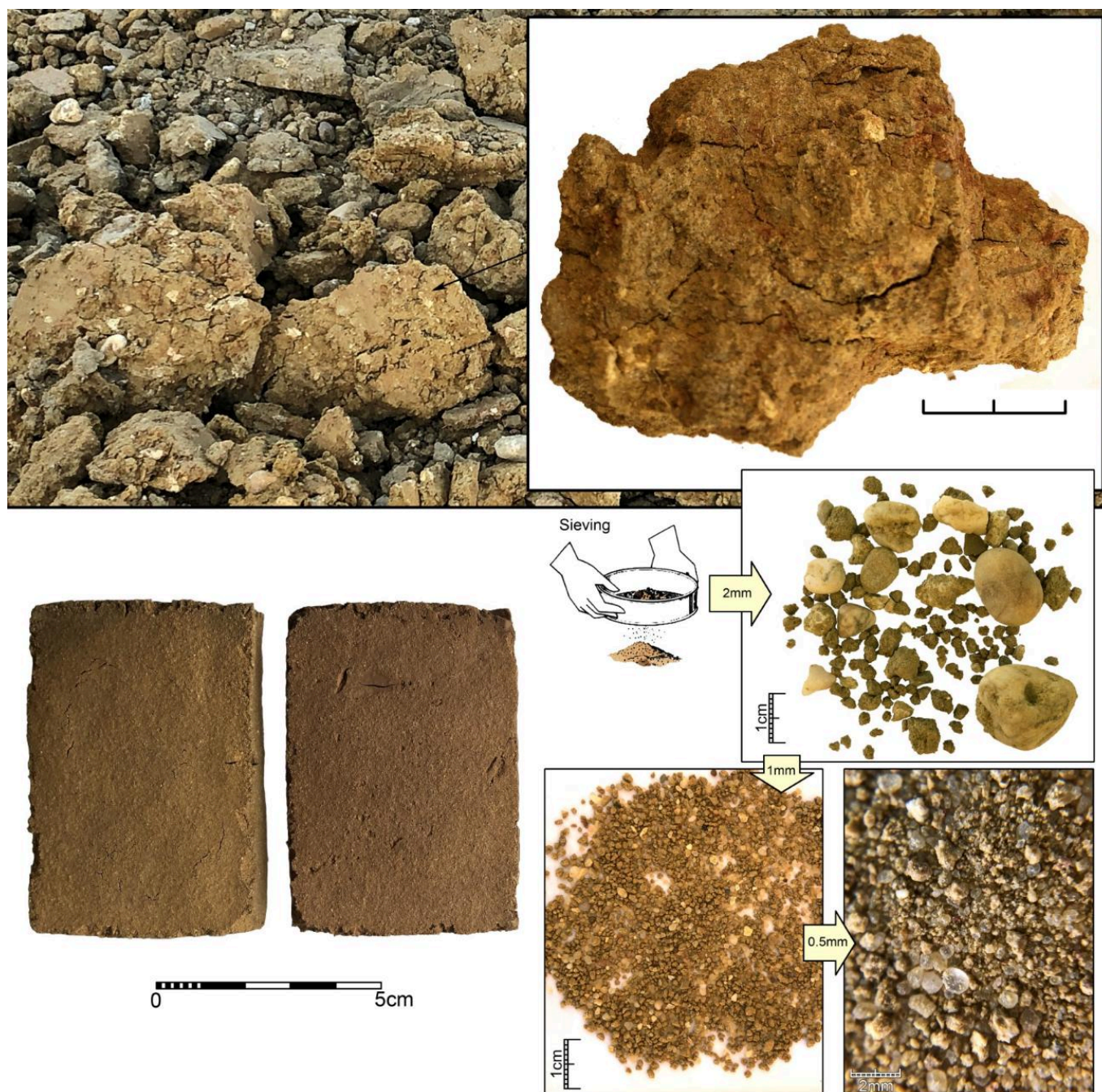
FIG 5. RAW CLAY SAMPLED IN THE VICINITY OF THE PUNIC KILN SITES OF VILLA MARUJA (SAN FERNANDO), SMALL PEBBLES AND QUARTZ SAND ELIMINATED AFTER DRY-SIEVING THE CRUSHED CLAY, AND SMALL BRIQUETTES USED TO TEST THE CONSISTENCY, QUALITY AND SHRINKAGE FACTOR OF THE LOCAL CLAYS THAT WERE USED TO PRODUCE THE T-11213 VESSELS. PHOTOS BY A. SÁEZ
