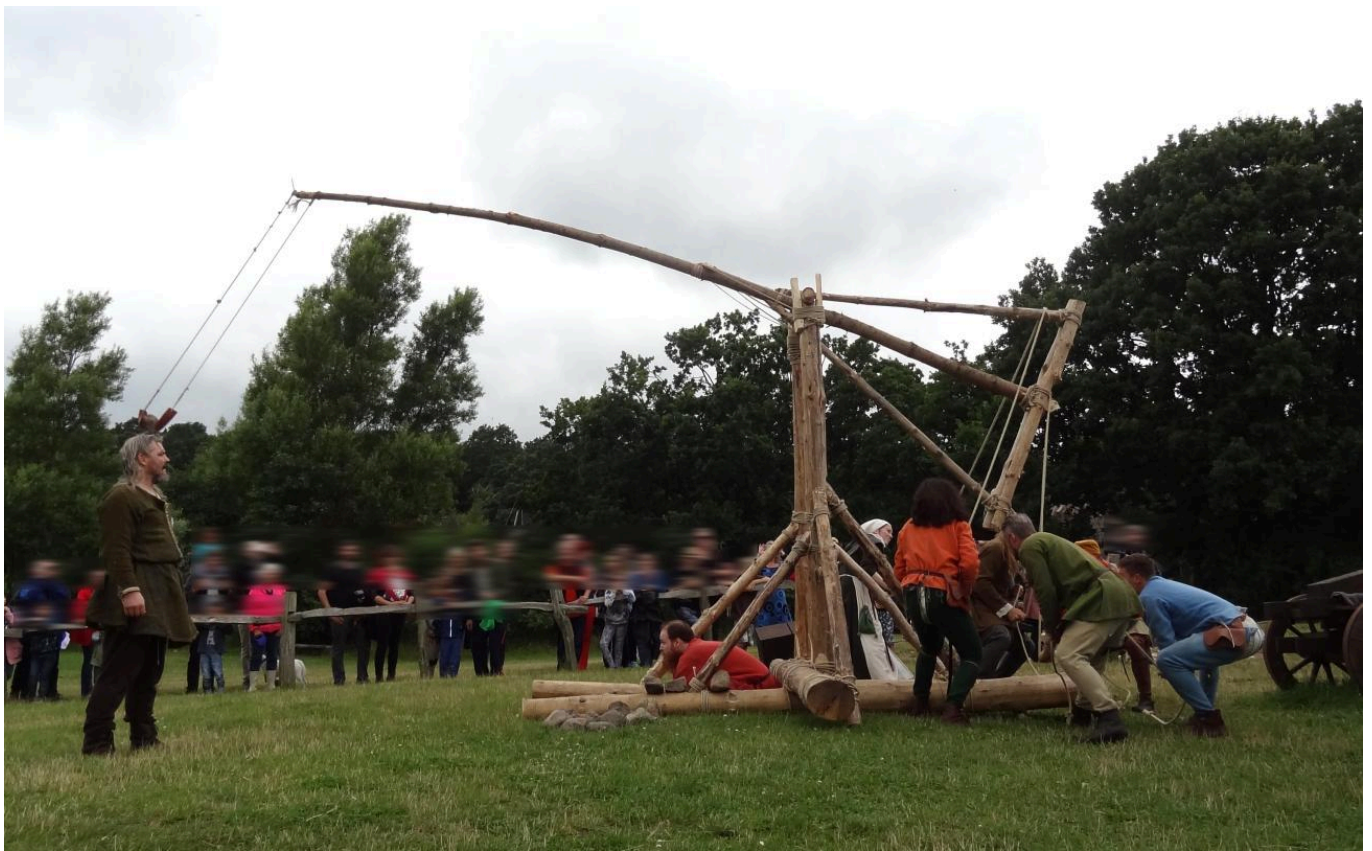
FIG 2. THE TREBUCHET IN ACTION. NOTE THE VERTICAL RELEASE HOOK ON THE END OF THE BENDING ARM, WHERE THE SLING IS ATTACHED. MIDDELALDERCENTERET NYKØBING FALSTER 2017
