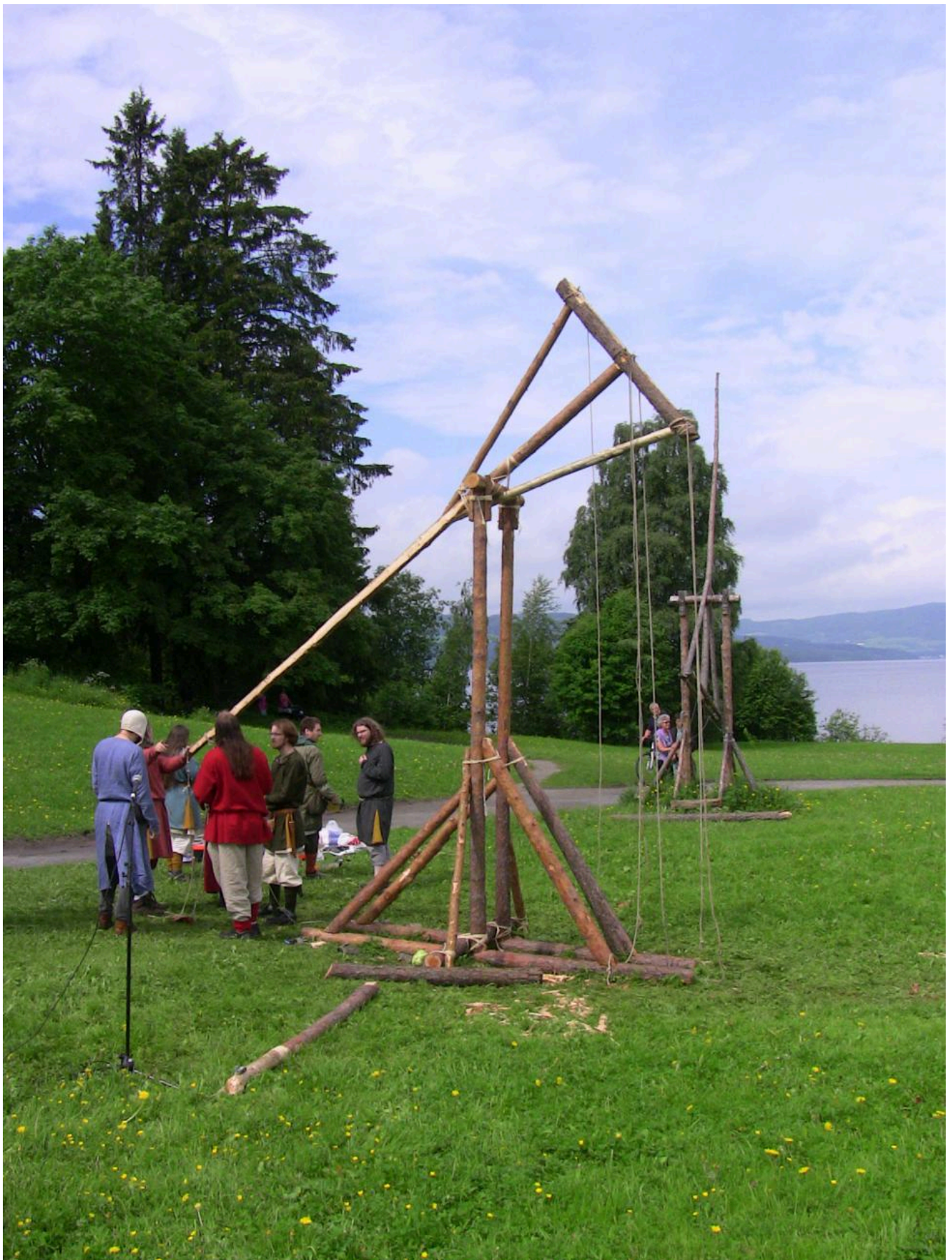
FIG 1. THE TREBUCHET IN THE BACKGROUND IS IN THE RELAXED POSITION WITH THE BRACING CLOSEST TO THE GROUND, THE ONE IN THE FOREGROUND IS BEING HELD DOWN, WITH THE SLING LYING ON THE GROUND. HAMAR MEDIEVAL FESTIVAL 2011
