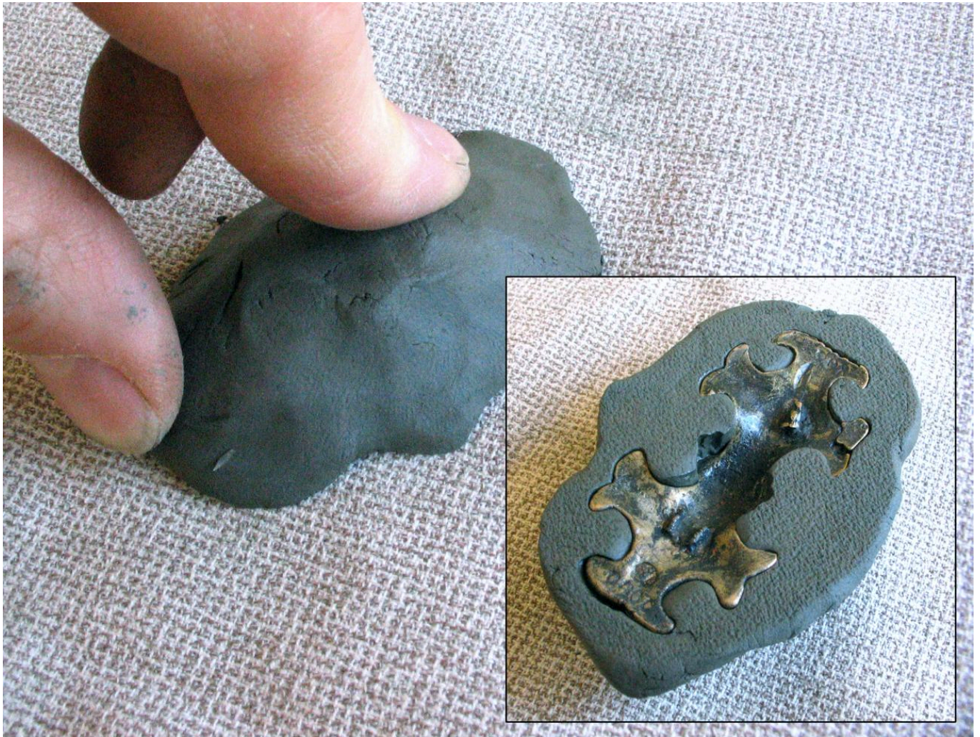
FIG 11. COPYING BY THE WAX COPY METHOD, AS SUGGESTED BY HEDEGAARD, 1992. RAW UNTEMPERED CLAY IS PRESSED ONTO THE METALLIC ORIGINAL MODEL, THAT HAS BEEN PROVIDED WITH A THIN OIL FILM AS A RELEASING AGENT.
