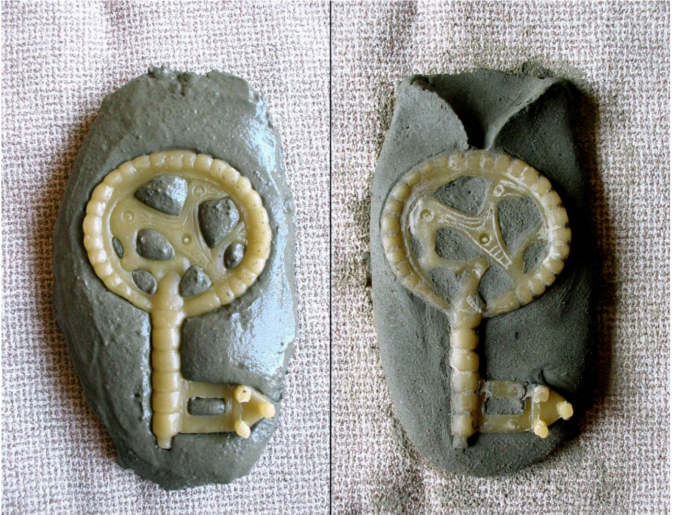
FIG 1. THE WAX MODEL IS PRESSED IN THE TEMPERED CLAY MIX (LEFT), THE SLIGHT GAPS BETWEEN THE MODEL AND THE CLAY THAT OCCURRED ARE CLOSED AND A SPRUE IS MODELLED (RIGHT). THE MOULD IS ALLOWED TO DRY UNTIL IT IS LEATHER HARD BEFORE THE UPPER PART CAN BE MADE.
