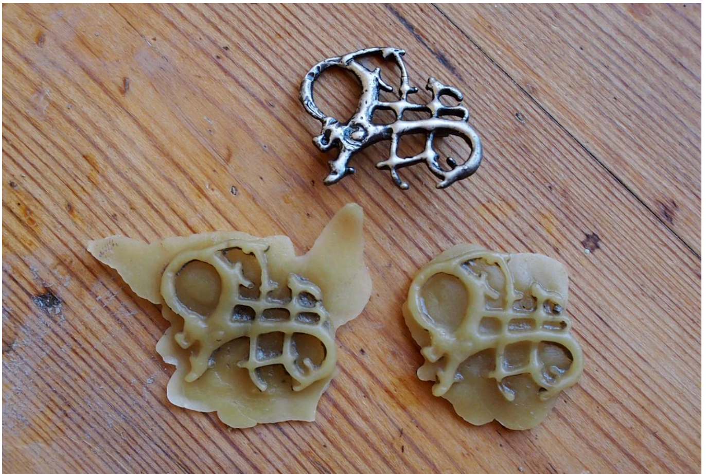
FIG 19. ...THE WAX MODEL IS REMOVED FROM THE CLAY...
