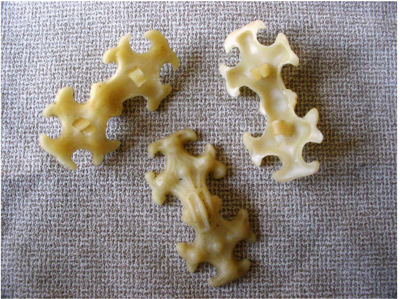
FIG 14. AFTER THE CLAY IS REMOVED FROM THE WAX, WHICH IS EASILY DONE BY PUTTING IT IN A BUCKET OF WATER FOR A WHILE, RETOUCHING THE ORNAMENT DETAILS CAN BE MADE IF NECESSARY. WAX MODELS FOR THE PIN ARRANGEMENT ARE ATTACHED, AND THE MODEL CAN NOW BE USED FOR MAKING MOULDS AS SHOWN IN FIGURES 1& 2.
