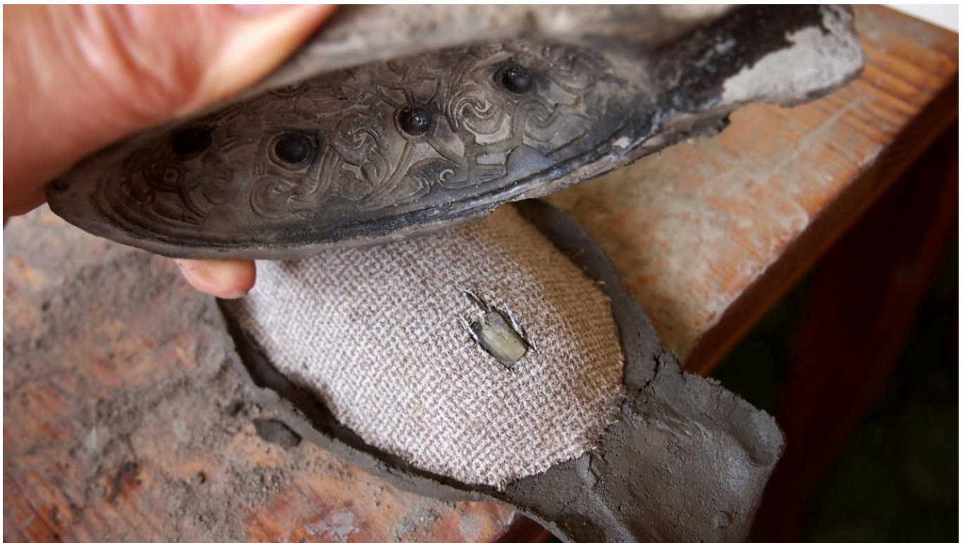
FIG 33. THE CLOTH HAS ATTAINED THE DESIRED SMOOTH CONCAVE-CONVEX SHAPE WHEN PRESSING THE WET CLAY MIX TO IT.
