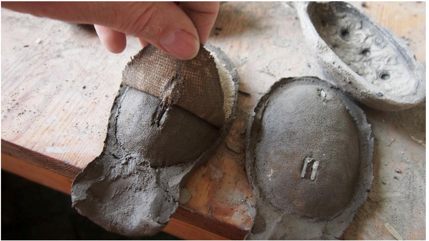
FIG 34. THE CLOTH CAN EASILY BE DETACHED FROM THE MOULD.
