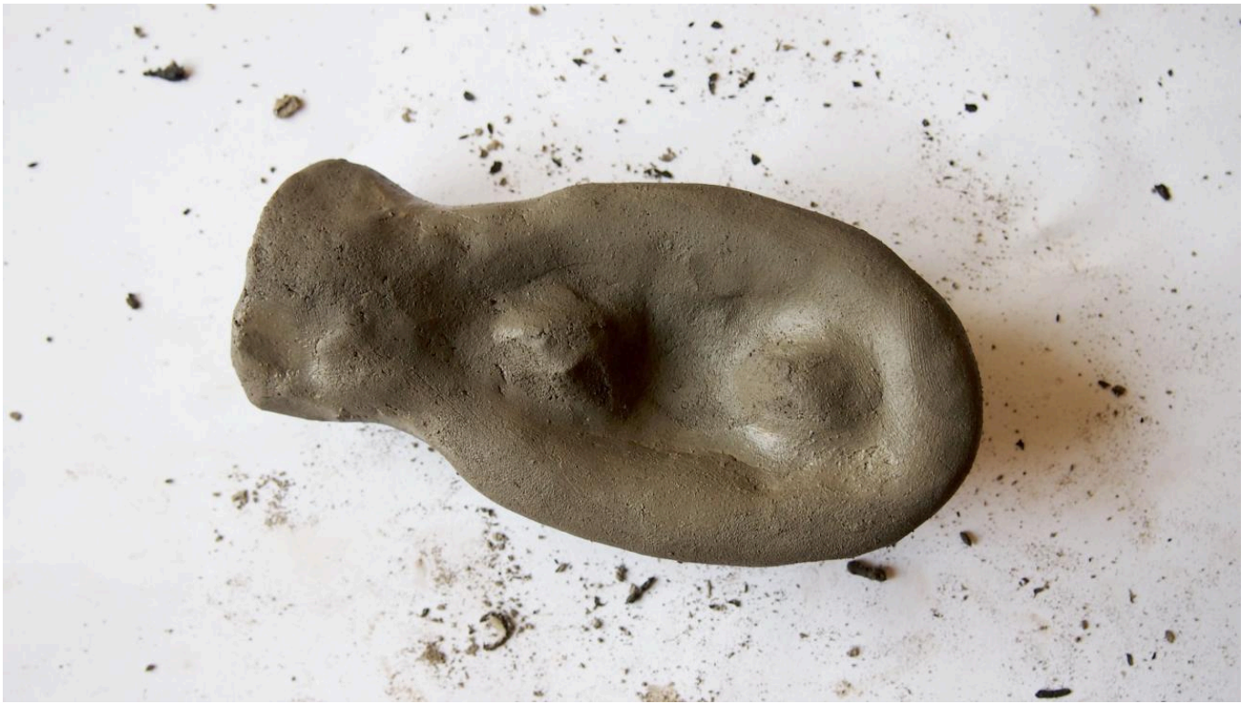
FIG 30. THE MOULD IS NOW FINISHED AND LEFT TO DRY. AS THE FRONT PART ALREADY WAS DRY WHEN THE REVERSE PART WAS MADE, THE LATTER WILL SHRINK AND CRACK DURING DRYING. THOSE FRACTURES MUST BE TAKEN CARE OF AND MENDED AS THEY APPEAR, THROUGHOUT THE REMAINING DRYING PROCESS.
