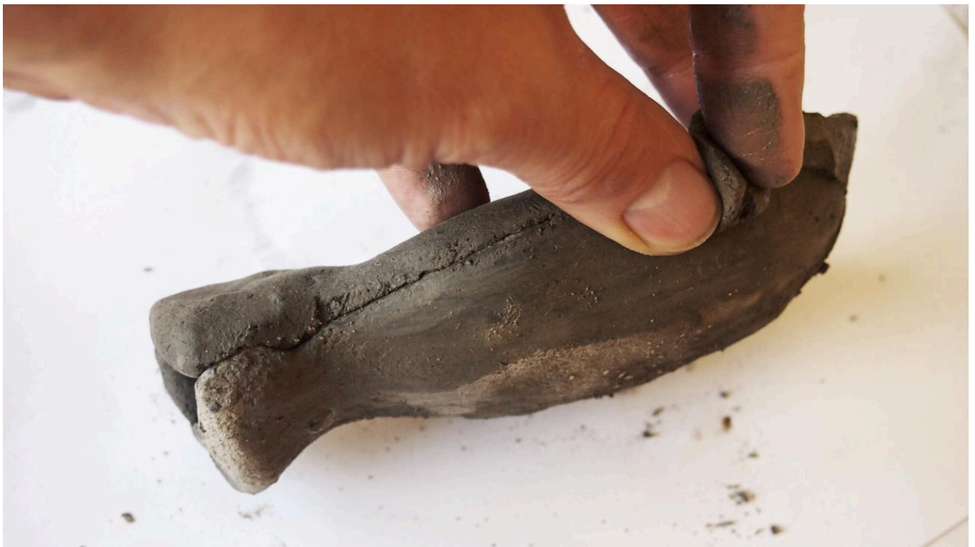
FIG 29. AFTER SLIGHT DRYING, THE MOULD CAN BE OPENED AFTER HEATING AND THE CLOTH CAN BE BROUGHT OUT OF IT. AFTER THIS, THE MOULD IS PUT TOGETHER AGAIN, AND THE JOINT IS SEALED WITH CLAY MIX.
