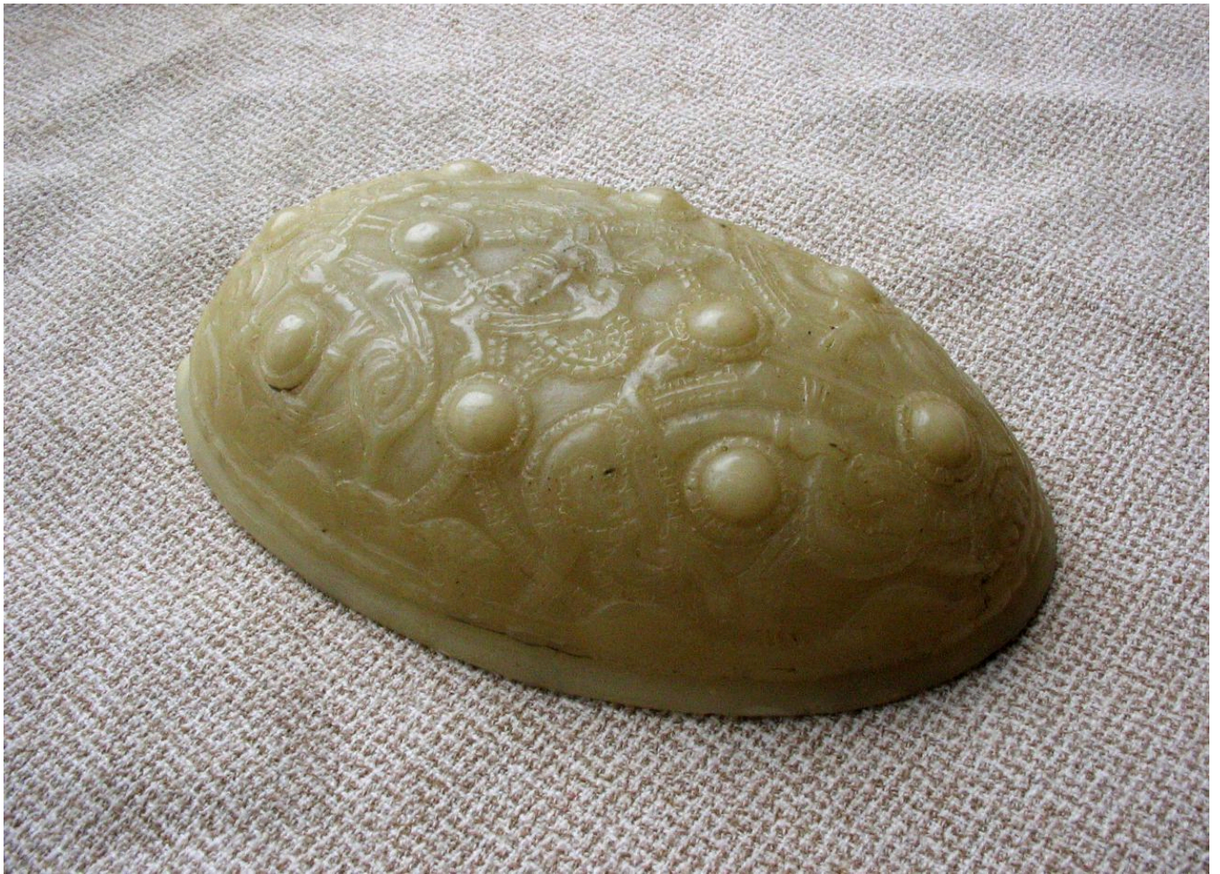
FIG 24. A WAX MODEL OF AN OVAL BROOCH OF THE P 27 TYPE, MADE WITH THE WAX COPY METHOD. THE PICTURE SHOWS THE ASTONISHINGLY GOOD TRANSFER OF DETAILS THAT YOU ATTAIN WITH THIS SIMPLE METHOD.
