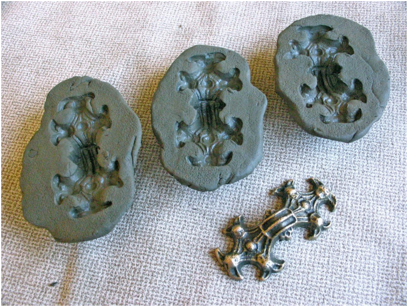
FIG 12. THE ORIGINAL MODEL IS REMOVED FROM THE CLAY, LEAVING A NEGATIVE IMPRINT.
