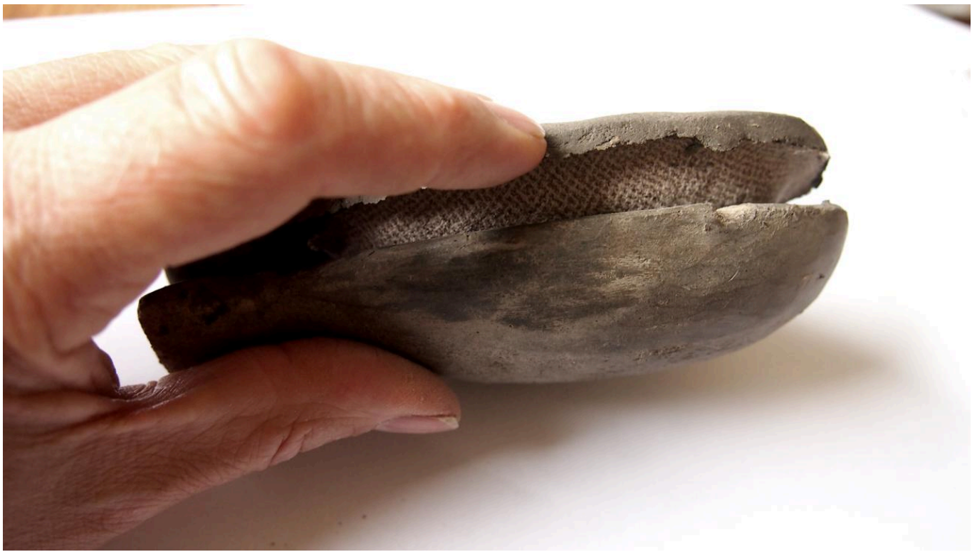
FIG 32. AFTER SLIGHT DRYING, THE MOULD CAN EASILY BE OPENED.
