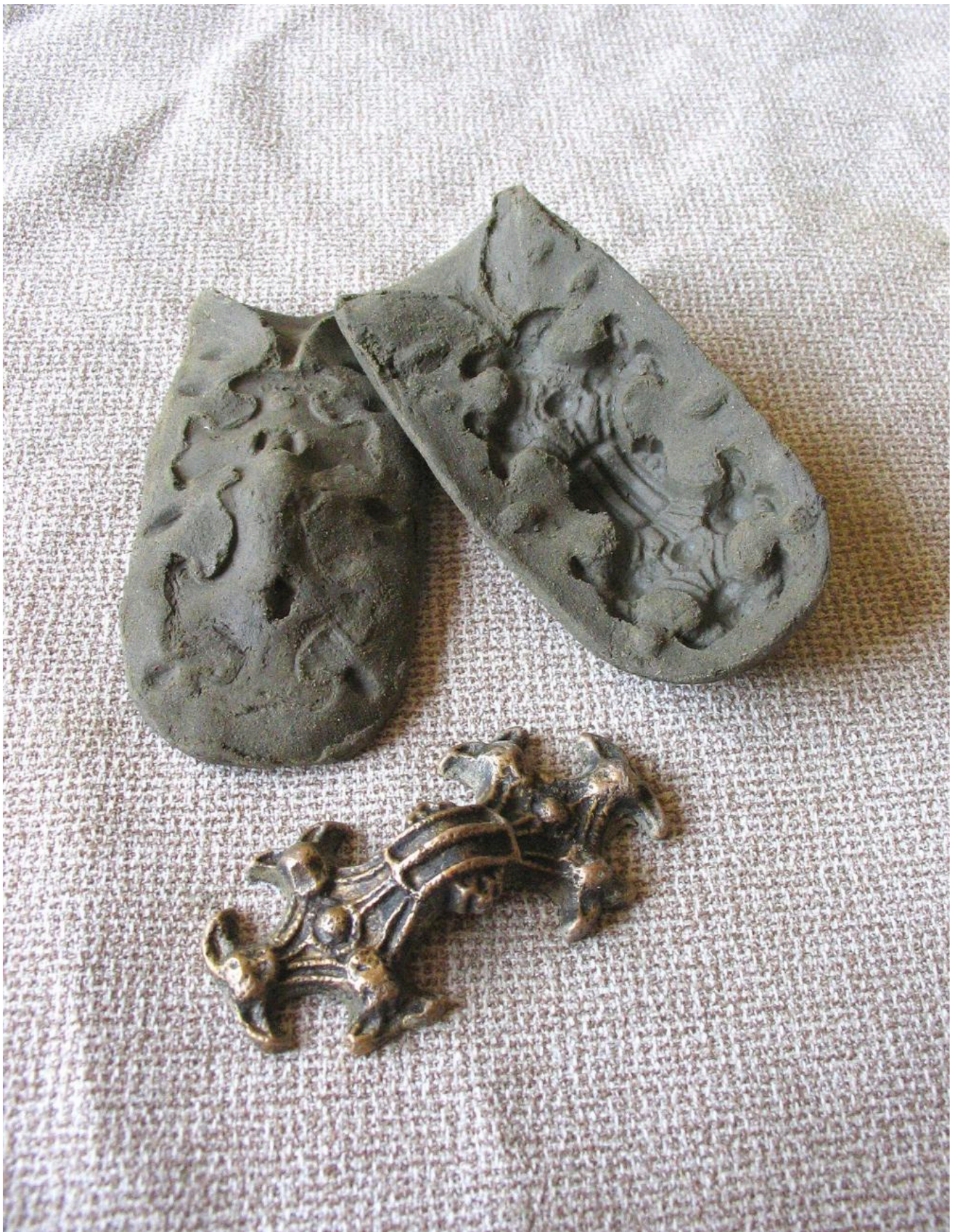
FIG 6. AFTER THE UPPER PART IS STABLE BUT NOT YET DRY, THE MOULD CAN BE OPENED AND THE MODEL CAN BE DETACHED FROM IT. AFTER THIS, THE TWO PARTS ARE JOINED TOGETHER AGAIN, AND THE MOULD IS CLOSED AT THE JOINS WITH A LAYER OF CLAY MIX.
