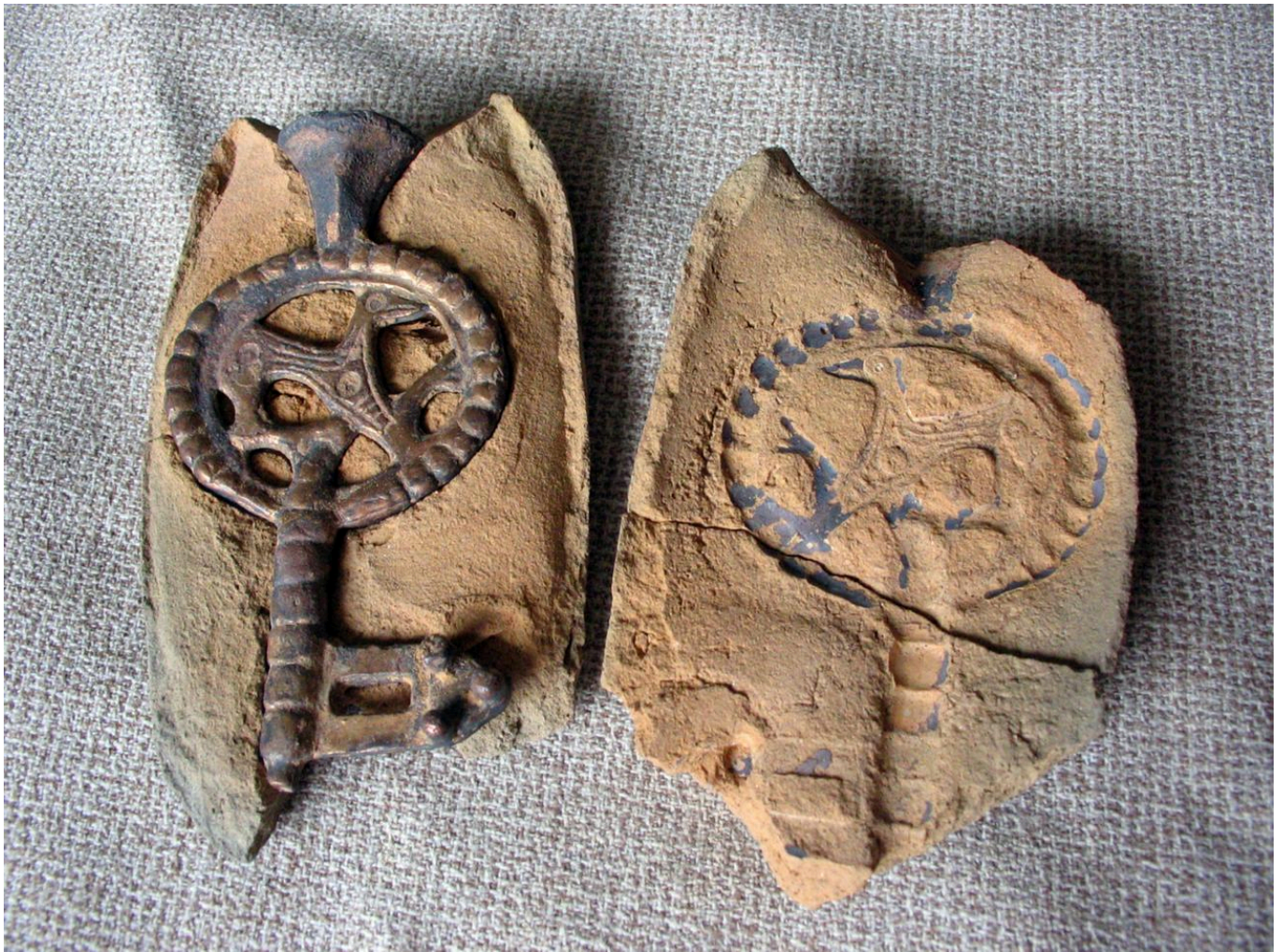
FIG 3. AFTER POURING THE METAL, THE MOULD IS OPENED. IT WILL SPLIT INTO TWO HALVES SPONTANEOUSLY.
