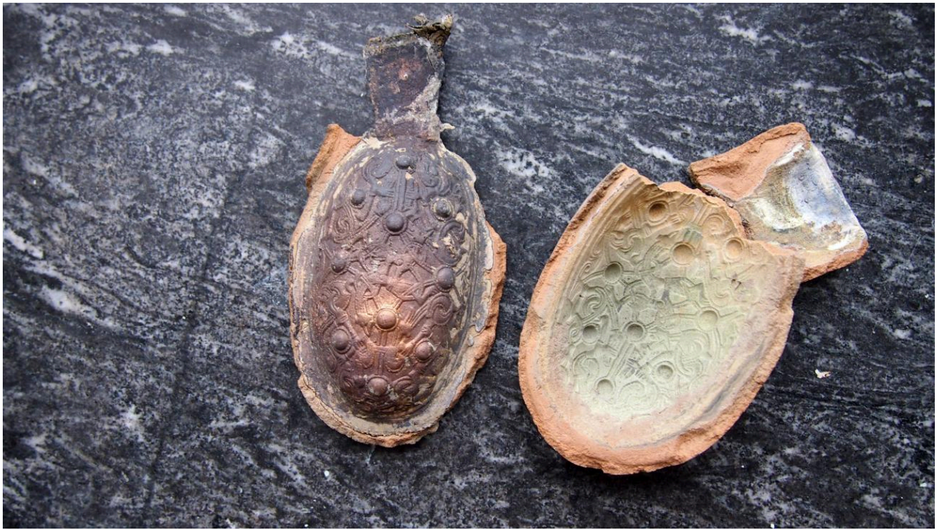
FIG 38. THE CAST RESULT. THERE IS A SLIGHT FINISHING WORK TO DO, LIKE FILING THE FLASHES AWAY FROM THE EDGES. THE MARK OF A GOOD CASTING IS WHEN YOU GET A MINIMUM OF THE NEED FOR RETOUCHING THE ORNAMENTS AFTER CASTING. IN THIS CASE, EVERYTHING THAT WAS SUPPOSED TO BE THERE IS THERE, AND IT WAS THERE ALREADY IN THE MORE EASILY WORKED WAX MODEL. THE BROOCH NEEDS NO MORE FINISHING WORK BUT FILING THE EDGES AND POLISHING.
