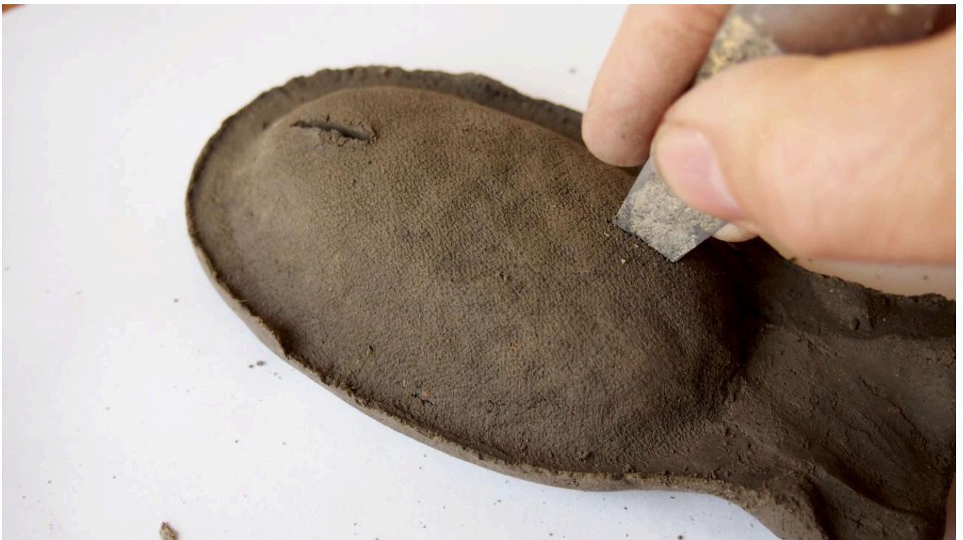
FIG 35. AN ALTERNATIVE WAY OF CREATING THE ARRANGEMENTS FOR THE PIN, BY SIMPLY CUTTING THEM WITH A KNIFE IN THE STILL SLIGHTLY WET CLAY.
