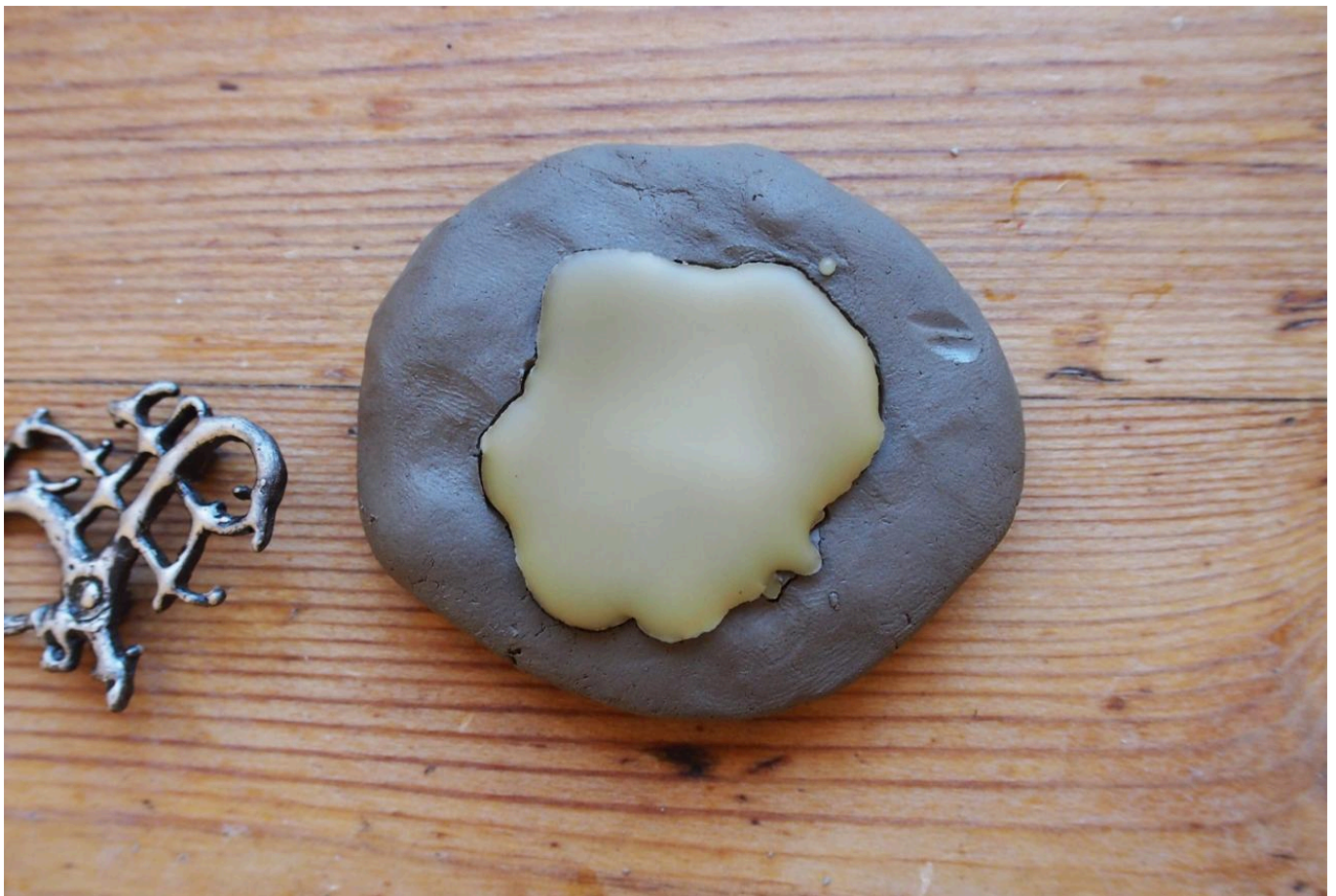
FIG 18. ...WAX IS POURED INTO THE NEGATIVE IMPRINT...
