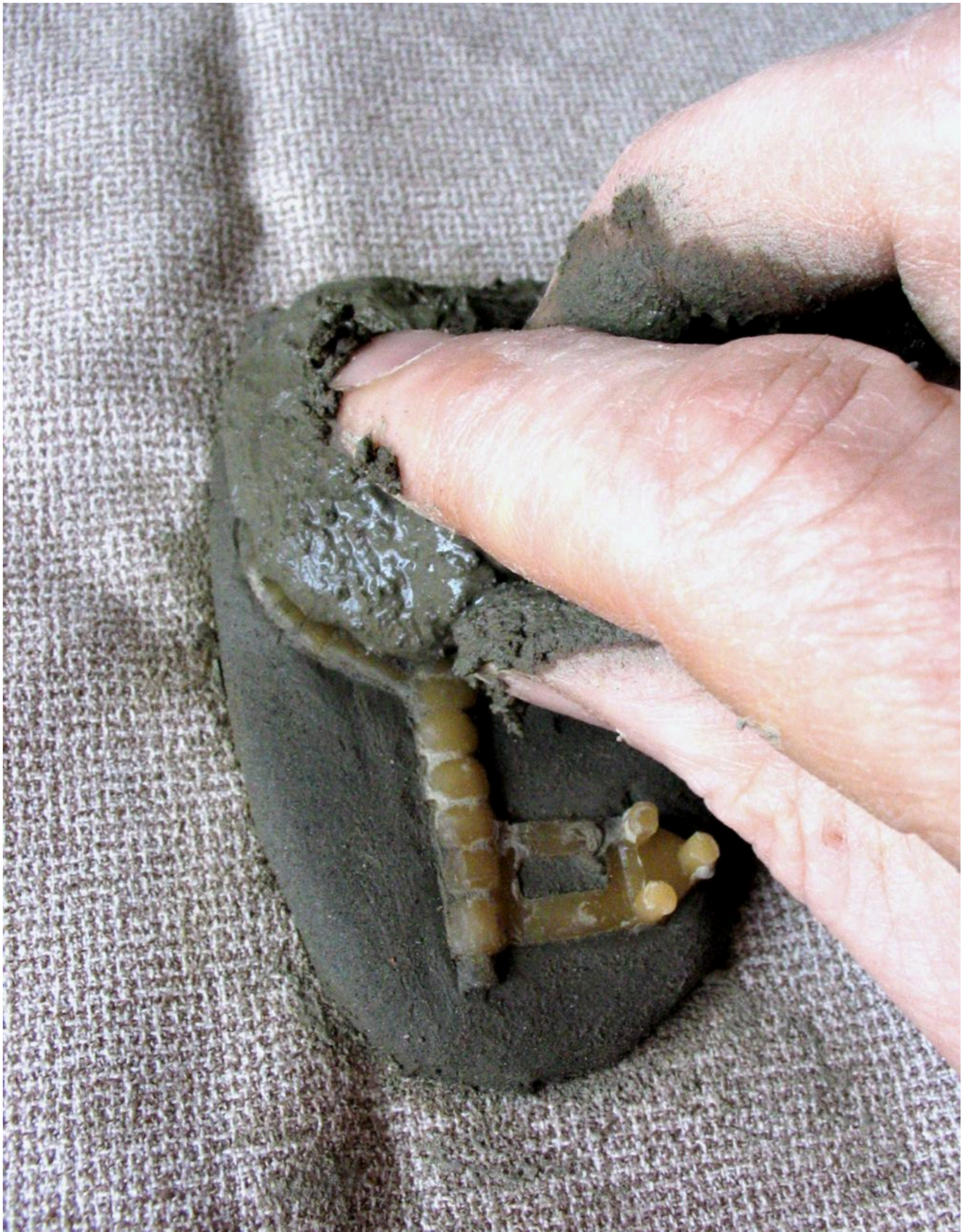
FIG 2. WHEN THE UNDER HALF OF THE MOULD IS STABLE, THE UPPER PART CAN BE MODELLED OVER IT. THE MOULD IS CLOSED AT THE JOINT BY FOLDING THE EDGES OF THE UPPER PART OVER. AFTER THIS, THE MOULD IS DRIED, THE WAX IS MELTED OUT FROM IT AND IT IS FIRED AND TURNED INTO CERAMIC MATERIAL.
