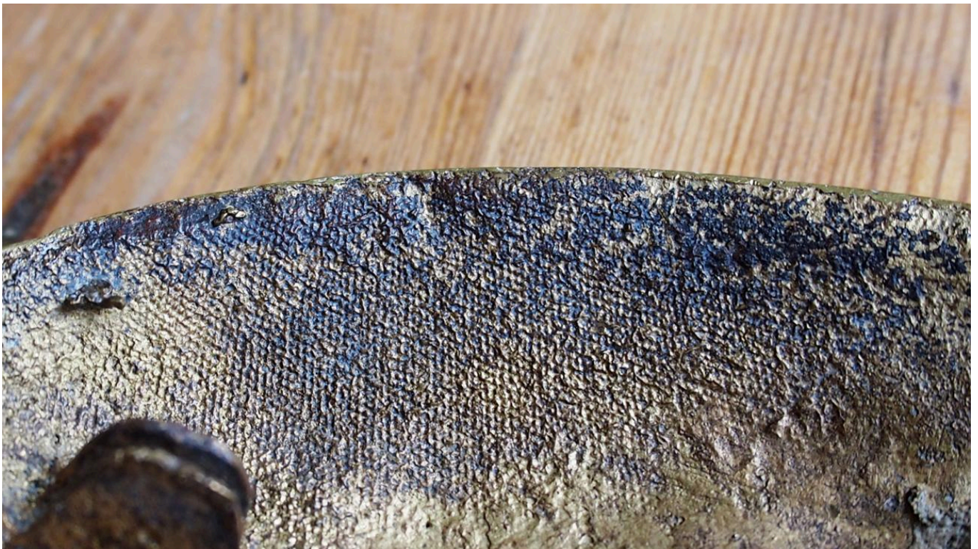
FIG 41. THE TEXTILE PATTERN ON THE REVERSE OF A BROOCH CAST BY THE SECOND SUGGESTED WAX COPY METHOD, WHERE THE CLOTH WAS USED TO REINFORCE A VERY THIN WAX MODEL. THE CLOTH WAS A VERY FINE LINEN TABBY.
