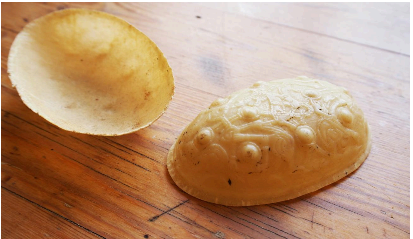
FIG 37. AN EXTREMELY THIN WAX MODEL WHERE THE CLOTH IS USED AS REINFORCEMENT, WITH THE DESIRED THICKNESS OF THE FINAL PRODUCT. THE REGISTRATION OF THE ORNAMENTS IS JUST AS GOOD AS WHEN USING THE ABOVE-SUGGESTED METHOD FOR WAX COPYING SOLID MODELS (CF. FIGURE 24).
