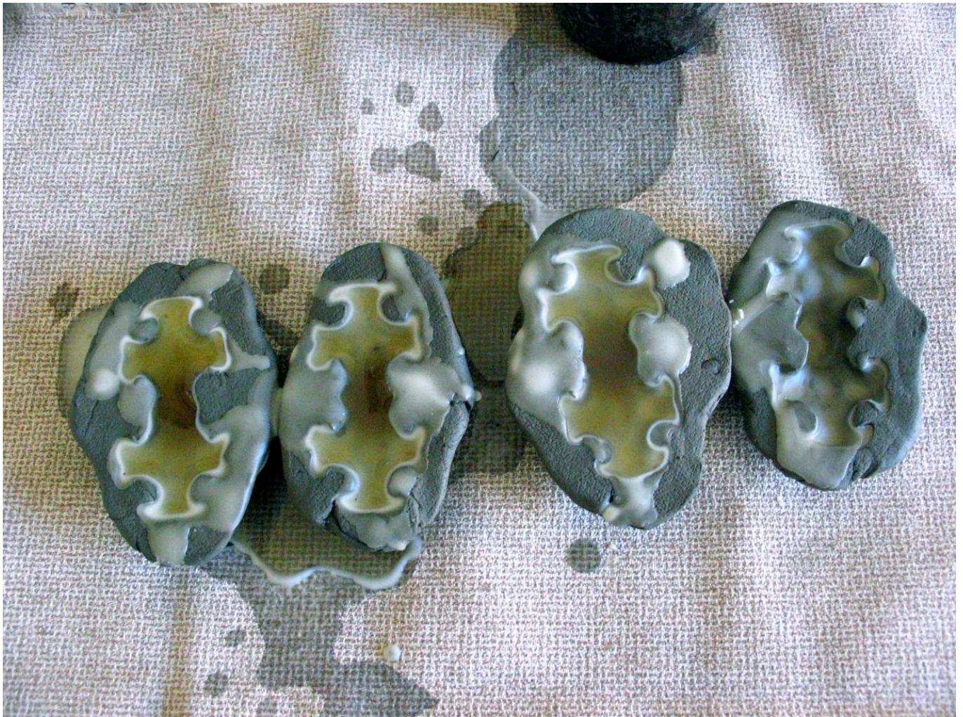
FIG 13. THE IMPRINT IS FILLED WITH WAX. AFTER THE WAX HAS SOLIDIFIED NEXT TO THE IMPRINT – WHICH HAPPENS FAST, AS THE WET CLAY IS COLD – SURPLUS WAX CAN BE POURED OUT LIKE IN THE RIGHT IMPRINT SO THAT THE MODEL WILL BE THIN, IN THIS WAY MAKING THE MATERIAL AS THIN AS POSSIBLE IN THE CAST PRODUCT (CF. FIGURE 15 AND 23, RIGHT).
