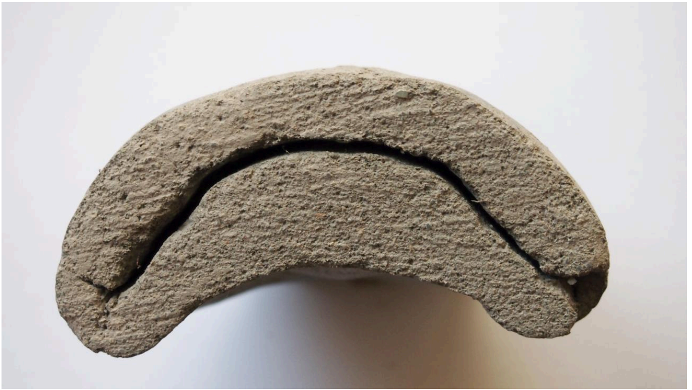
FIG 36. A CROSS-SECTION OF AN UNFIRED MOULD MADE WITH A PIECE CLOTH THAT HAS NOT BEEN SOAKED WITH WAX. AS THE MOULD SHRINKS THE CAVITY WILL WIDEN UP A LITTLE AND THE THICKNESS OF THE GOODS IN THE FINAL BROOCH WILL NOT BE AS THIN AS THE TEXTILE. IN THIS CASE, THE MOULD WAS PROBABLY OPENED FOR DETACHING THE CLOTH WHEN IT WAS STILL TOO WET. THE DRYING SHRINKAGE MADE THE CAVITY A BIT TOO WIDE, UP TO TWO MILLIMETRES. THE OVAL BROOCHES WERE USUALLY INCREDIBLY THIN.
