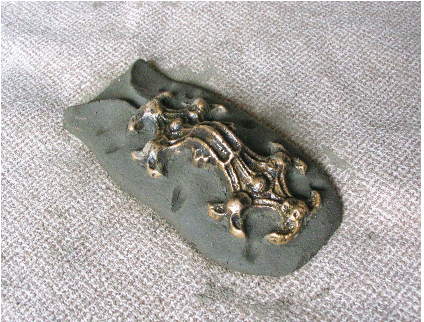
FIG 5. MAKING A MOULD WITH A MODEL OF A SOLID MATERIAL, WITHOUT THE USE OF WAX. THE MODEL IS PRESSED IN CLAY MIX, THE SURFACES ARE SMOOTHED, AND A NUMBER OF KEY HOLES ARE PRESSED IN IT. AFTER DRYING FOR HALF AN HOUR, UNTIL THE CLAY IS STABLE, THE UPPER PART CAN BE MADE AFTER APPLYING A RELEASING AGENT ON THE UNDER PART. THIS AGENT COULD BE FAT OR SOAP.
