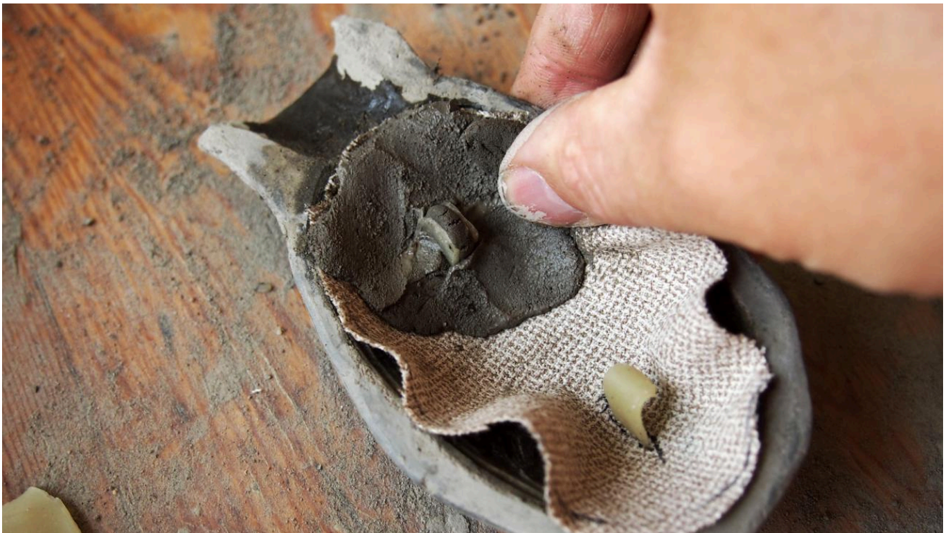
FIG 31. AN ALTERNATIVE METHOD, USING A PIECE OF CLOTH THAT HAS NOT BEEN WAXED.
