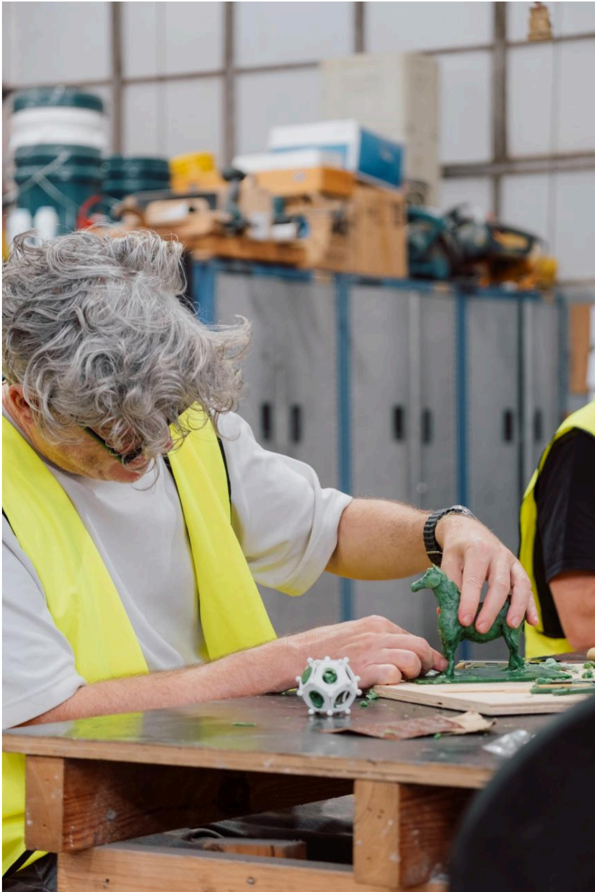
FIG 13. WAX-HANDLING WORKSHOP DURING PRELIMINARY FORMING TRIALS. PRELIMINARY HANDLING TESTS EXPLORED HOW SOFTENED WAX BEHAVED UNDER PRESSURE AND HOW IT COULD BE SHAPED WITHOUT POURING.
