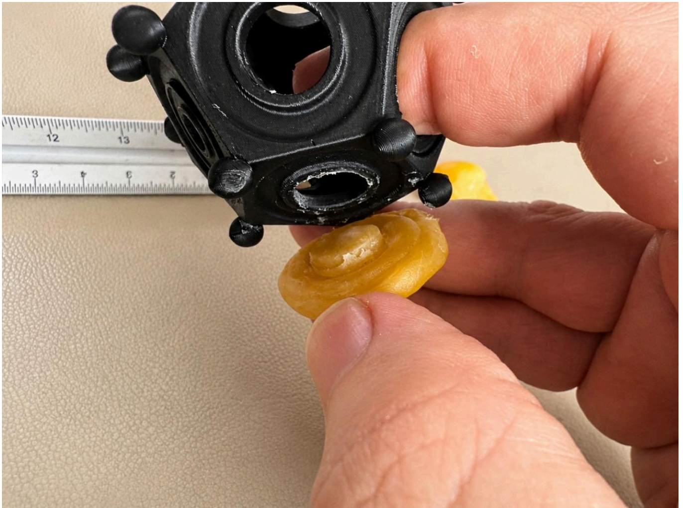
FIG 8B. REMOVAL OF THE FORMED WAX BULLA FROM THE DODECAHEDRON. THE WAX WAS RELEASED BY MANIPULATING IT THROUGH THE LARGER APERTURE RATHER THAN PULLING IT FROM THE EXTERIOR. THIS HANDLING METHOD HELPED PRESERVE THE RAISED BOSS AND SURROUNDING FORMED SURFACE.
