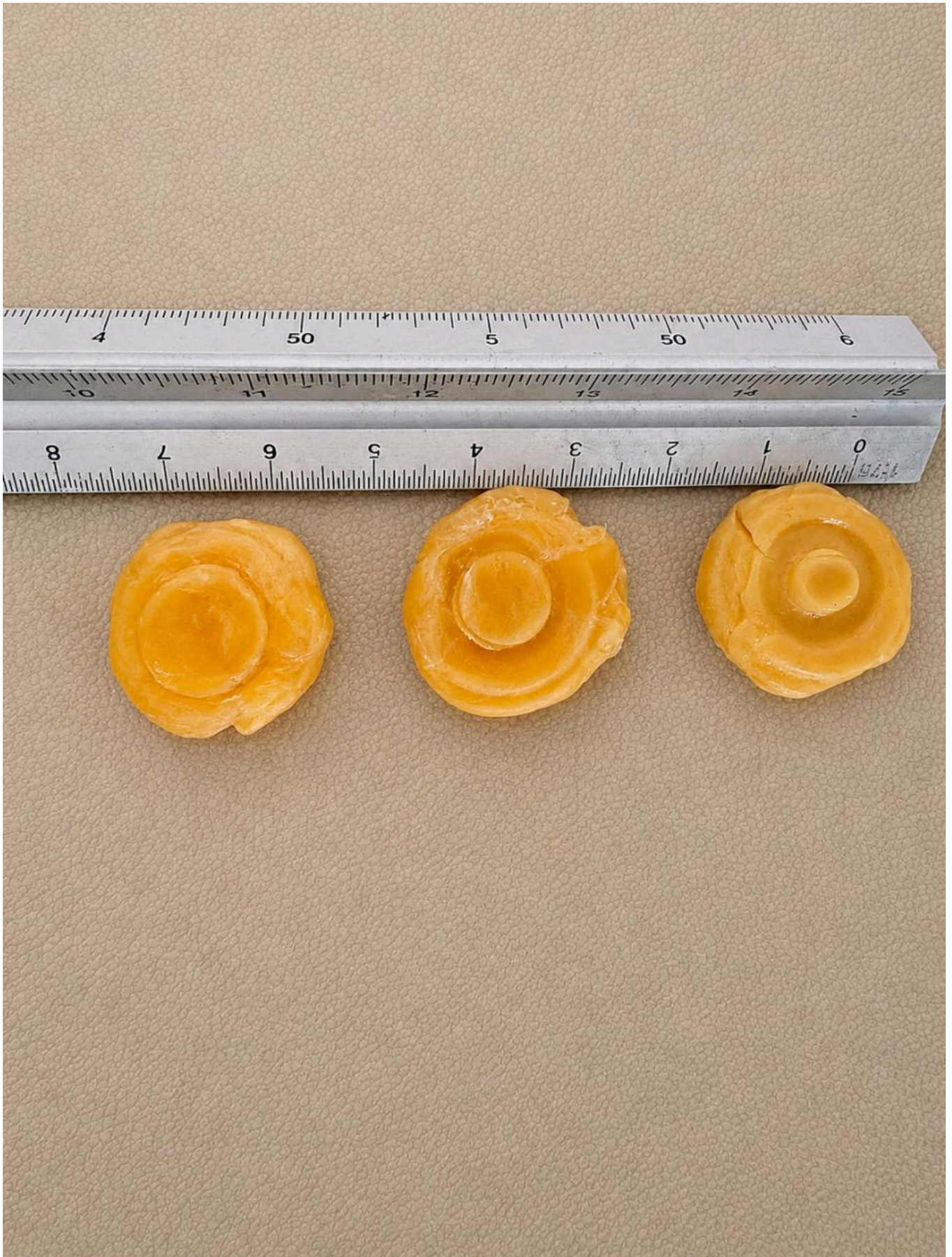
FIG 4. COMPARISON OF WAX BULLAE FORMED WITH AND WITHOUT A RELEASE AGENT. THE EXAMPLES SHOW THE EFFECT OF SURFACE PREPARATION DURING REMOVAL FROM THE DODECAHEDRON. A VERY THIN FILM OF OLIVE OIL REDUCED ADHESION AND ALLOWED THE FORMED WAX TO RELEASE MORE CLEANLY, SUGGESTING THAT THE DIFFICULTIES OBSERVED WITH PLA REPLICAS WERE PARTLY RELATED TO SURFACE TEXTURE RATHER THAN THE FORMING GEOMETRY ITSELF.
