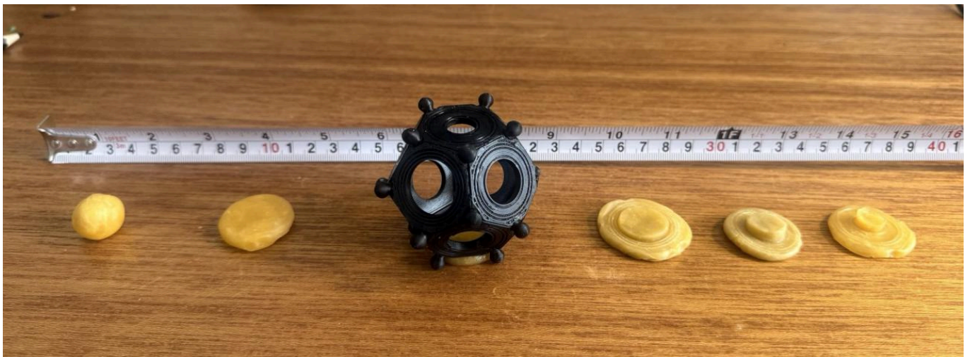
FIG 9. KNOB-CONTROLLED THICKNESS IN REPEATED WAX-FORMING TRIALS. FROM LEFT TO RIGHT: AN UNFORMED WAX BALL, A FLATTENED DISC, WAX COMPRESSED USING THE DODECAHEDRON, AND FINISHED WAX FORMS PRODUCED USING DIFFERENT APERTURES. THE CONSISTENT PERIMETER THICKNESS SUGGESTS THAT THE PROTRUDING KNOBS ACTED AS PASSIVE DEPTH STOPS DURING COMPRESSION.
