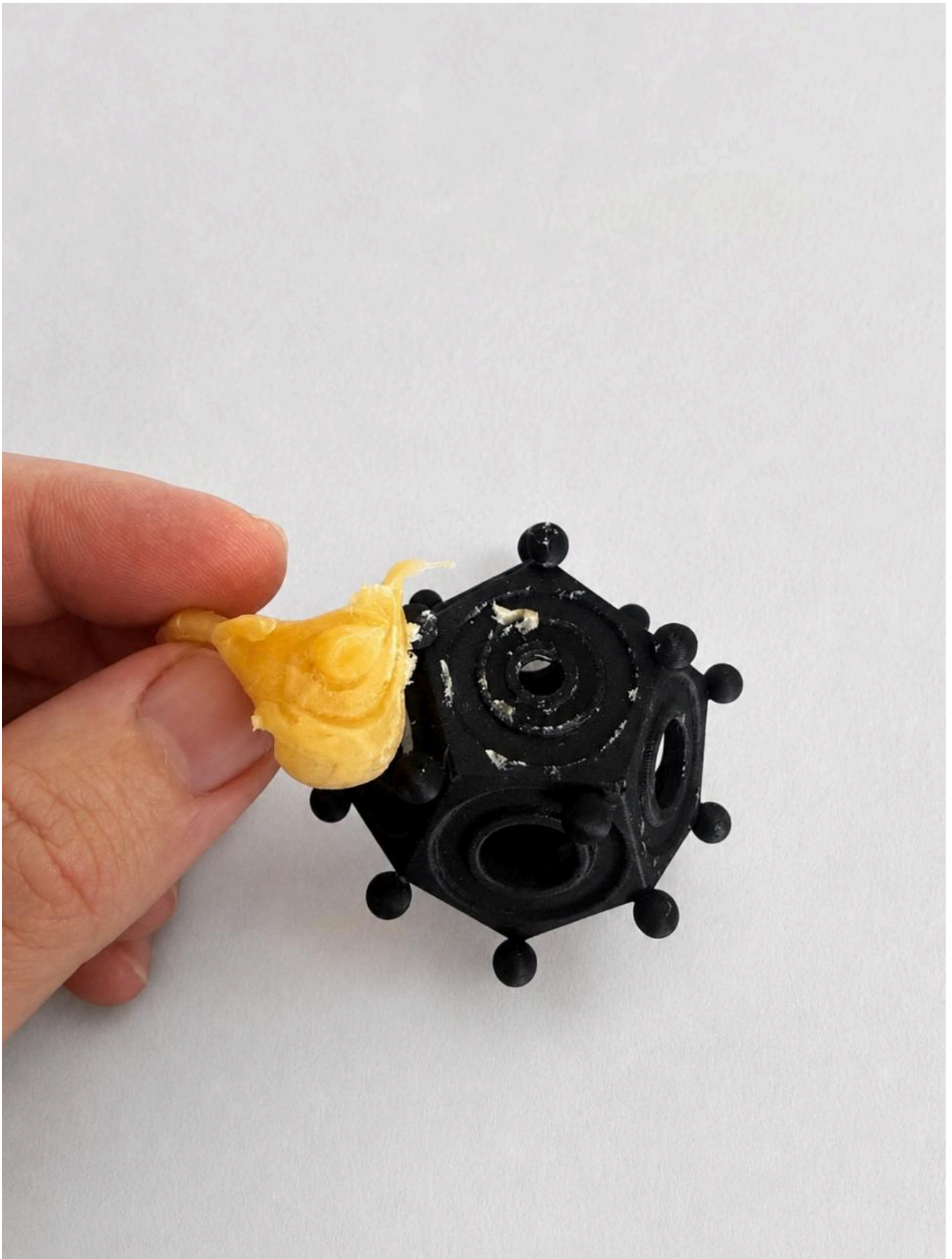
FIG 3. FAILED WAX BULLA CAUSED BY ADHESION DURING REMOVAL. IN EARLY TRIALS, SOFTENED WAX ADHERED TO THE TEXTURED SURFACE OF THE 3D-PRINTED REPLICA, PARTICULARLY WHEN PRESSED THROUGH SMALLER APERTURES. REMOVAL OFTEN DISTORTED OR TORE THE WAX, DEMONSTRATING THAT RELEASE BEHAVIOUR WAS A CRITICAL FACTOR IN ASSESSING THE TOOL'S FUNCTIONAL PLAUSIBILITY.
