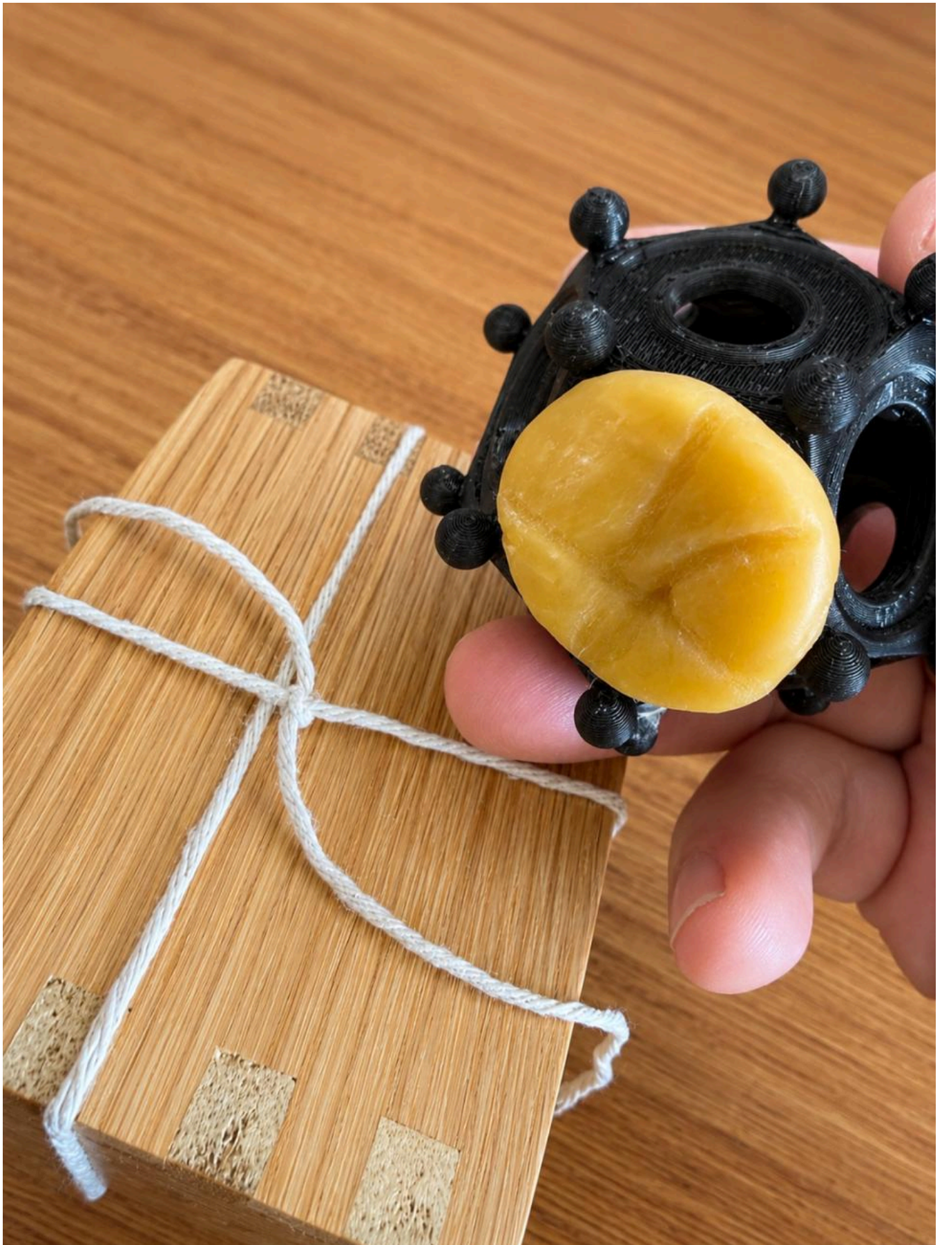
FIG 5. EARLY DOCUMENT-SEALING TRIAL USING A SINGLE MASS OF WAX. WAX WAS PRESSED DIRECTLY OVER CORD TO EMULATE THE FUNCTION OF A ROMAN SEAL BOX OR CORD-SECURED DOCUMENT SEAL. ALTHOUGH A VISUALLY PLAUSIBLE BULLA COULD BE PRODUCED, THE CORD WAS NOT RELIABLY ENCLOSED. WHEN THE WAX DETACHED, THE STRING COULD BECOME EXPOSED, INDICATING THAT A MORE SECURE FORMING METHOD WAS REQUIRED.
