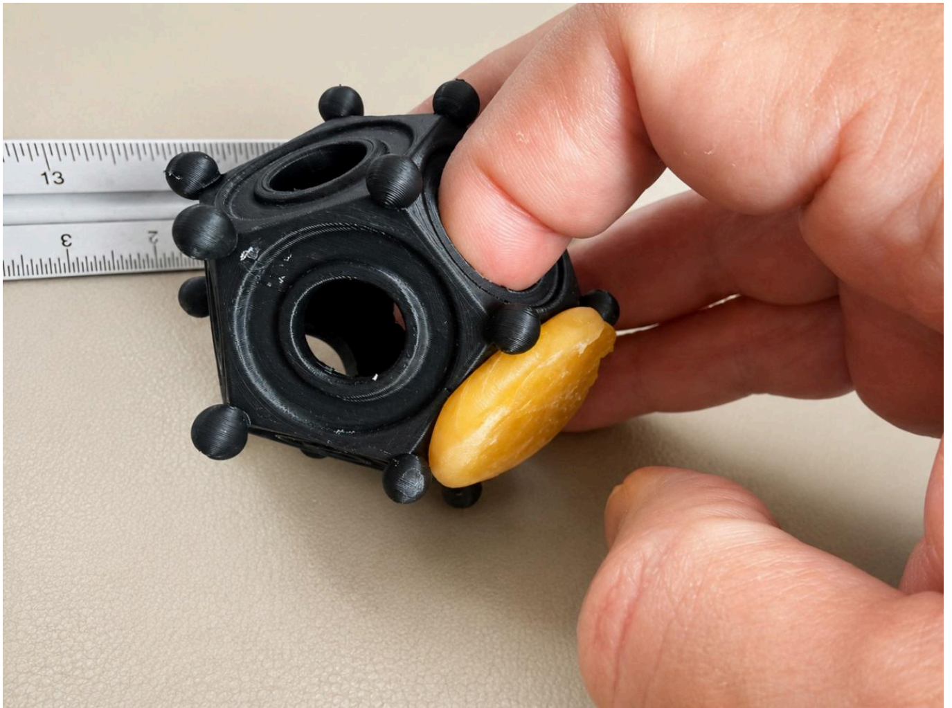
FIG 8A. FINGER ACCESS THROUGH THE LARGER APERTURE DURING REMOVAL. THE LARGER APERTURES ALLOWED A FINGER TO ENTER THE HOLLOW BODY OF THE DODECAHEDRON AND GENTLY PUSH THE WAX AWAY FROM THE TOOL. THIS REDUCED DISTORTION DURING RELEASE AND SUGGESTS A PRACTICAL ROLE FOR THE LARGEST OPENINGS BEYOND SIMPLE VARIATION IN APERTURE SIZE.
