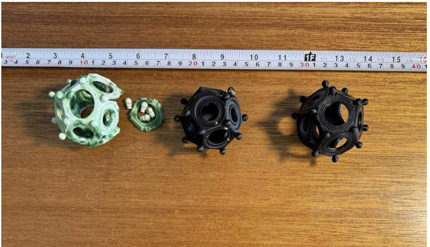
FIG 1. 3D-PRINTED DODECAHEDRON REPLICAS USED IN THE EXPERIMENTAL TRIALS. FROM LEFT TO RIGHT: THE INITIAL PRINT, AN ALTERNATIVE SINGLE-PIECE PRINT, AND THE FINAL MECHANICALLY STABLE PRINT USED FOR THE MAIN FORMING TRIALS. EARLIER PRINTS WERE USEFUL FOR EXPLORING HANDLING, ADHESION, AND FAILURE MODES, WHILE THE FINAL REPLICA PRESERVED THE KEY FUNCTIONAL FEATURES REQUIRED FOR TESTING: HOLLOW CONSTRUCTION, VARIABLE APERTURES, AND PROTRUDING CORNER KNOBS.
