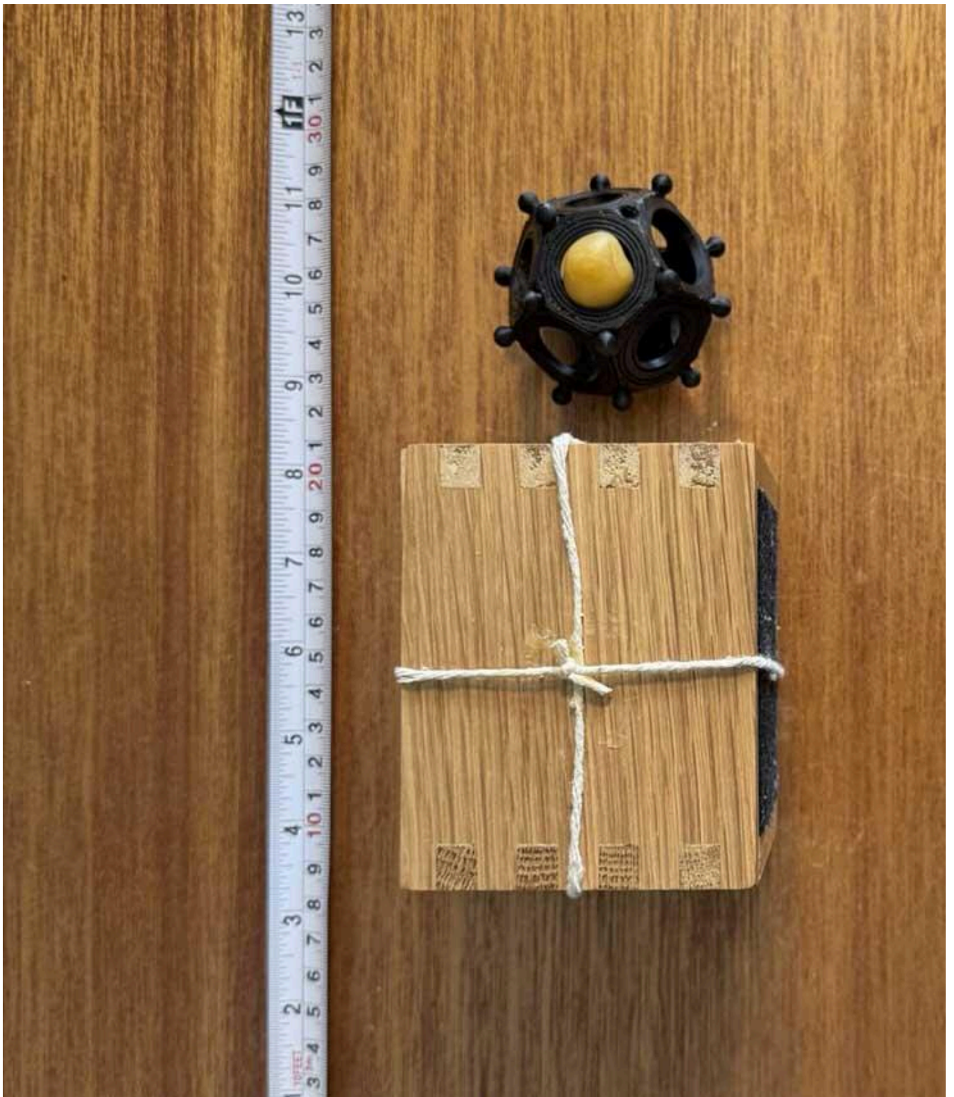
FIG 6A. INITIAL WAX BALL PREPARED FOR THE REVISED TWO-PART METHOD. A WAX BALL WAS FORMED BY HAND AND SIZED VISUALLY AGAINST THE LARGER APERTURE OF THE DODECAHEDRON. THIS PROVIDED A QUICK PRACTICAL GAUGE FOR ESTIMATING THE AMOUNT OF WAX REQUIRED BEFORE DIVIDING IT INTO TWO PARTS.
