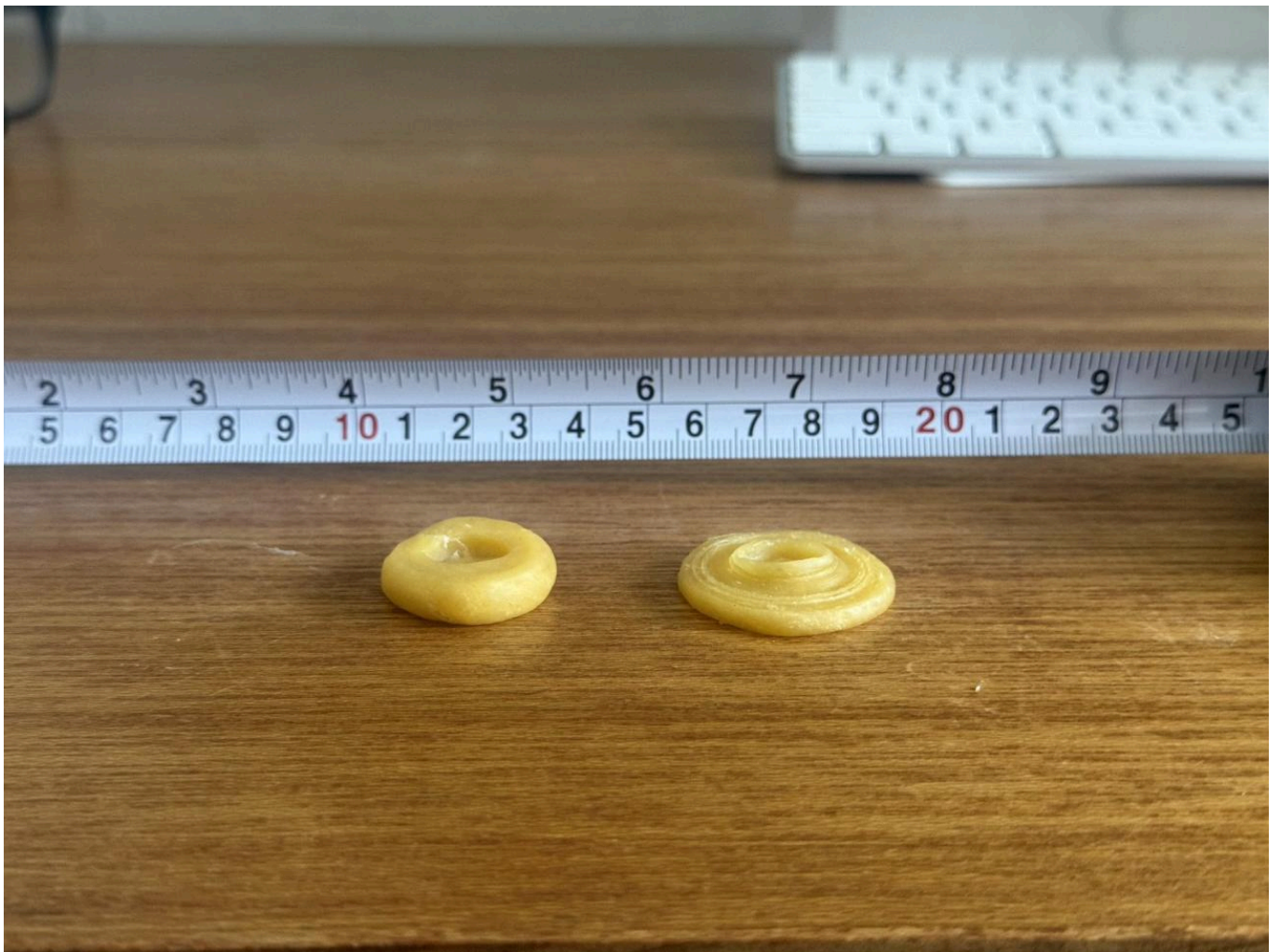
FIG 10A. SIDE COMPARISON OF HAND-FORMED AND DODECAHEDRON-FORMED WAX OBJECTS. TWO WAX OBJECTS OF SIMILAR STARTING VOLUME ARE SHOWN AFTER FORMING. THE HAND-FORMED EXAMPLE HAS A LESS REGULAR EDGE PROFILE, WHILE THE DODECAHEDRON-FORMED EXAMPLE SHOWS A FLATTER PERIMETER AND MORE CONTROLLED SURFACE DEFINITION.
