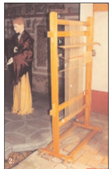
Fig. 7-8: Reconstruction of the warp-weighted loom (1) and the two-beam vertical loom (2) and their most important parts: a: upper beam, b: heddle rods, c: textile, d: shed-hole, e: warp, f: lower cross-beam, g: weights, h: lower beam
